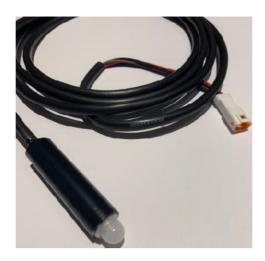
This cable is used to connect the (PIR) radar to the driver board. This cable, from one side end with the radar (PIR), keep in the appropriate support, to the other side instead, there is an IP68 connector. The length is 2 meters and can be fixed where you like. The suggestion is to fix it under the front bumper, near the center, between the fog lights for a better performance.
