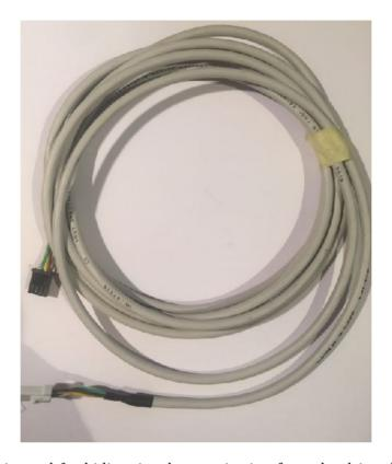
The DMX cable is used for bidirectional comunication from the driver board to the sound board. The sound board, which will be discussed later, is the one which interfaces with the ZA electronic set; this connection is done with a 6 rows<-> sound board cable; in case that the IP68 connector is used by swicthpod relay board, the sound board can be connected to a ZA relay board.
