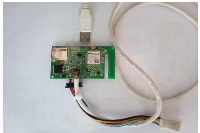
Fig 6 ; Meander Line Antenna Insulated With GSM Module
