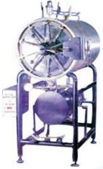
Inner chamber made of Stainless Steel (304 Grade), Outer Body Made of thick Mild Steel finished with Hammer Tone Paint/ S.S. Coated, Head made of Mild Steel- S.Steel lined. Pressure gauge. Provided with Radial locking system, safety device and with S.S. basket, water level indicator. Pressure up to 20 PSI, Complete with plug in Cord to work on 220 volts. A.C. Optional PID Control temp. controller.
