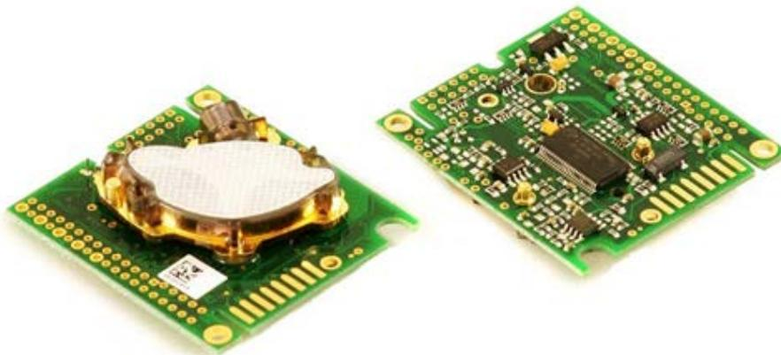
The K30 CO2 Sensor will be connected to the Arduino using wires and both devices will be attached to a small piece of plywood board which will neatly fit in the 4 inch diameter body tube. There will also be openings on the sides of the body tube where the sensor is so that the payload can measure the air quality in the atmosphere. The SD card will be connected to the Arduino and
