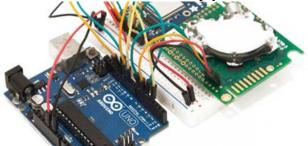
The Sensor has a response time of 2 seconds and a diffusion time of 20 seconds. Its measurement range is from 0 to 10,000 ppm and its repeatability is  $\pm$  20 ppm  $\pm$  1 % of measured value within specifications. To perform self-diagnostics, we will run a complete function check. A circuit board is needed to regulate the voltage of the battery, filter out noise, and organize the connection between the K30 CO2 Sensor to the Arduino.
