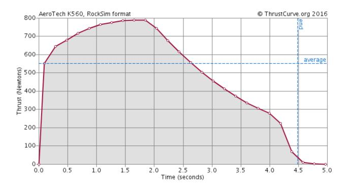
We would have preferred a motor with a higher initial impulse, or a spike, in the graph above, to increase the velocity of the rocket. Increasing the velocity of the rocket would have increased the normal force exerted by the center of pressure of our rocket and resulted in an overall straighter flight ("Calculating the Center of Pressure of the Model Rocket" by James Barrowman).
