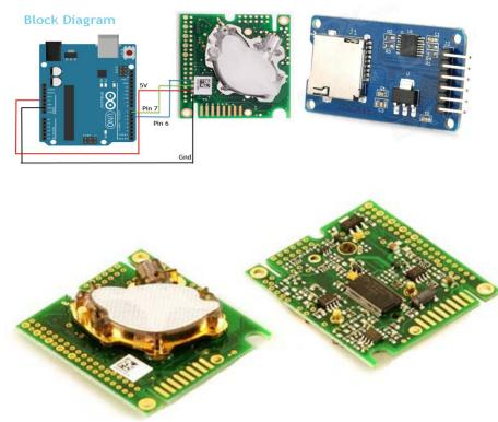
The K30 CO2 Sensor will be connected to the Arduino using wires and both devices will be attached to a small piece of plywood board which will neatly fit in the 4 inch diameter body tube. There will also be openings on the sides of the body tube where the sensor is so that the payload can measure the air quality in the atmosphere. The SD card will be connected to the Arduino and
