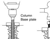
Drill holes using<sup>5</sup>/<sub>8</sub>" carbide tipped masonry drill bit per ANSI standard B94.12.1977.
