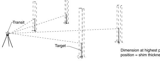
Dimension at highest position minus of position = shim thickness required
