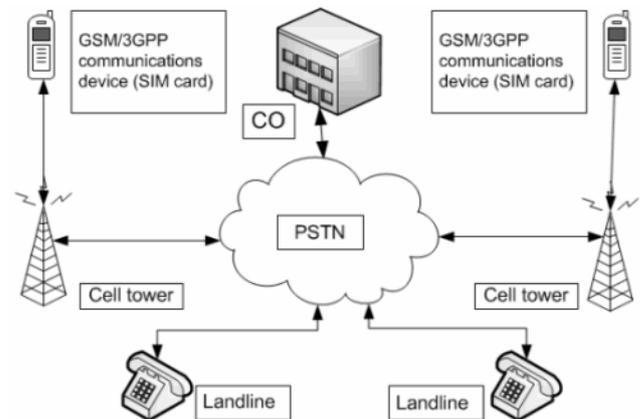
Fig.1 Architecture of Global Service for Mobile communications
