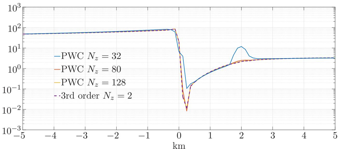
**Figure 1:** Apparent resistivity  $\rho_{xy}$  (at frequency  $10^{-3}$  Hz) along profile shown in Fig 2a. Solid (blue, red and yellow curves) are the results obtained with the use of piece-wise constant (PWC) IE solver. The colors distinguish between the results of modelings with different number of cells in vertical direction  $N_z$ . Dashed curve stands for the results obtained with the use of the presented high-order IE solver. See details in the text.
