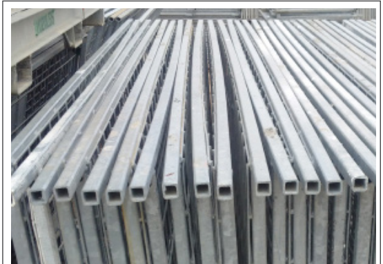
Maximum smooth deflection: ½" horizontal - panel acceptable
