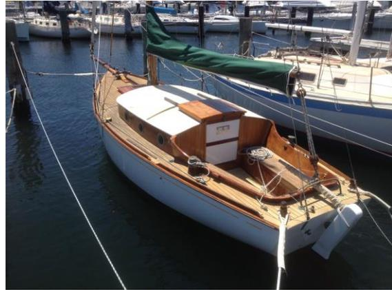
Her deck is marine ply on sheoak beams with laid teak overlay. The cabin is Jarrah and sheoak sides and beams with dynel sheathed plywood over sheoak tongue and groove roof. The cockpit has Jarrah coamings, plywood floor, plywood seats with laid teak overlay and sheoak tongue and groove sides
