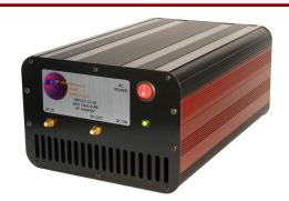
The RFPS27.12-50 is a Class AB 27.12MHz ISM amplifier mini-system, complete with power supply, heatsink, fan and thermal protection. It is excellent as a standalone driver for industrial, scientific, medical, or commercial applications. It utilizes a combination of three active device technologies for optimum performance and ruggedness.
