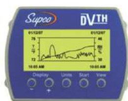
DVTH Temperatures, Humidity And Dew Point
