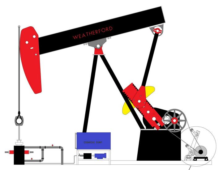
TITE-JAC™ is the system to use to ensure proper belt tension at all times. With high angular belt systems it is extremely hard to keep and maintain proper belt tension. TITE-JAC™ maintains proper belt tension at all times, even as belts stretch under load. TITE-JAC™ takes up the slack.
