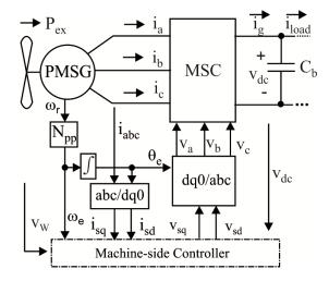
The concepts of the control have been developed in [5]and in the present paper new theoretical evidences that confirm the previous analysis were included. The block diagram for the control system is shown in Fig.5. The dc-link voltage control loop generates the required PMSG speed reference ( $_r^*$ ). The output of the dc-link
