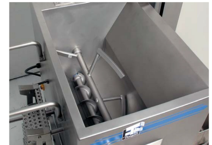
Model 6400 with programmed reciprocating paddle.
