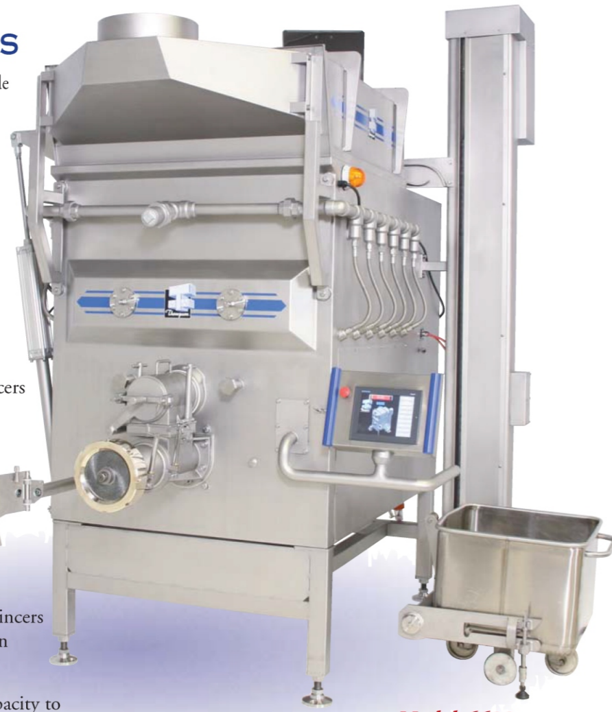
Model 6600 - 66 shown with 37 kW Variable Speed Control
