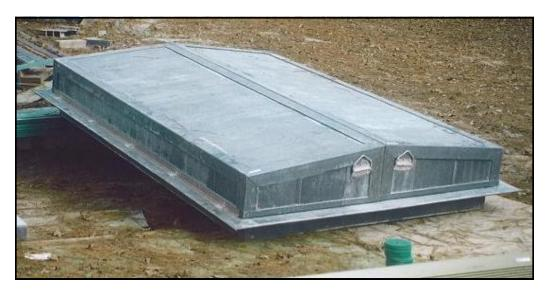
Above is a raised equipment drop-in access door assembly for Ontario, CA. This fabricated door assembly can be provided with sealed or non-sealed applications. Raised doors are used to protect equipment that protrudes above the concrete deck. Both halves are hinged for total access.
