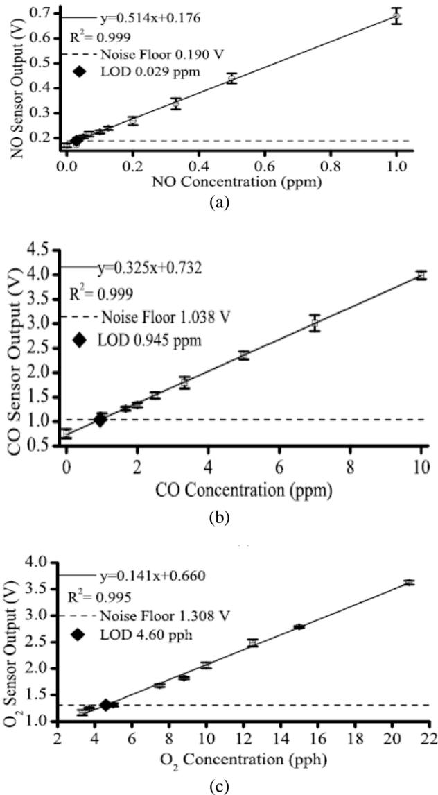
Fig 4: a) Calibration of Nitric oxide sensor. b) Calibration of Carbon monoxide sensor. c) Calibration of Oxygen sensor.
