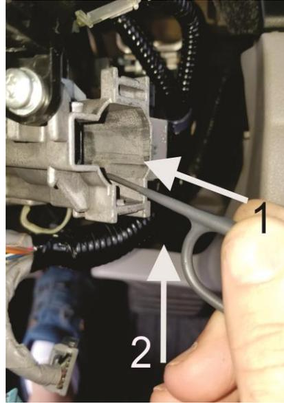
**Step 4** Once the tip of the tool slips off the bottom of the plunger, push inward on the tool to get a bite on the side of the plunger **Pic 3-1**. While holding medium inward pressure, raise the handle of the tool upward **Pic 3-2**. This will pull the spring-loaded plunger downward and at the same time the ramp of the tool will push the spindle back into place.
