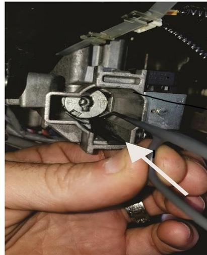
**Step 3** Slowly tilt the tool handle down, which raises the tip until the tip of the tool contacts the bottom of the spring loaded plunger **Pic 2-1**. Gently pull outward on the tool slightly (approx. 3/16<sup>th</sup> in) just until the tip of the tool slips off the bottom of the plunger **Pic 2-2**. (You should feel the tool handle drop slightly when the tip slips off the plunger)
