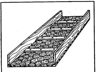
Building a Sluice Box: With a staple gun, attach to the plywood base a precut piece of indoor/outdoor carpet covered with a precut rectangle of fine chicken wire and four wooden crosspieces. Affix the base to the 3-m-long scrap-board sides.
