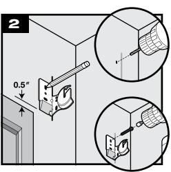
Mark bottom of slotted top hole on brackets. Drill 3/32" pilot hole on mark. If necessary, use wall anchor (not included). Secure brackets with one screw using a 1/4" driver.
