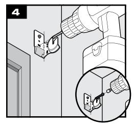
Drill second 3/32" pilot hole. If necessary, use wall anchor (not included). Secure brackets with second screw using a 1/4" driver.
