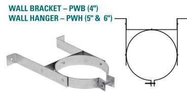
Used to provide lateral support while maintaining proper clearance. Recommended spacing is 6 ft. between bands above the starting point.
