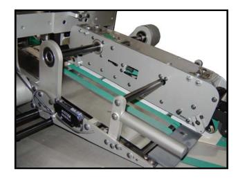
Speed matching between the feeder and base ensures accurate placement of a wide variety of stock from plastic cards up to 8.5" x 11" sheets.
