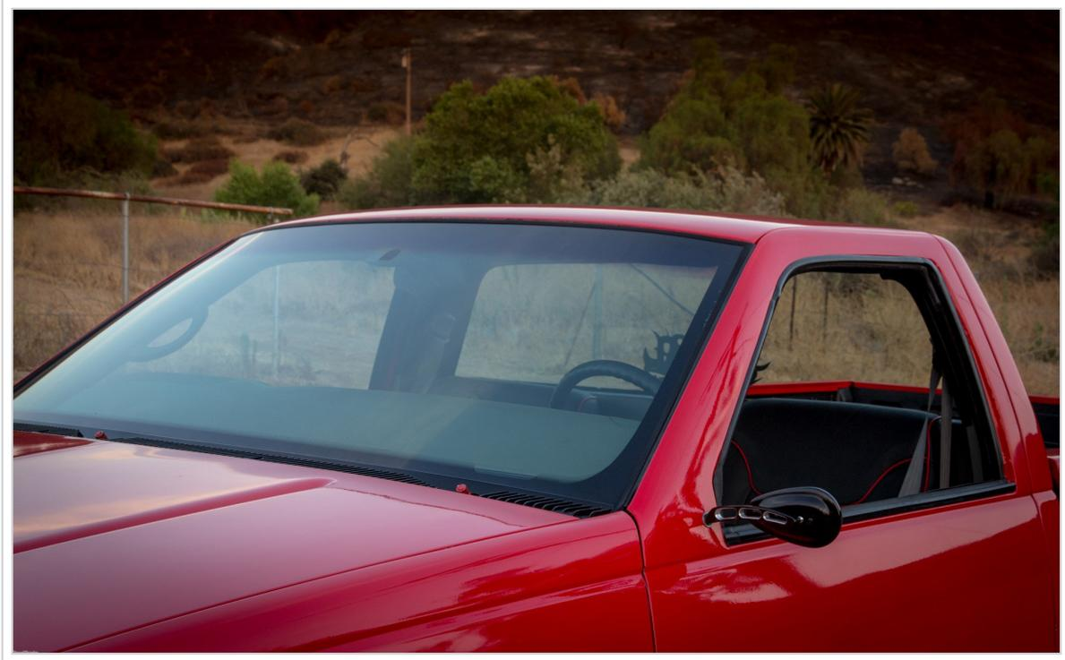
A 3-inch chop top performed by Bio Kustoms uses the stock glass and sets this C/K apart from the custom pack.
