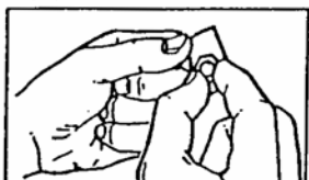
Step 3) For through holes, seal one end with tape.
