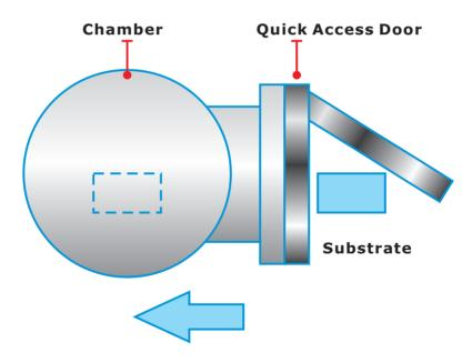
Substrate can transfer from atmosphere to vacuum chamber via quick access door
