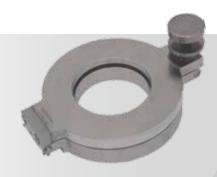
Fast Entry Doors provide convenient and fast manual loading of samples in and out of vacuum chambers. Doors are fitted with a spring-loaded hand knob locking mechanism, this patented design also prevent the Load Lock Chamber from being over-pressurized as the door will be pushed open.
