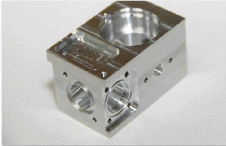
A finished sensor block machined on every side in two setups on a Doosan HP5100 heavy-duty HMC.
