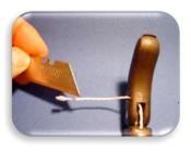
4. Adjust cable length to proper length and mark with marker
