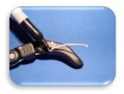
5. Tie new knot and apply super glue to back side of knot. Cut cord 1/8" past knot
