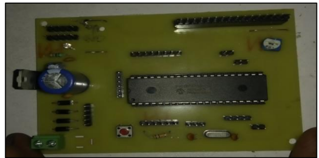
Fig.No.3 Power supply and control section
