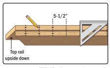
STEP #2 - Align top and bottom rails side by side with the top rail turned upside down as shown.
