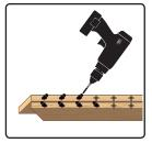
STEP #3 - Insert screw through connector and install where lines intersect for both top and bottom rails. Top and bottom baluster connectors will be facing opposite directions.
