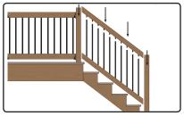
STEP #4 - With bottom rail mounted in place, insert all balusters into bottom rail. Start top rail at one end and insert connectors into balusters.
