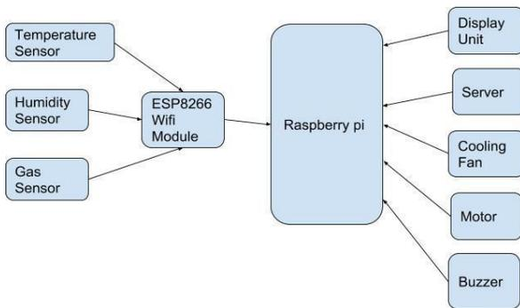
Fig. 1. Block diagram of WSN system
