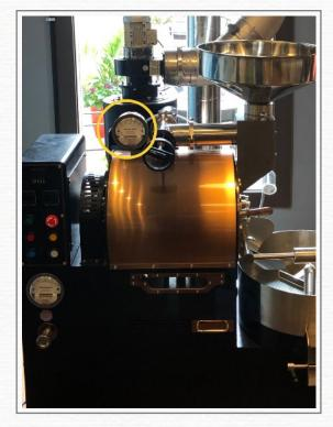
USING A MAG AIRFLOW GAUGE (SUCH AS THE ONE IN IMAGE ABOVE) WILL HELP YOU TO KEEP TRACK OF PROPER POSITIVE AIRFLOW THROUGH ROASTER AND EXHAUST
