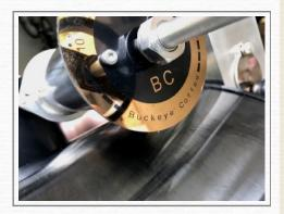
DAMPER HAS OPENINGS RANGING FROM 1-10. MOST ROASTING BEGINS WITH LOWER AIRFLOW (2-4 DURING DRYING PHASE) THEN INCREASES DURING BROWNING OR MAILLARD PHASE (4-6) AND MAY INCREASE MUCH HIGHER DURING ROASTING PHASE(6-9) DEPENDING ON
