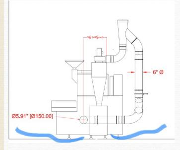
As seen in illustration of front view on the BC-1 thru 5 airflow into roaster<u>in part</u> comes through the bottom of unit and must not be covered or blocked in any way. There are also side vents near burner room.
