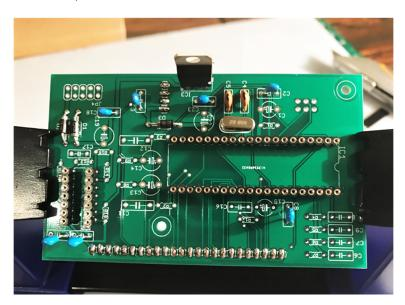
Install and solder the 2 x 100uf electrolytic capacitors (C1, C19) followed by the 10uf electrolytic capacitor (C15) and the 470uf electrolytic capacitor (C22).
