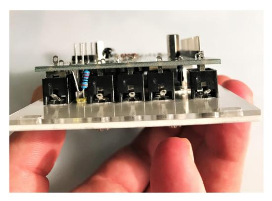
Lastly, push the LED to make sure it is inserted firmly into the hole on the front panel.
