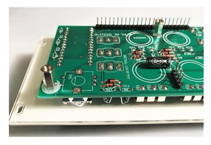
Inspect the soldering joints and look for shorts, bad joints and unsoldered joints.
