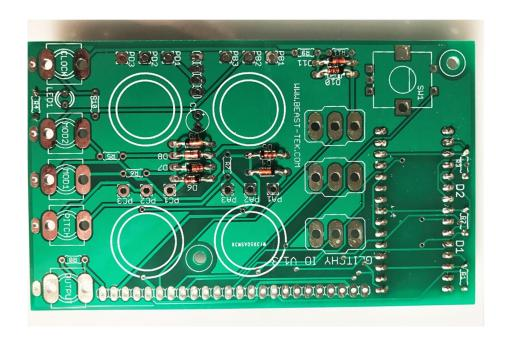
Install the 180 ohm resistors R1, R2, R3 and R4 on to the BACK of the PCB (no silk screen side). Install the 10K resistor R11 on to the BACK of the PCB (no silk screen side). Solder in place, trim leads.
