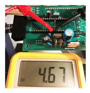
Connect the negative probe from a multimeter to pin 11 of IC1. Connect the positive probe to pin 9. The reading should be somewhere around 4.75v - 5.0v.
