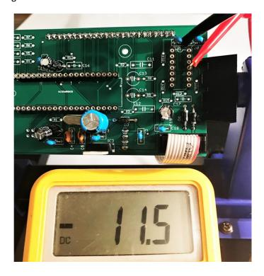
If these voltages do not check out, double check all solder joints and check the orientation of the voltage regulator (IC3) and the power diodes.
