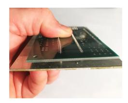
Tip: Solder only 2 pins of each socket at first to hold them into place. Now flip the board over to make sure the socket strips are sitting at right angles to the PCB. If required, they can be adjusted easily by heating the 2 joints one at a time and maneuvering the socket into place.
