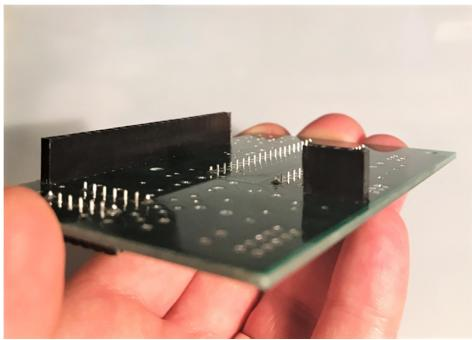
Once seated correctly, solder the remaining header strip pins.
