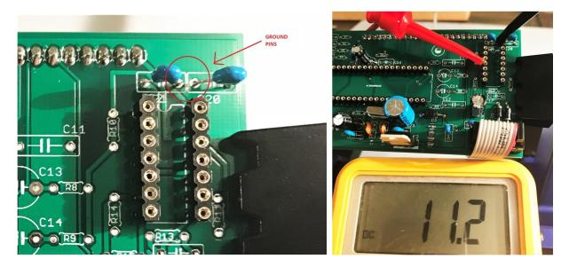
IC2 – connect the positive probe to pin 11 and connect the negative probe to one of the ground pins on C20 or C21 located directly above IC2.
