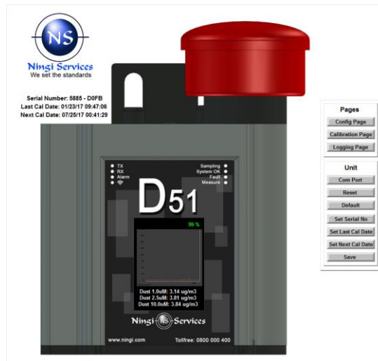
Figure 1 - D51 SCADA Screenshot
