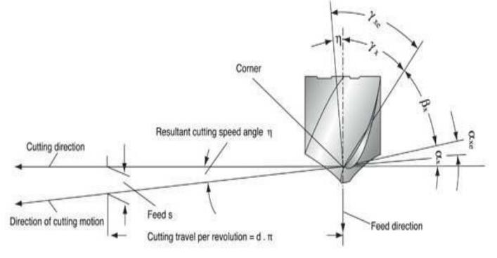
If the cutting lip is ground flat, it turns the drill into a scraping action which is great for wood/brass/plastic, but, it kills the self feeding characteristic and makes it nearly impossible to drill steel
