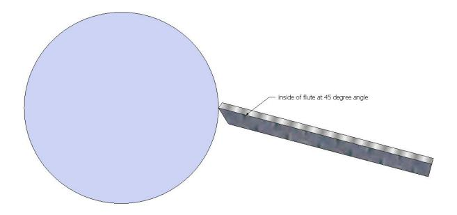
With the flute angled down, it will be a negative rake scraper and negative rakes don't want to cut. It will take more force to make this orientation cut.
