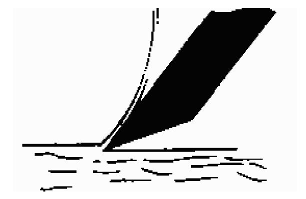
The common belief of the twist on a drill bit is for chip removal, which it does do, BUT the twist gives the cutting edge a positive angle which helps PULL the drill bit into the work piece
