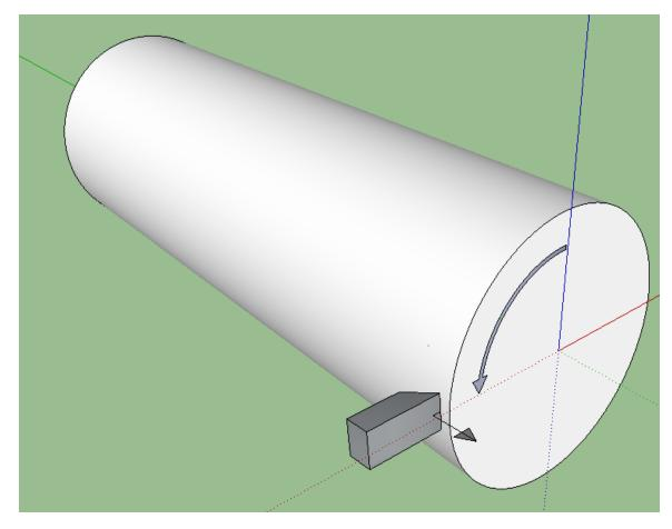
First, you have to consider the grain direction. You should always go WITH the grain, going against the grain causes tear out. Always cut <u>WITH</u> the grain, not against the grain direction. Cutting against the grain direction will pull the wood fibers up like petting a dog backwards.
