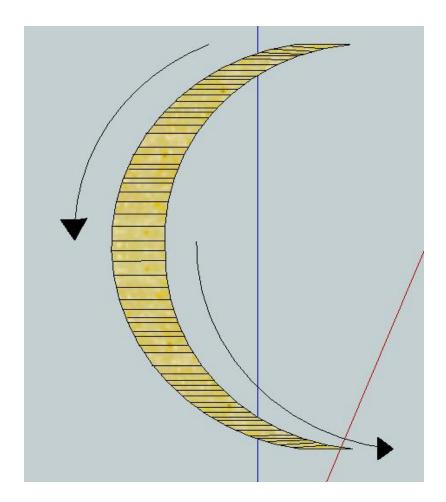
I use the gouge with the flute about half open to rough turn. It may be hard to see, but I am rubbing the bevel to control the depth of the cut. <u>Shear Cut.</u> <u>Notice the positive gouge angle!</u>
