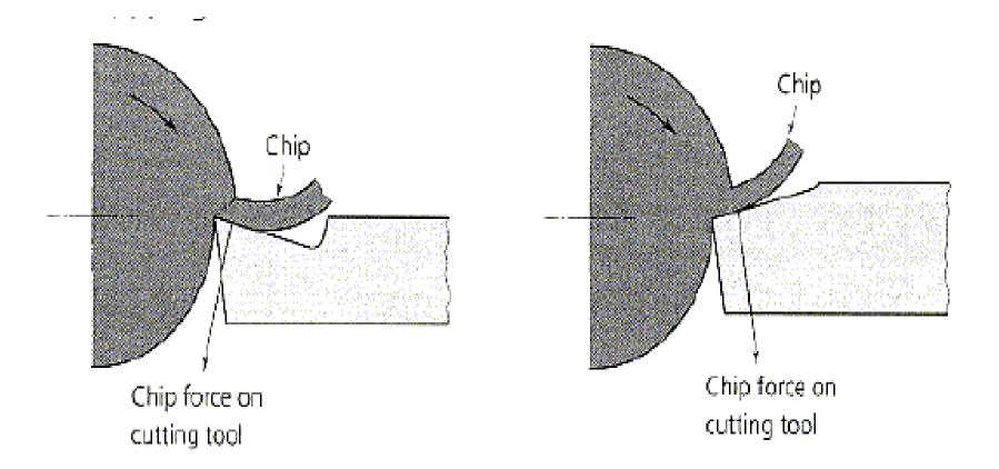
The negative rake tool actually pushes the wood fibers down and with that, the other wood fibers support the others so the fibers can be cleanly cut off. So what angle/twist angle do you hold the gouge when turning? Simply put, it is not a static angle, but it constantly changes throughout the cut!
