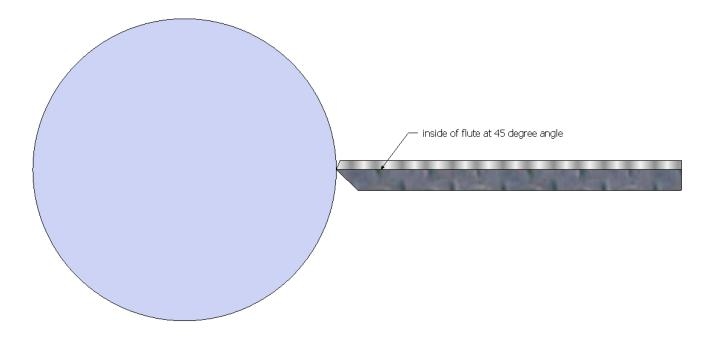
With the inside of the flute angled up (positive rake), the gouge will tend to self feed. If the angle is too great, it will cause the gouge to be "grabby" so then the angle should be reduced.
