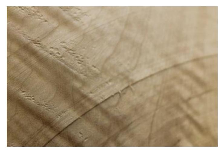
Slicing Cut: By closing the flute, the gouge will slice the side of the wood fibers with the nose radius instead of just shear cutting them. Notice that the cutting edge is almost parallel to the rotation of the wood.
