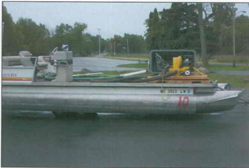
Figure 24. A suction dredging apparatus. © Superior Photique, 2009
