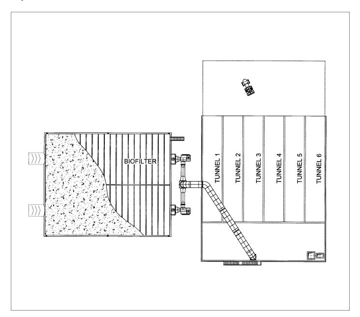
The plant uses biotunnel composting technology for the biological treatment of organic waste deriving from screened mixed municipal waste, as well as organic material deriving from source separation.
