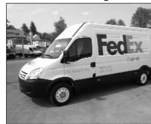
Results of FedEx's first six months of testing its ten Daily hybrid diesel-electric vans built by Italian truck maker Iveco have been completed. Over the first six months of the trial, which will continue until May 2010, each vehicle covered an average of 7900 km with a 26.5% reduction in fuel consumption and a total decrease in CO<sub>2</sub> emissions of 7.5 tons when compared with a fleet of traditional vehicles.
