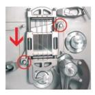
Extremely easy to insert, so that no time is lost for cleaning and refitting: "click&go" grid.
