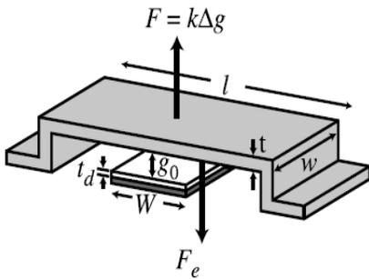
FIG. 2 Fixed beam structure
