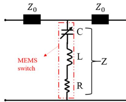
FIG. 3 Electrical Model of the RF MEMS Switch
