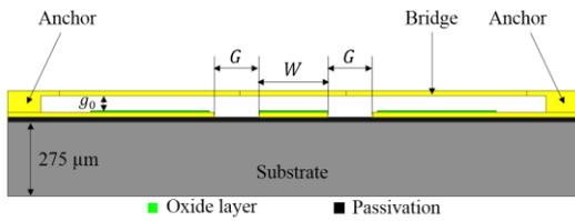
(a) Side view of proposed RF MEMS switch
