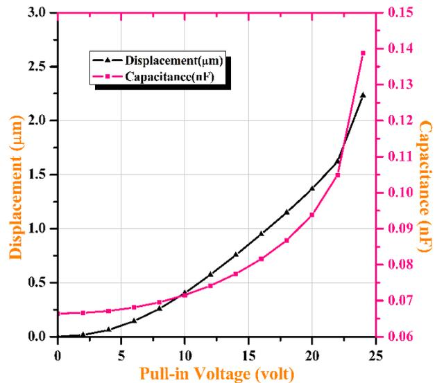
FIG. 4 RF MEMS Pull-in Voltage Vs Displacement and Capacitance
