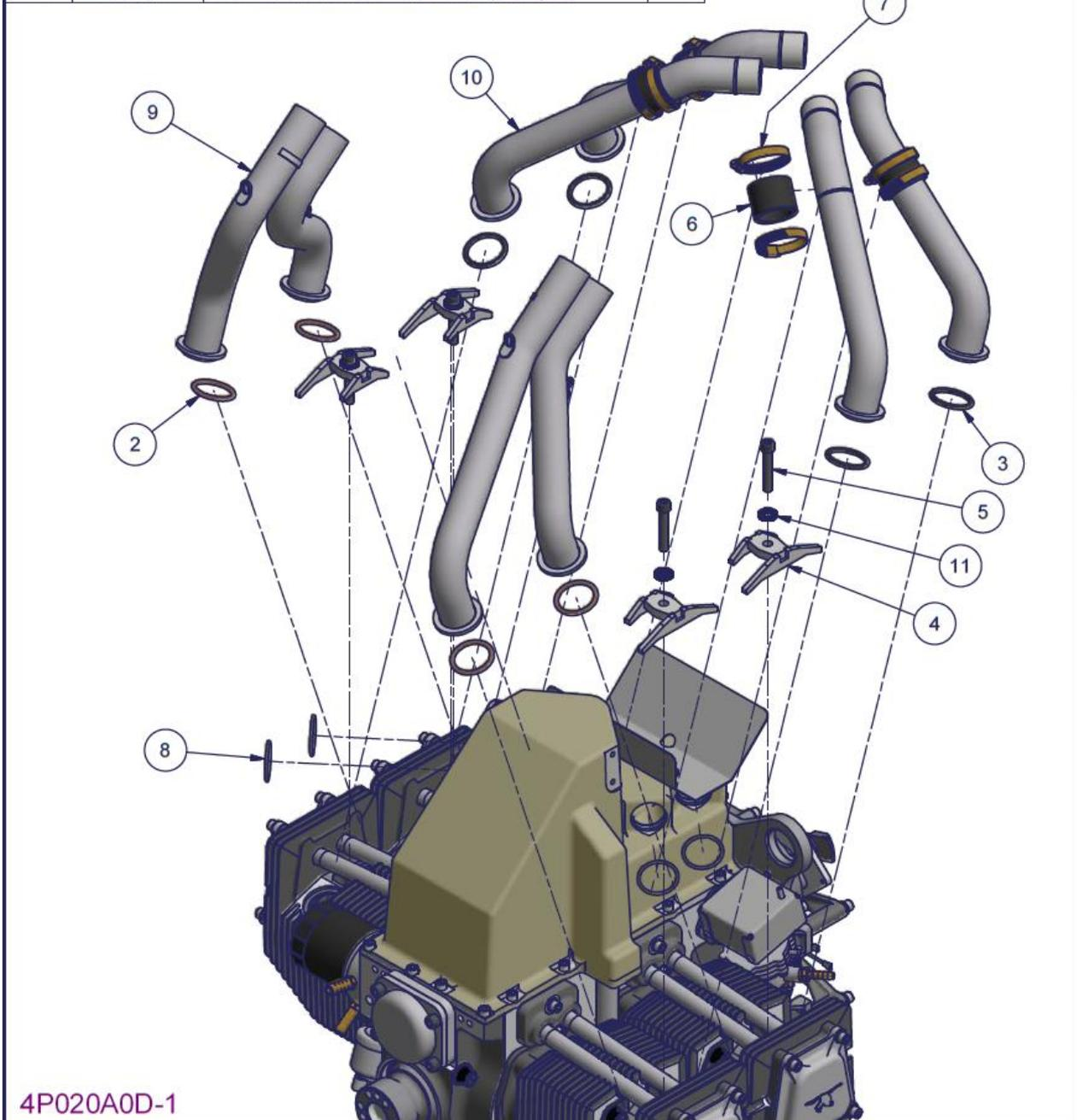
Figure 163 – 2200 Exhaust and induction pipe installation
