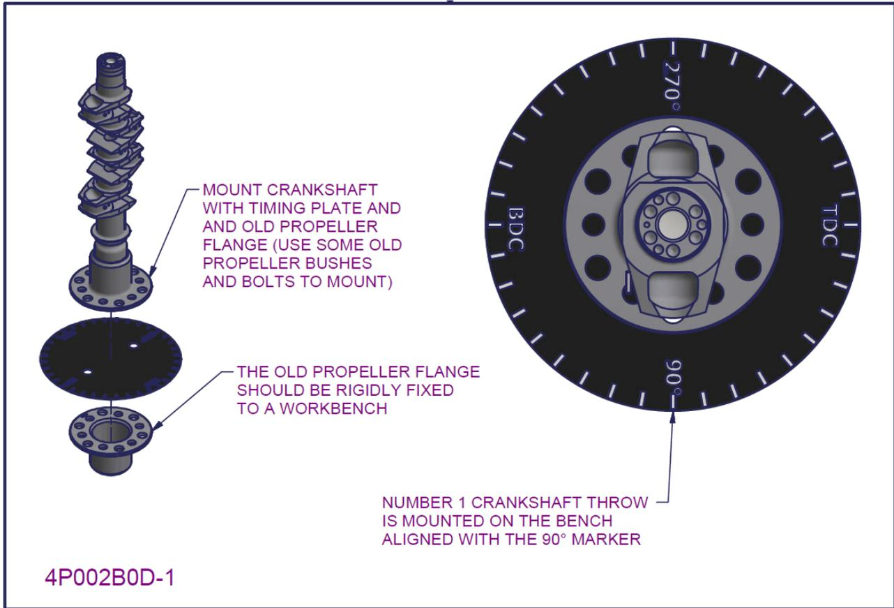
Figure 46 – 2200/3300 crankshaft subassembly 6
