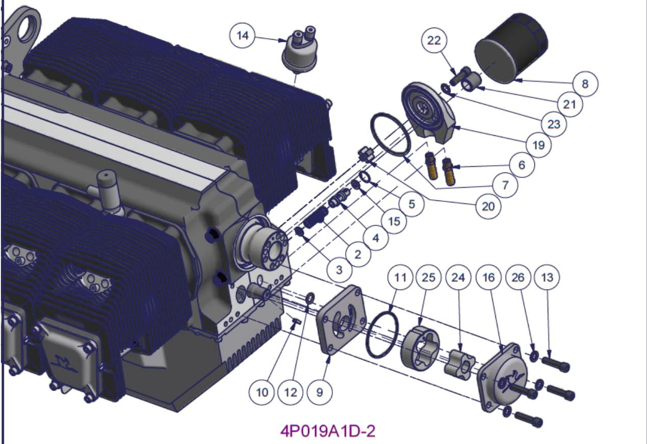
Figure 157 – 3300 Oil pump and filter installation (billet crankcase) – Parts List
