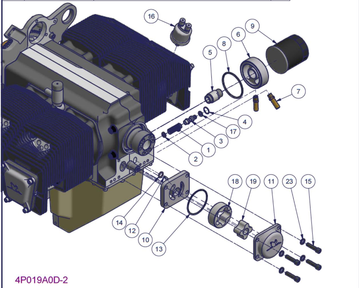
Figure 156 – 2200/3300 Oil pump and filter installation – Parts List
