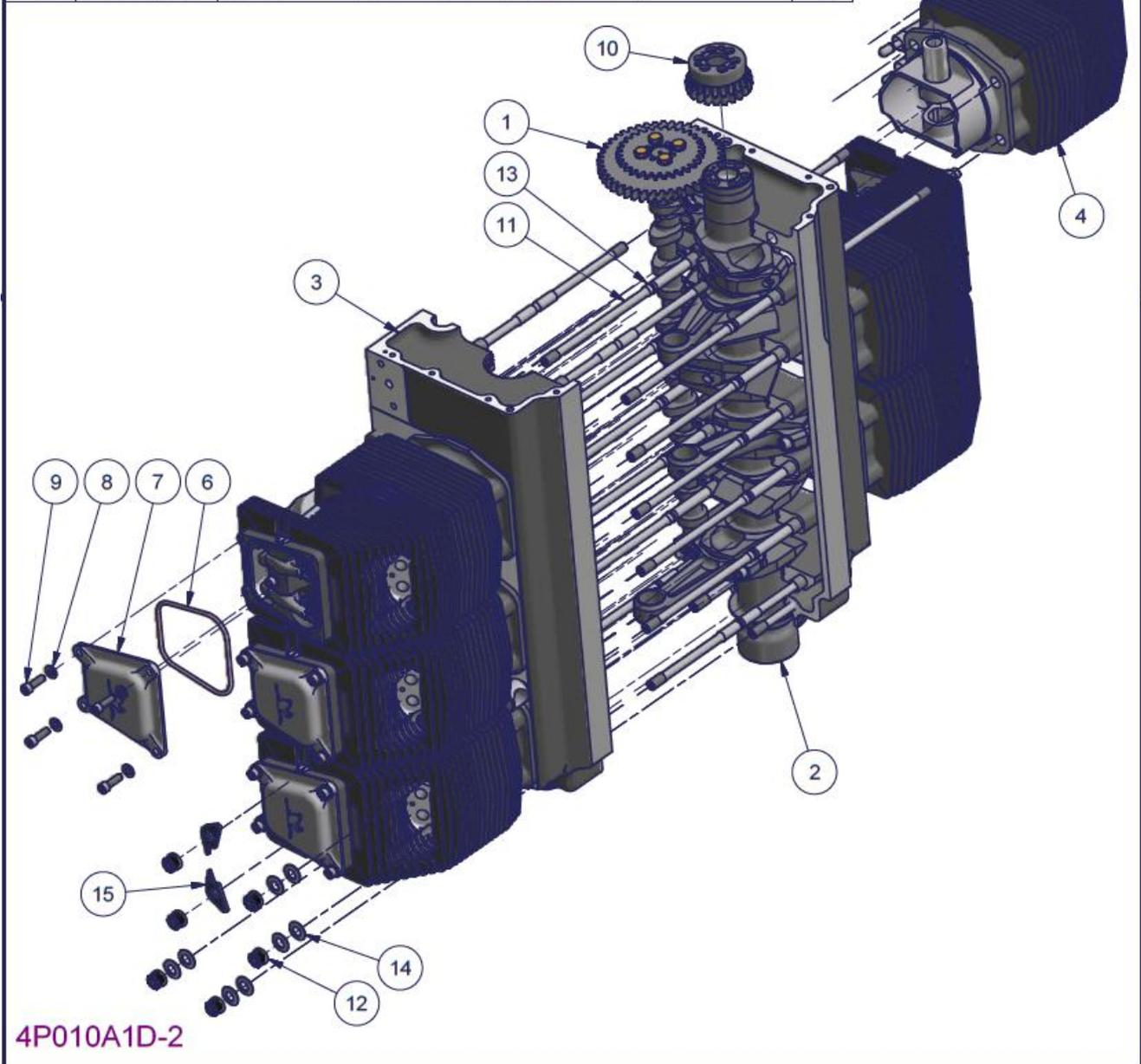
Figure 101 – 3300 joint engine – Parts List
