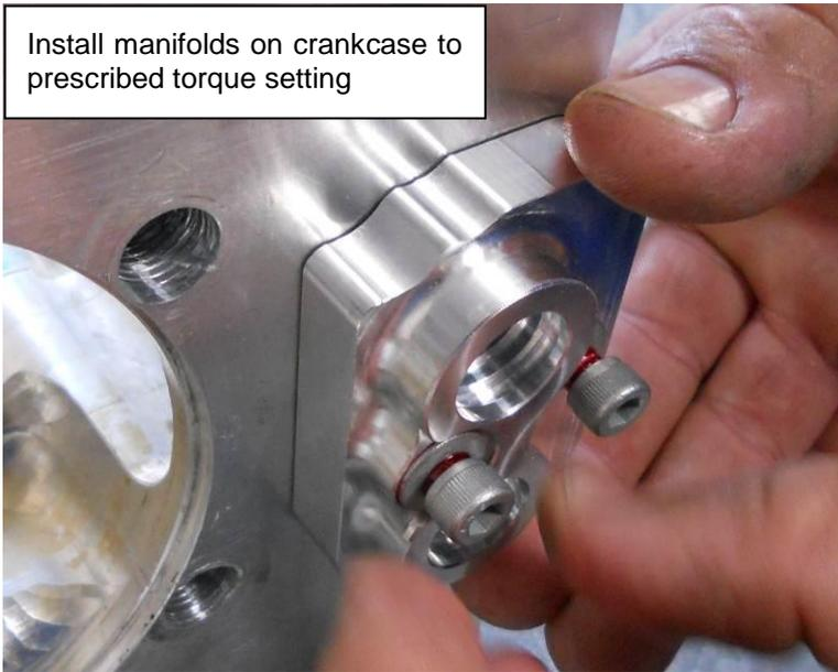
Install manifolds on crankcase to prescribed torque setting
