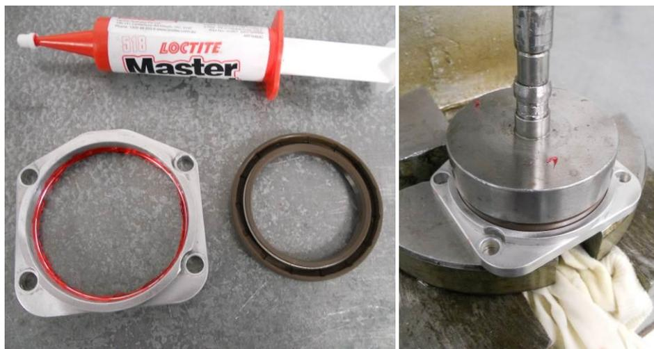
Figure 193 - External housing front seal installation
