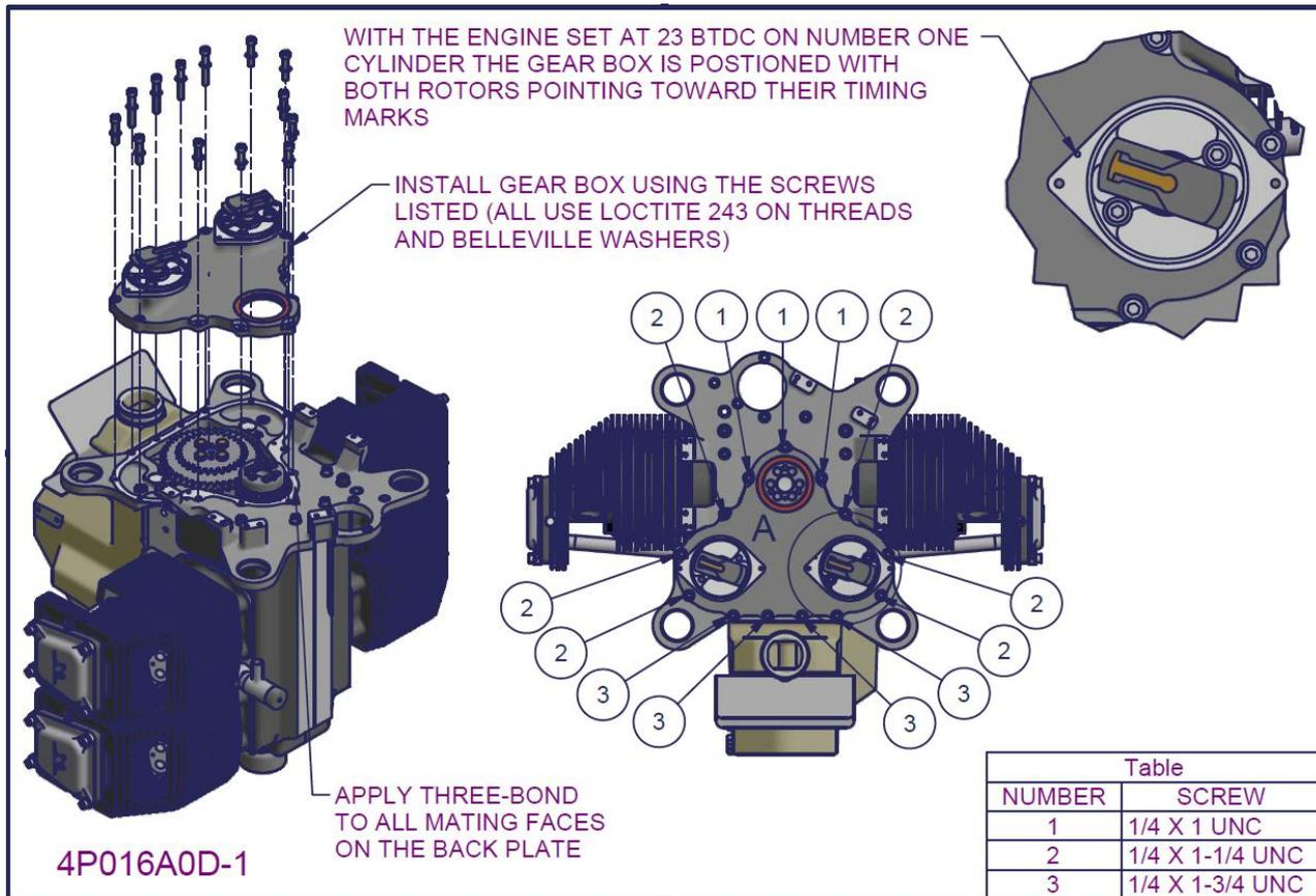
Figure 141 – 2200/3300 back plate and distributor gearbox installation 3
