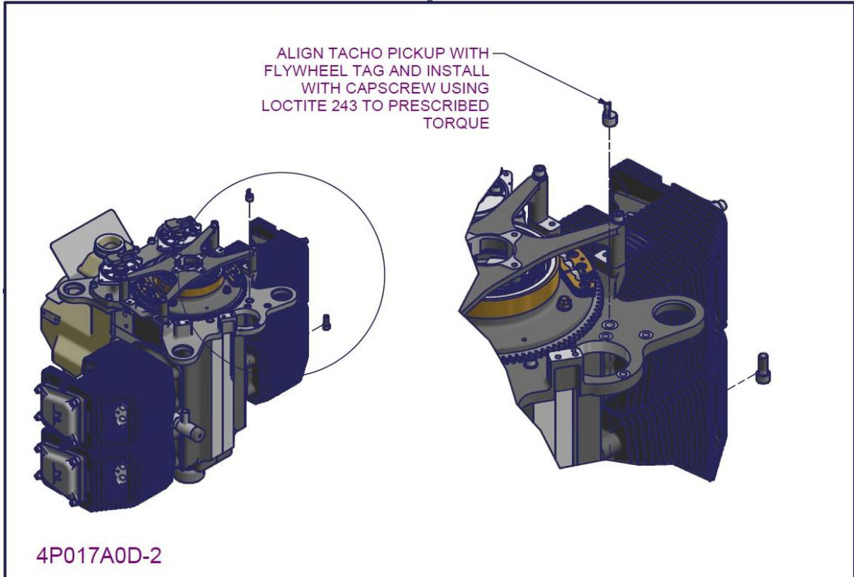
Figure 150 – 2200/3300 flywheel and alternator installation 3
