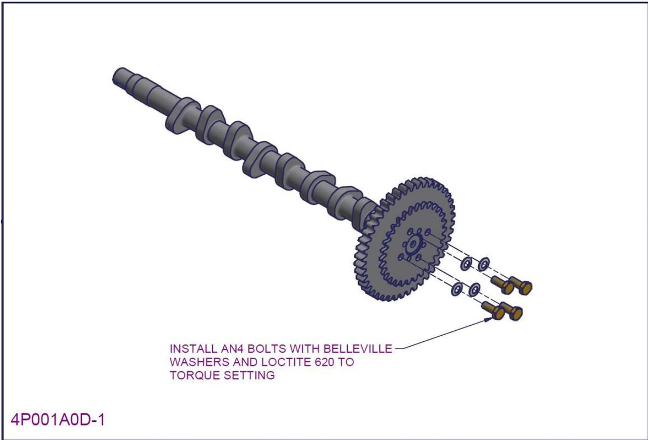
Figure 33 – 2200/3300 camshaft subassembly 2
