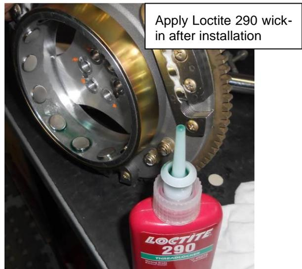
Figure 92 - Alternator magnet installation
