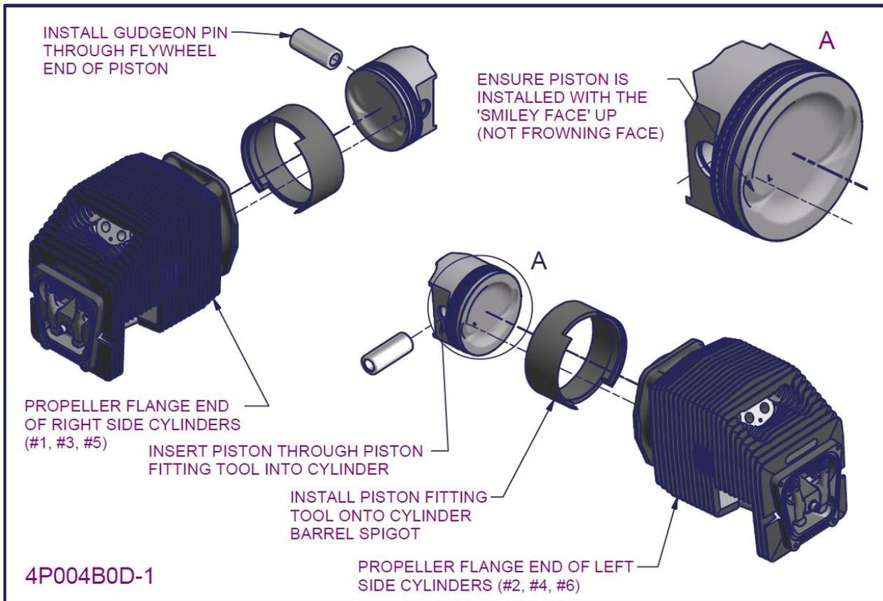
Figure 65 – 2200/3300 cylinder assembly 9
