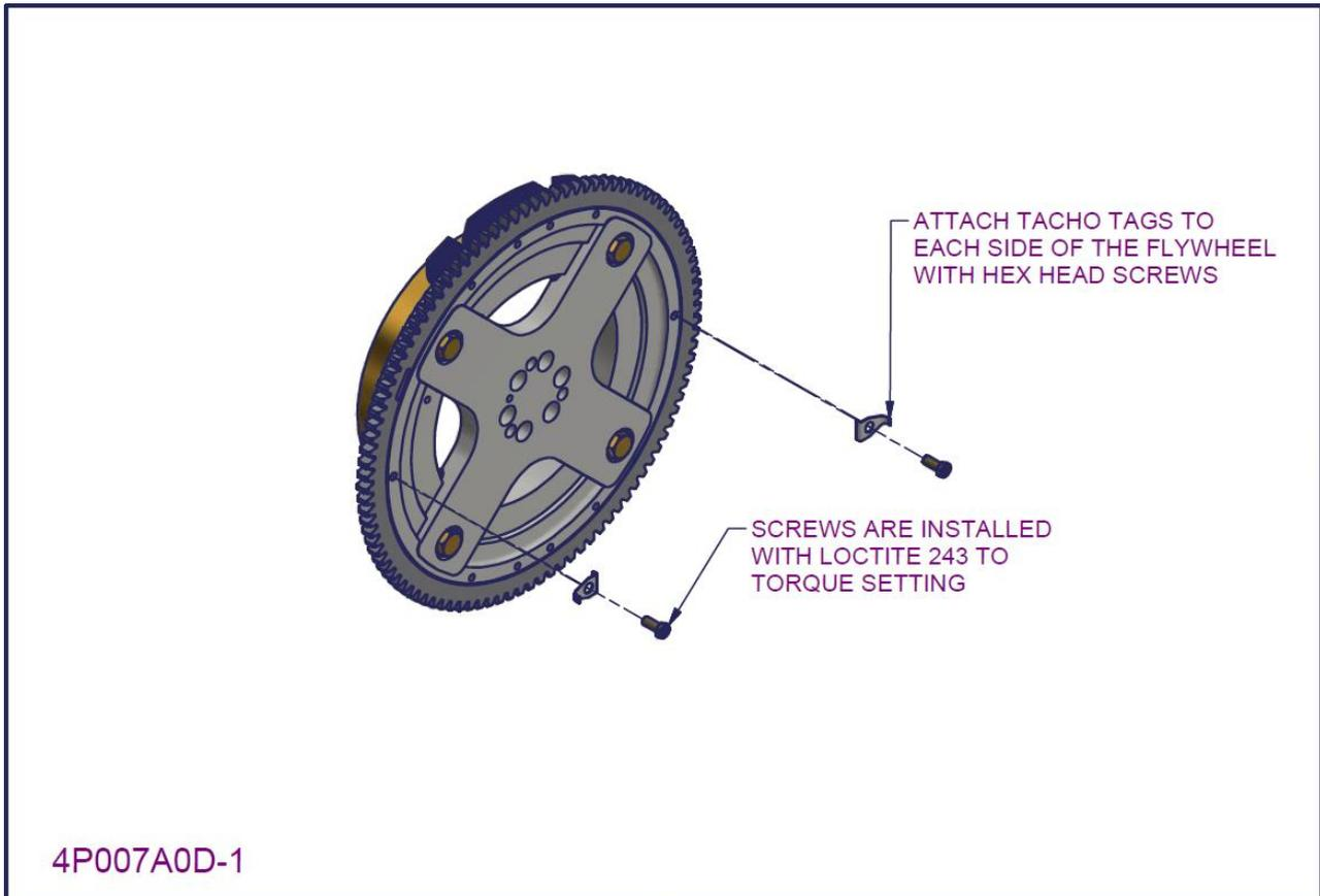
Figure 97 - 2200/3300 Flywheel subassembly (aluminium cross piece) 5
