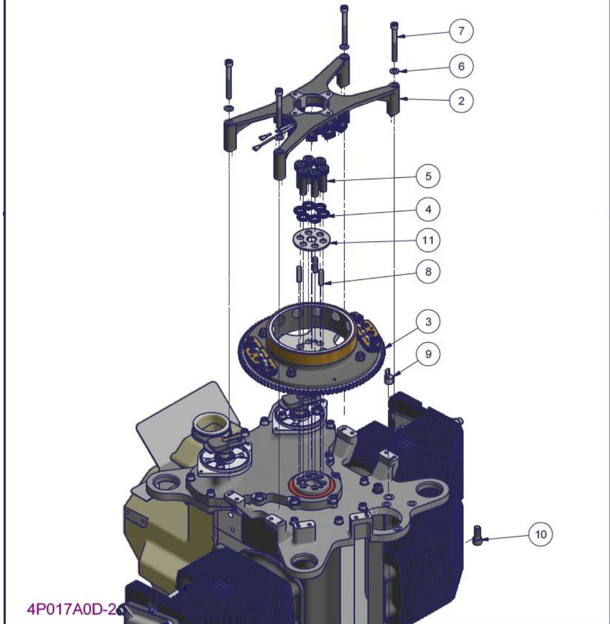
Figure 143 – 2200 flywheel and alternator installation – Parts List
