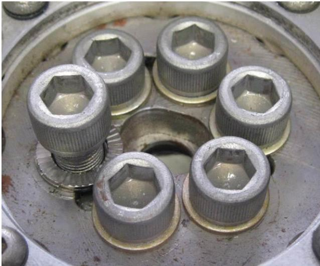
Reinstall capscrew with ONE Nordloc washer pair to **Prescribed Torque** (section 0) directly. Mark with Torque seal, or paint pen.
