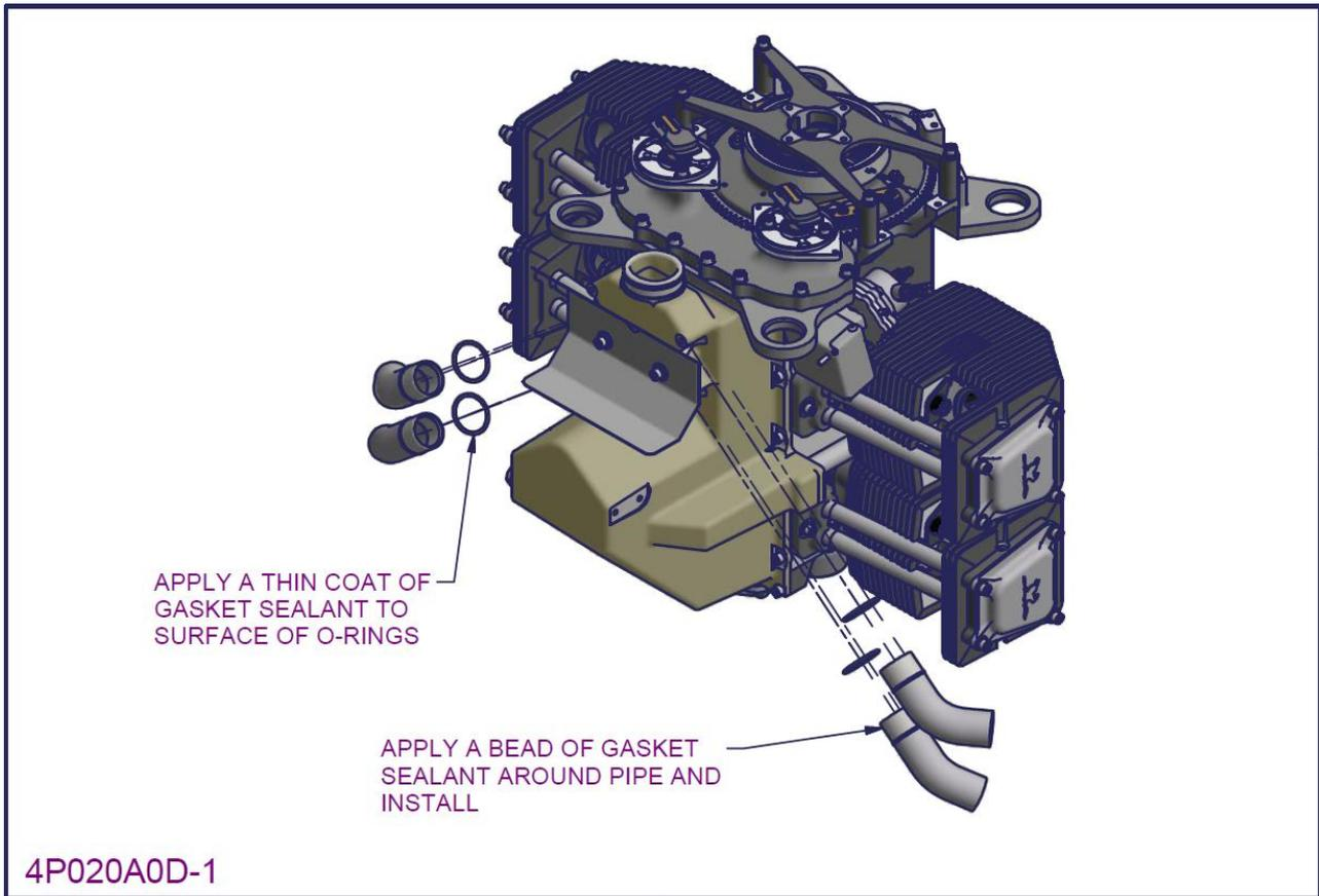
Figure 166 – 2200/3300 Exhaust and induction pipe installation 2
