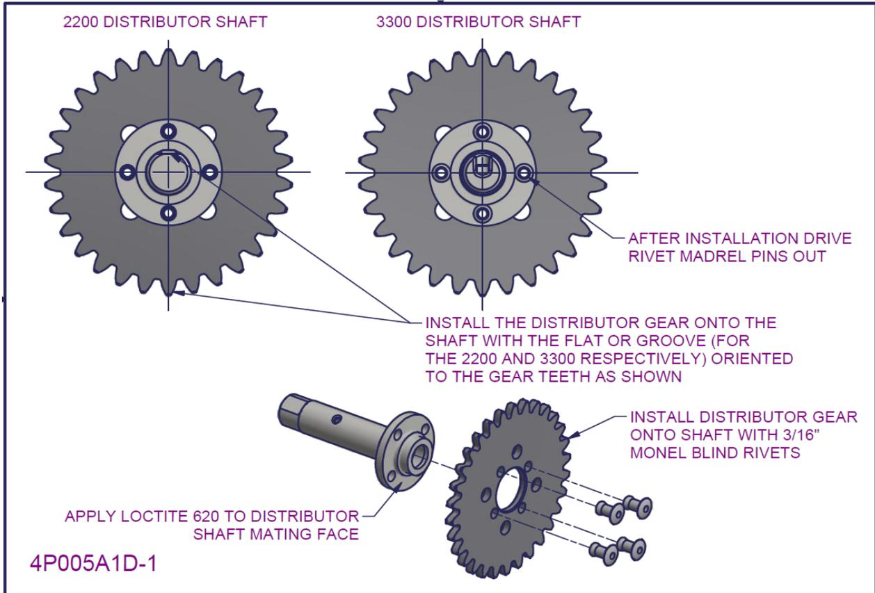
Figure 77 – 2200/3300 Distributor gearbox subassembly 4
