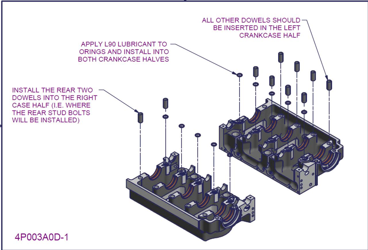
Figure 17 – 2200/330 crankcase subassembly 5
