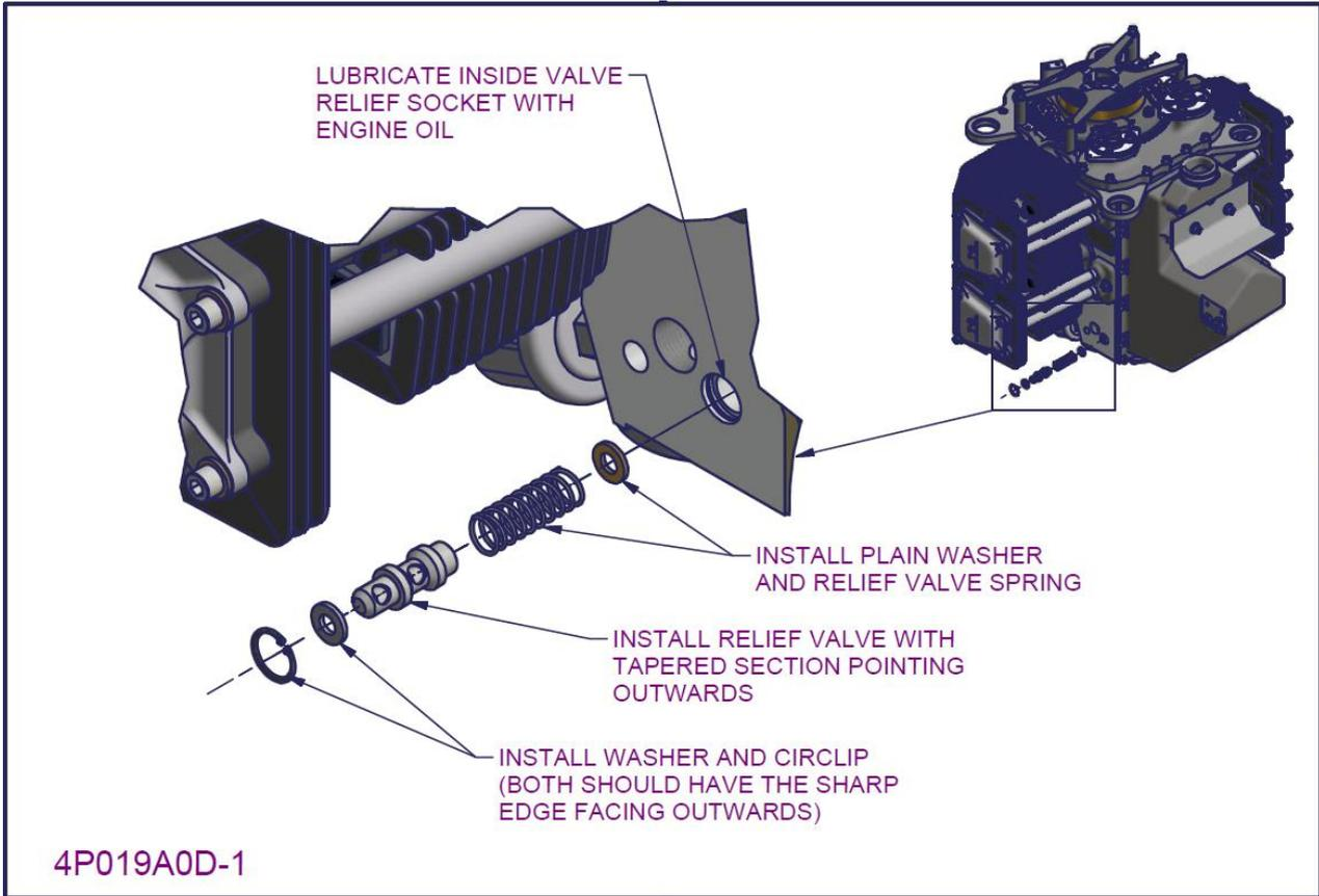
Figure 160 – 2200/3300 Oil pump and filter installation 2
