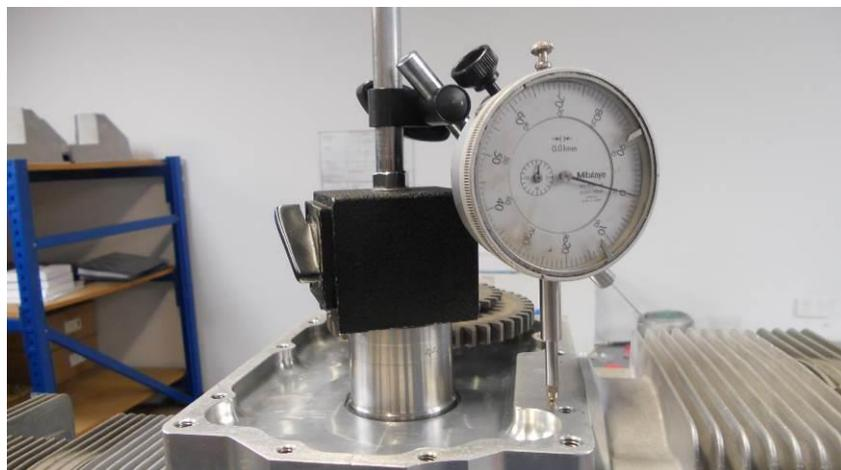
Figure 111 - Verifying end float using a dial gauge
