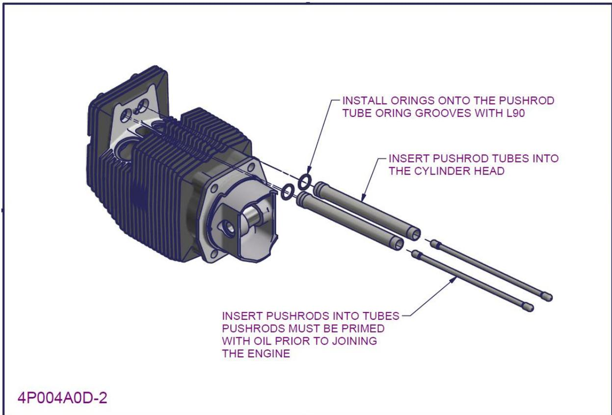
Figure 67 - 2200/3300 cylinder assembly 10a (external O-ring groove cylinder head)
