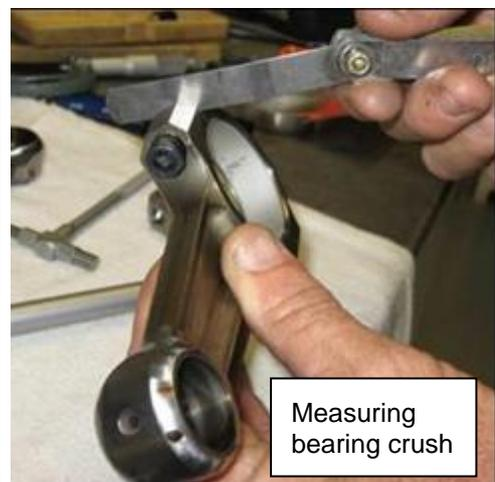
Figure 43 - Conrod measurements
