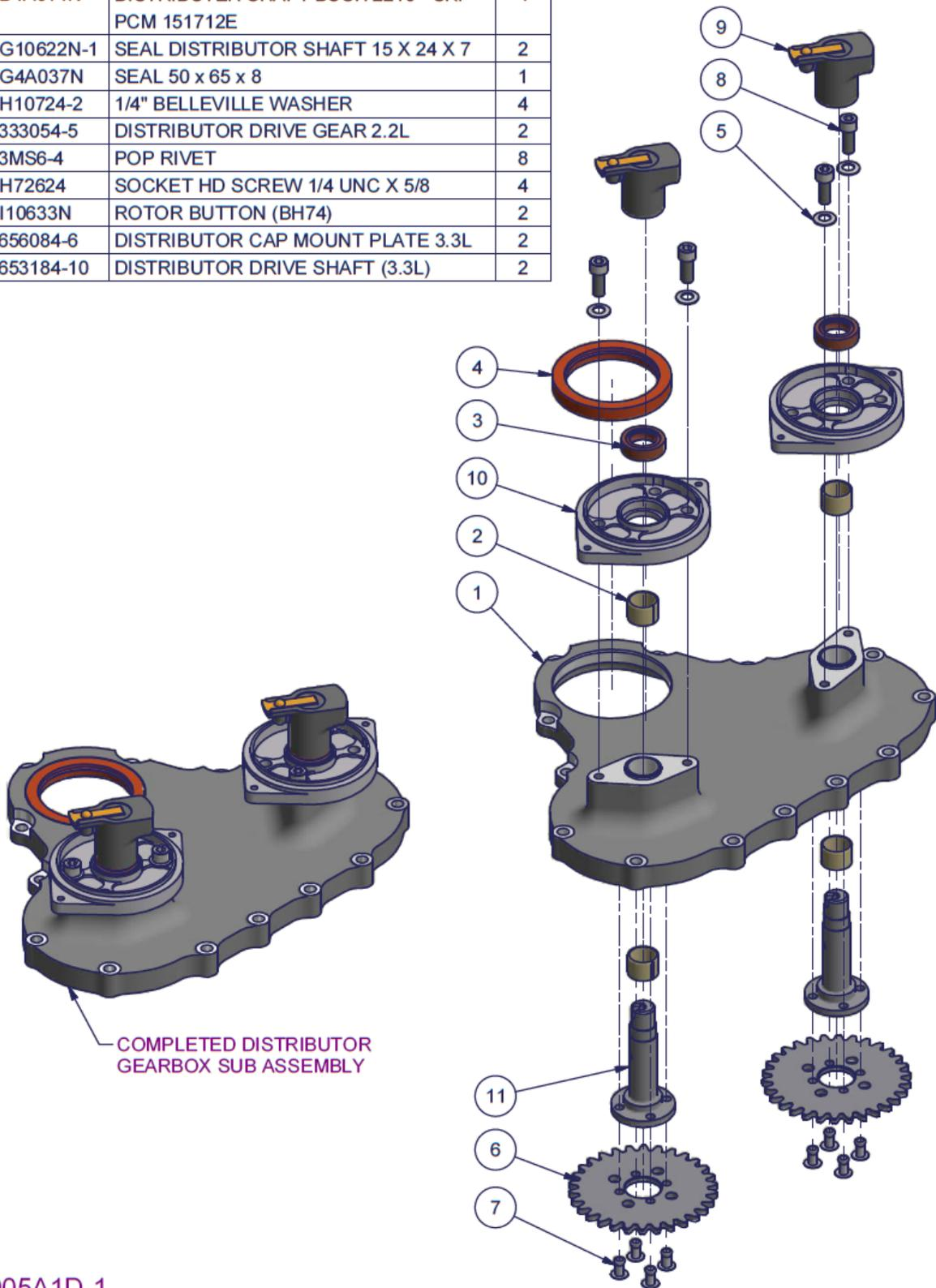
Figure 70 - 3300 Distributor gearbox subassembly - Parts list
