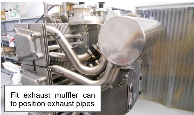
Fit exhaust muffer can to position exhaust pipes
