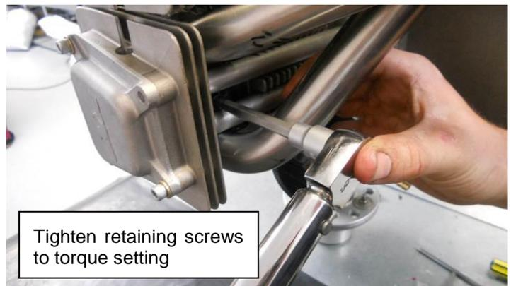
Tighten retaining screws to torque setting
