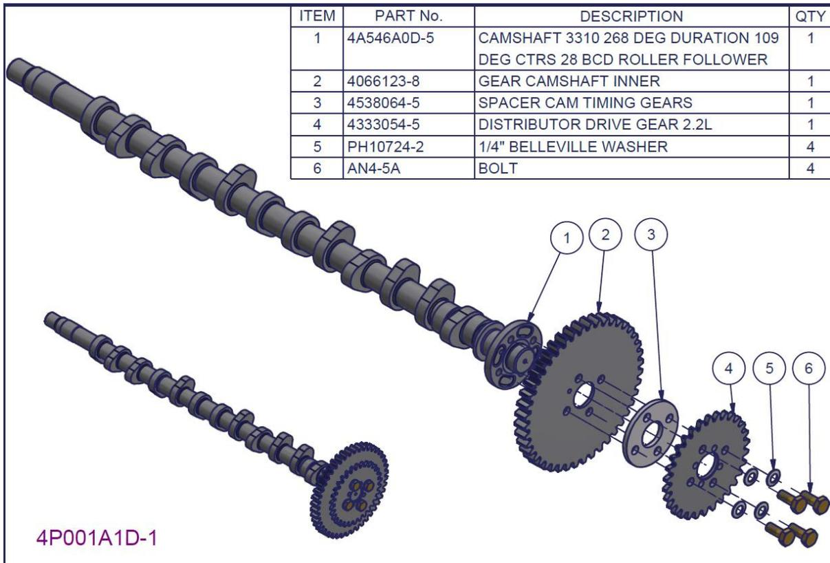
Figure 30 – 3300 Camshaft subassembly – Parts List
