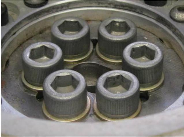
Install capscrews with 6 plain washers to **15ft.lb** and then the **Prescribed Torque** (section 0) progressively using diagonal pattern shown in Figure 145
