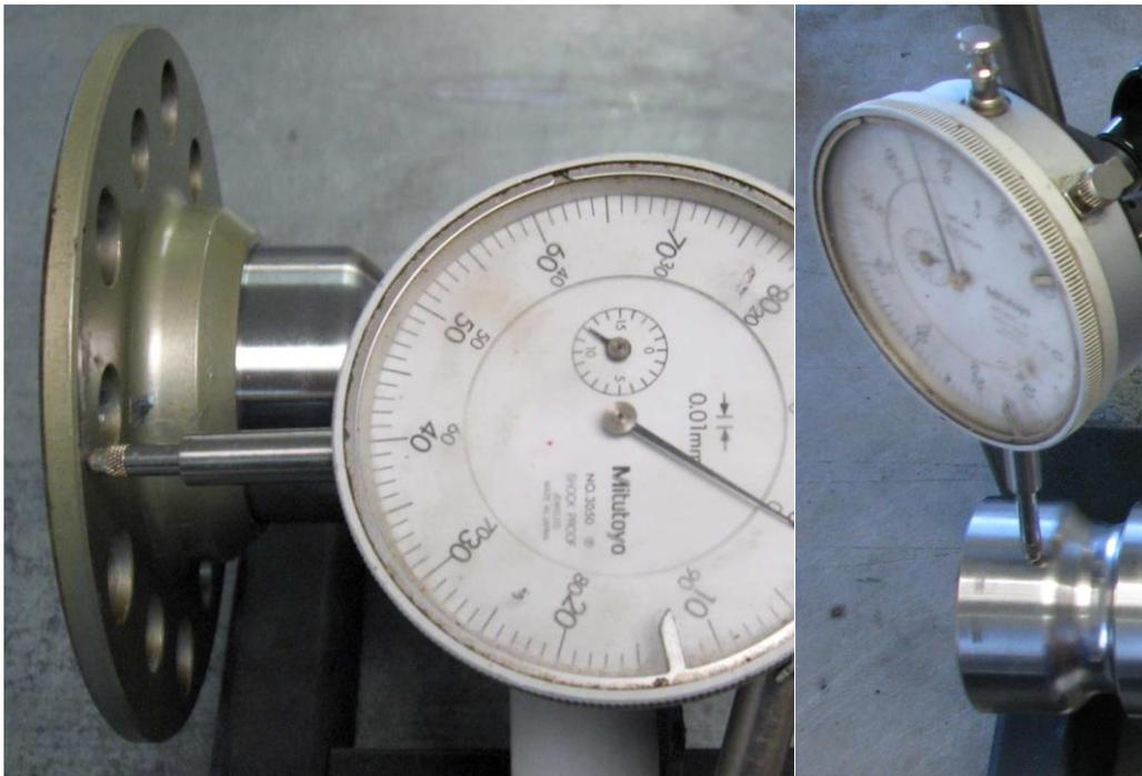
Figure 3 – Dial Indicator Position for Crankshaft & Prop Flange Run Out
