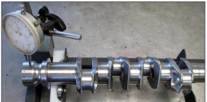
Figure 38 - Measuring propeller flange and crankshaft runout
