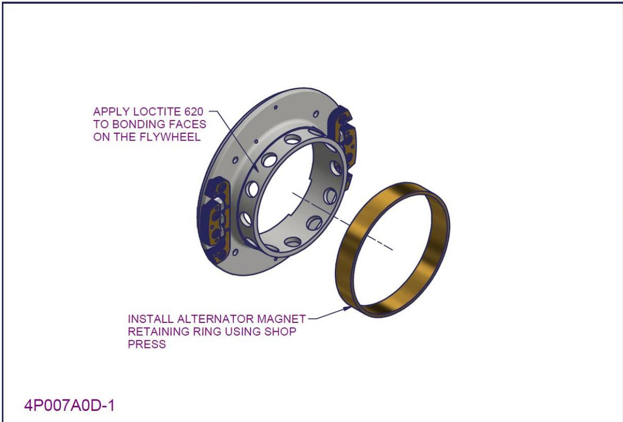
Figure 87 - 2200/3300 Flywheel subassembly (aluminium cross piece) 2
