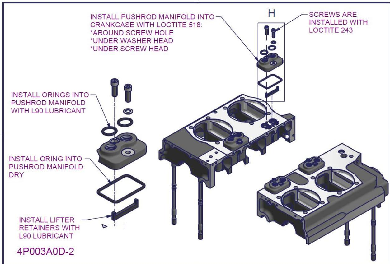
Figure 24 – 2200/330 crankcase subassembly 9
