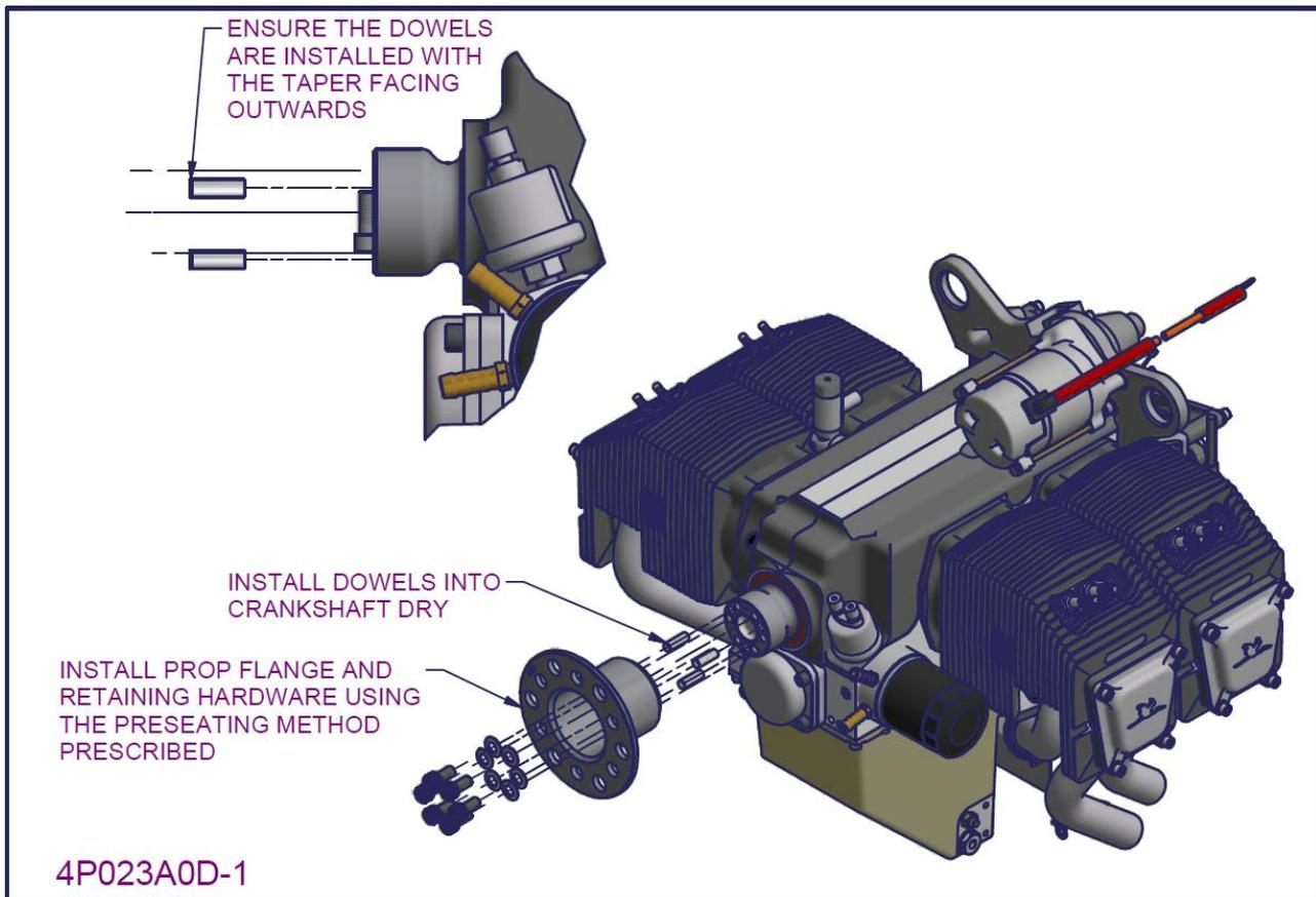
Figure 190 – 2200/3300 Front seal and propeller flange installation 3
