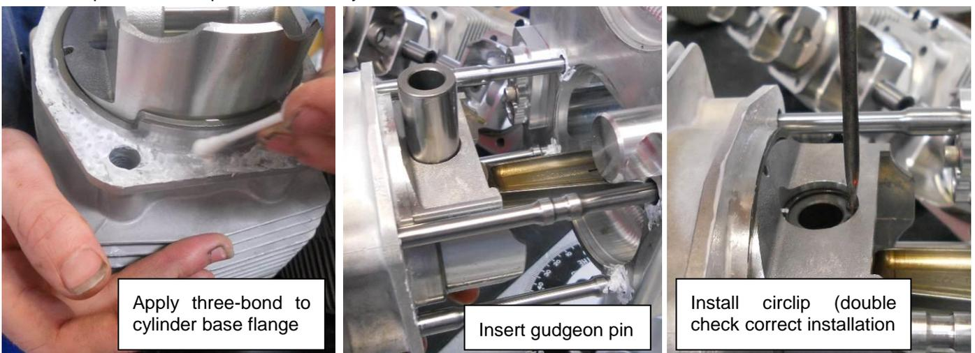
Figure 107 - Cylinder installation
