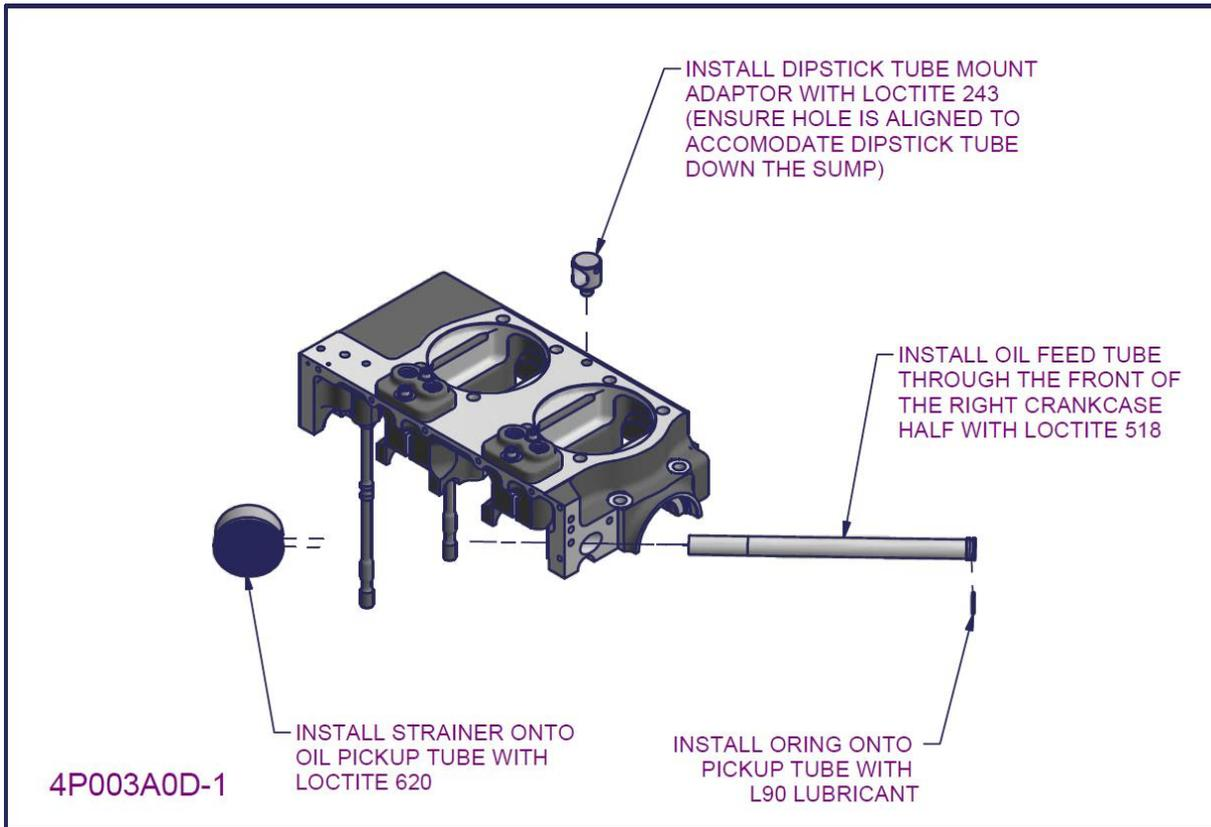
Figure 26 – 2200/330 crankcase subassembly 10
