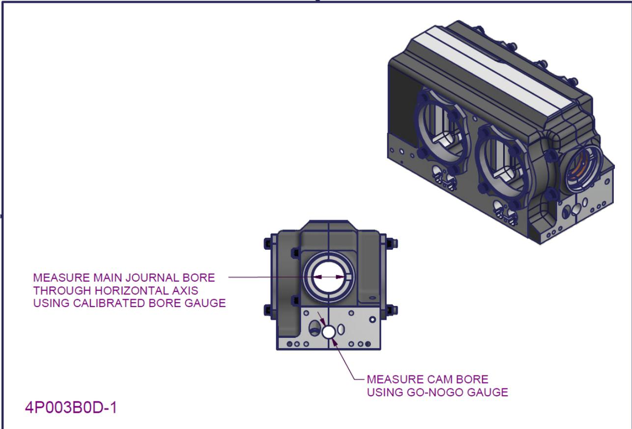
Figure 15 – 2200/330 crankcase subassembly 4
