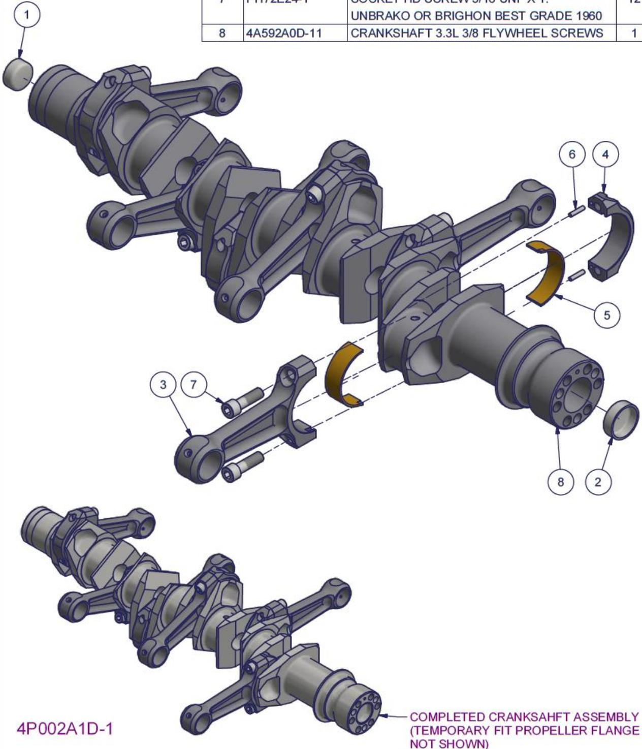
Figure 35 – 3300 Crankshaft subassembly – Parts List
