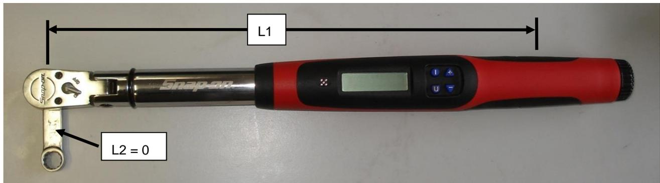
Figure 7 – Torque Wrench & Crows foot Adaptor Setting 2
