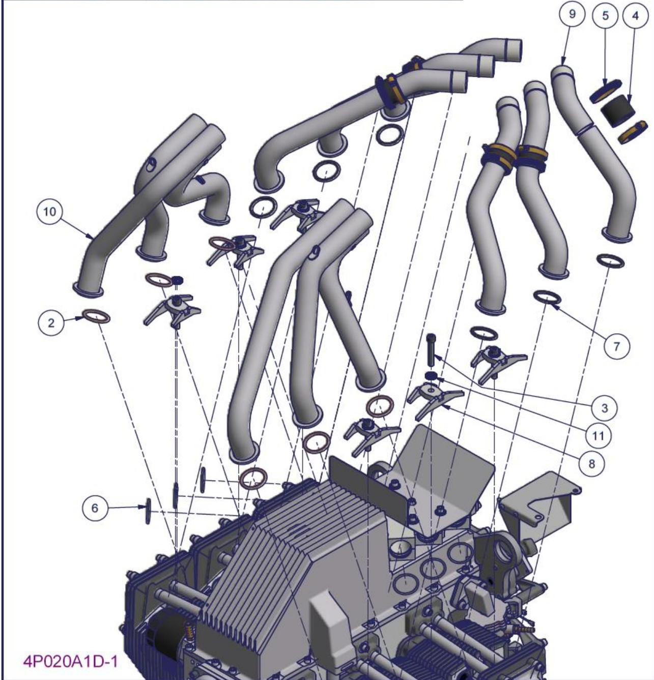
Figure 164 – 3300 Exhaust and induction pipe installation
