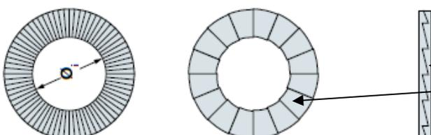
The Nordloc washer halves are assembled together with the broad wedges facing into each other
