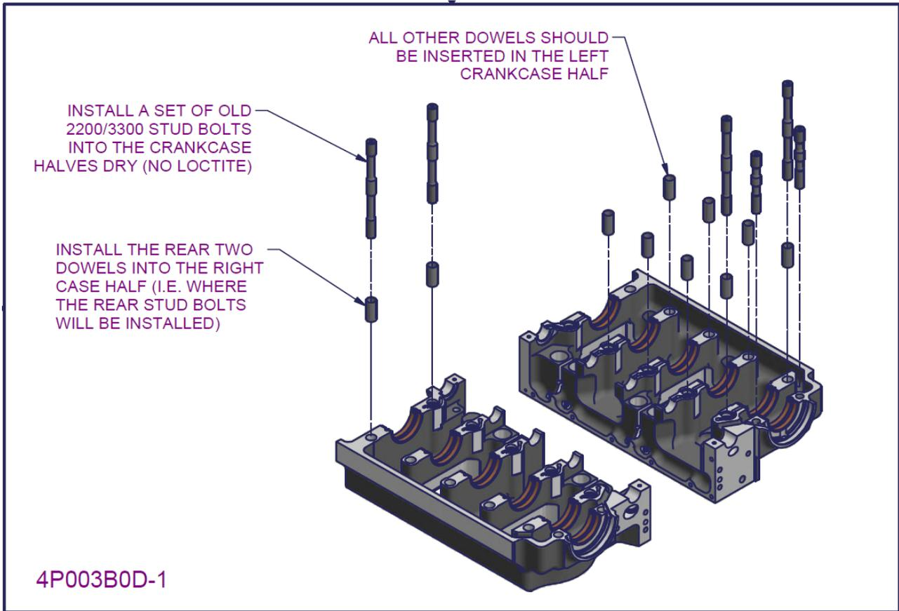
Figure 12 – 2200/330 crankcase subassembly 2
