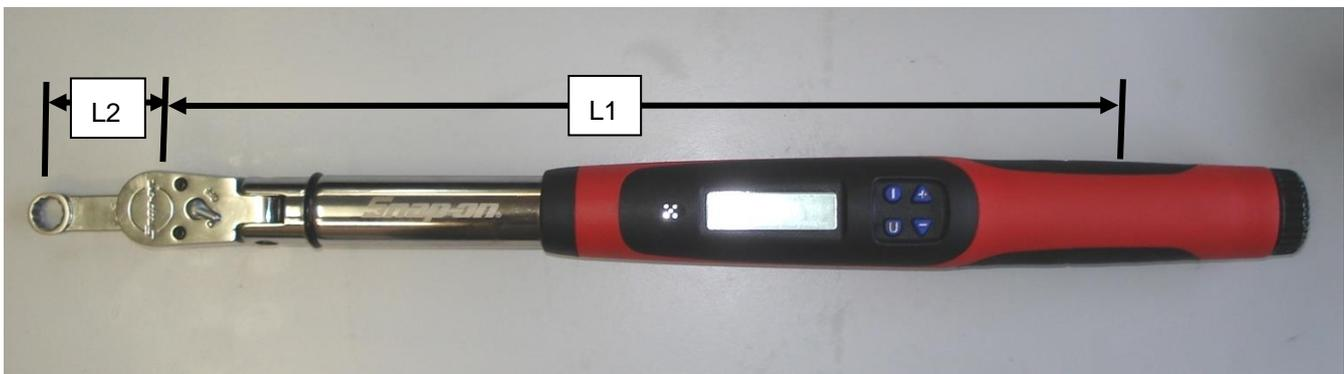
Figure 6 – Torque Wrench & Crows foot Adaptor Setting 1
