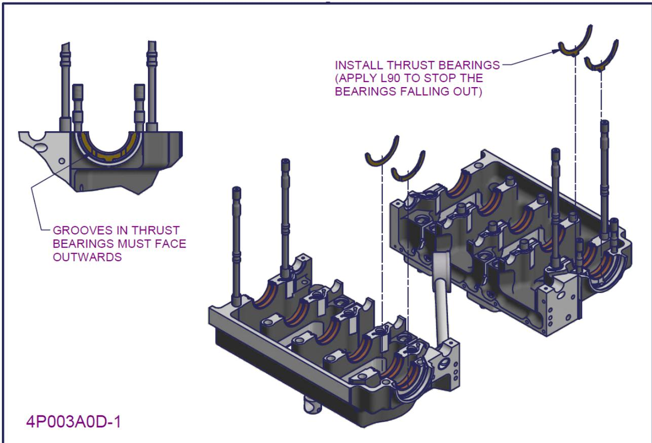
Figure 28 – 2200/330 crankcase subassembly 11
