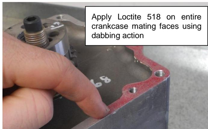
Figure 140 - Applying three-bond to crankcase faces
