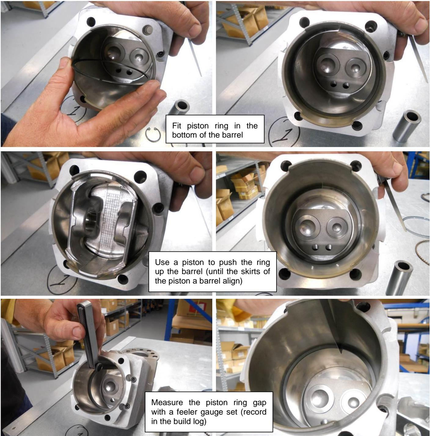
**Figure 61 - Piston ring installation and measurement**
