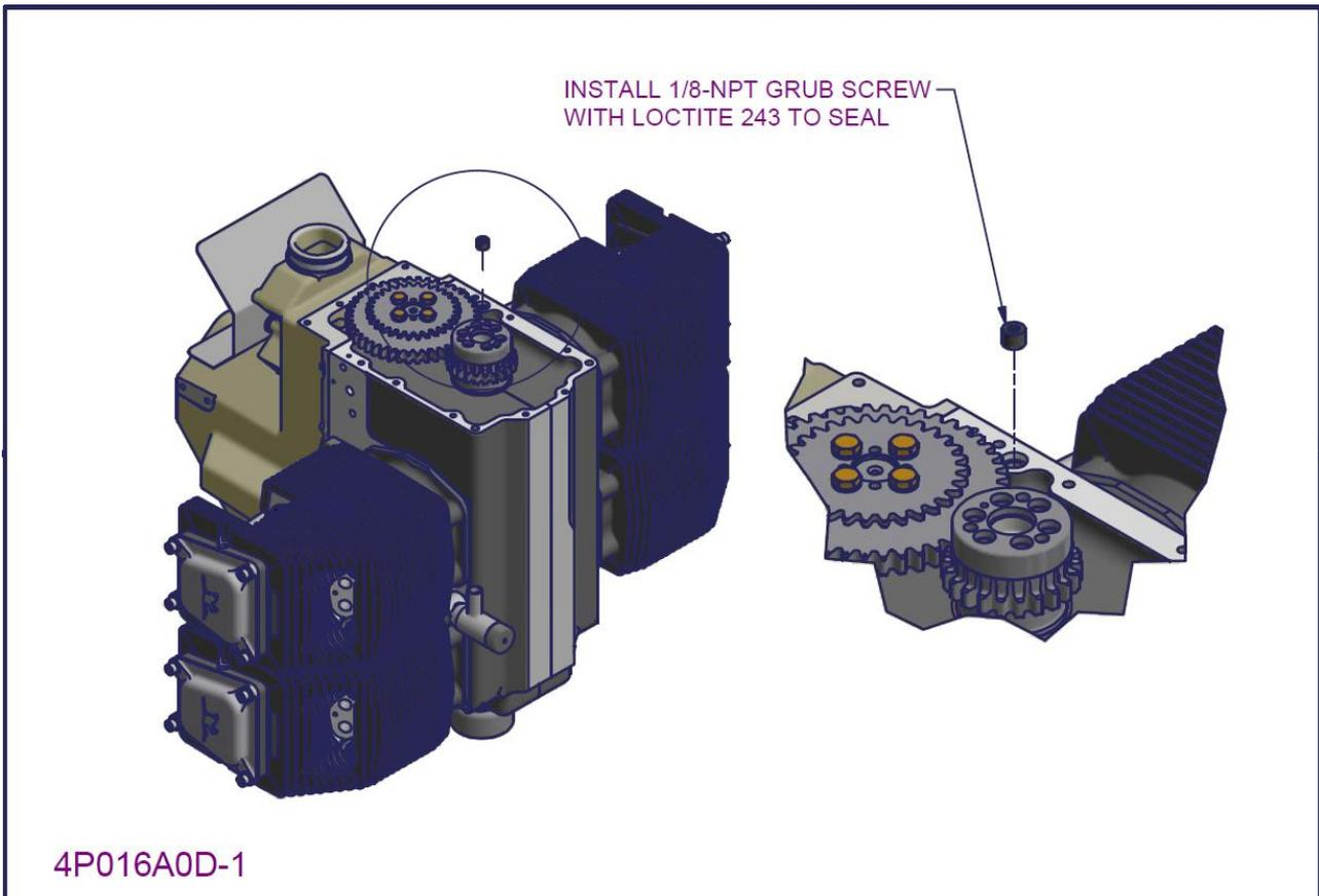
Figure 138 – 2200/3300 back plate and distributor gearbox installation 1
