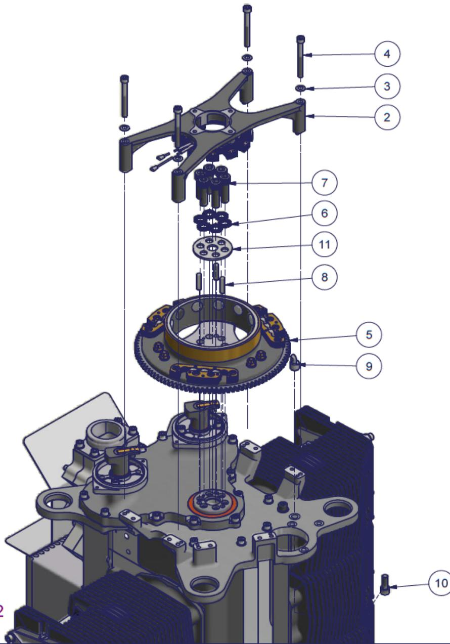
Figure 144 – 3300 flywheel and alternator installation – Parts List
