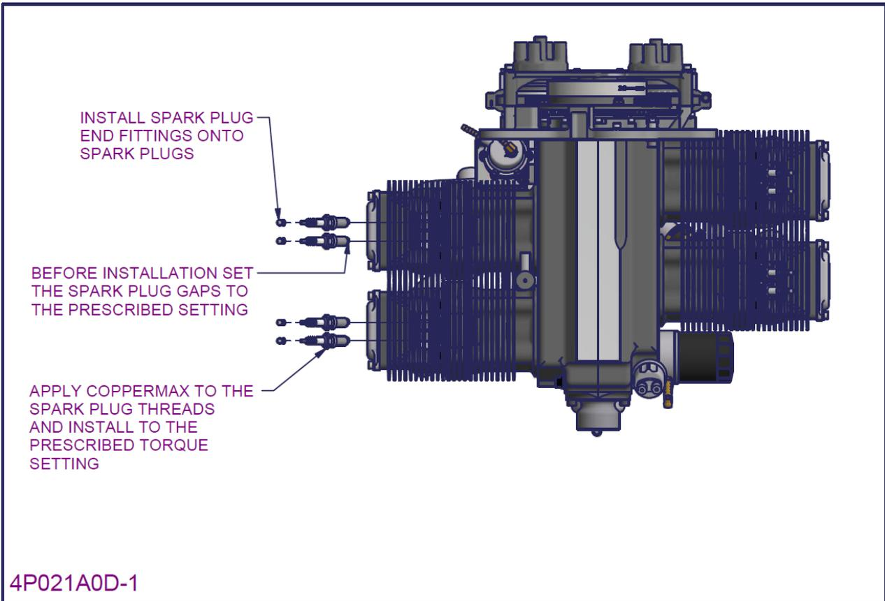
Figure 177 – 2200/3300 Ignition system installation 3
