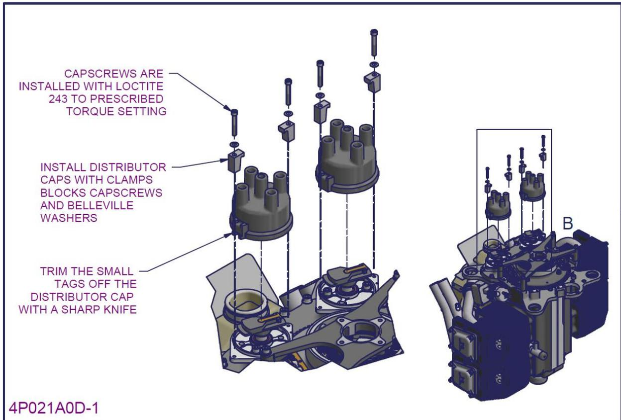
Figure 174 – 2200/3300 Ignition system installation 1
