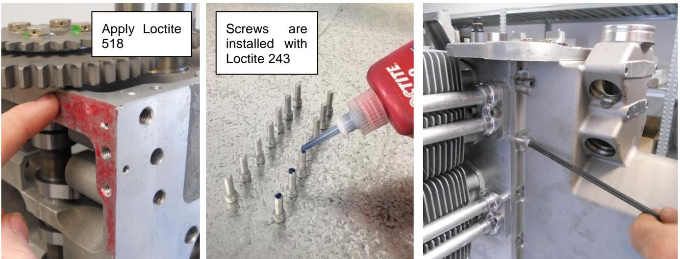
Figure 126 - Sump installation
