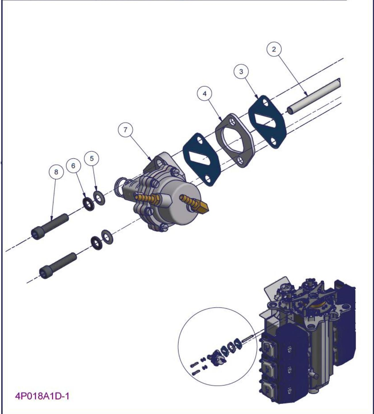
Figure 153 – 3300 Fuel pump installation – Parts List
