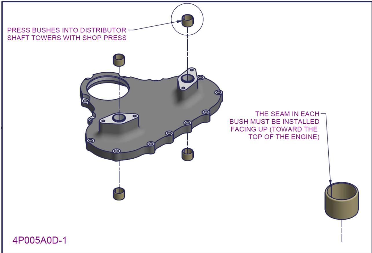
Figure 71 – 2200/3300 Distributor gearbox subassembly 1
