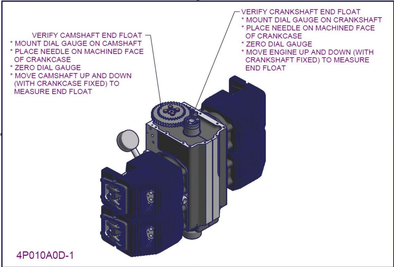
Figure 110 - 2200/3300 Joint engine assembly 5
