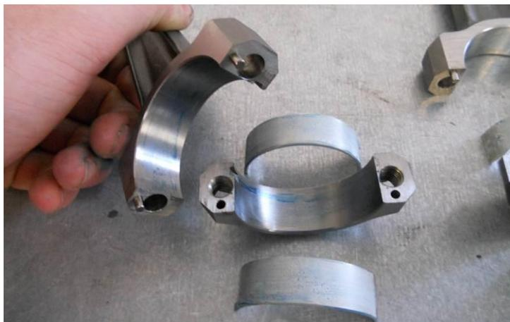
Figure 45 - Check for bearing blue transferal
