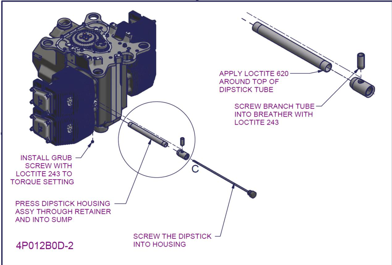
Figure 129 – 2200/3300 Sump installation 4
