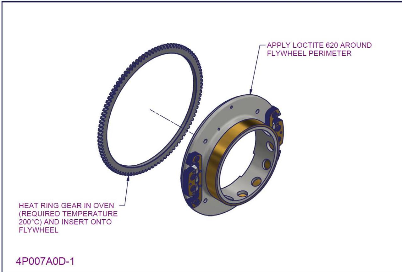
Figure 89 – 2200/3300 Flywheel subassembly (aluminium cross piece) 3
