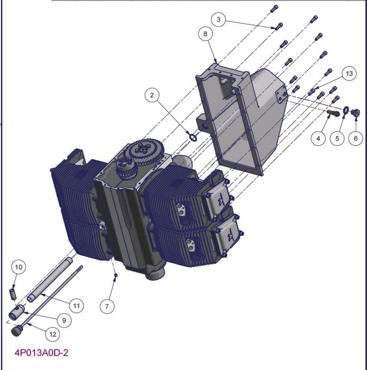
Figure 121 – 2200 Sump installation (machined plenum) – Parts List
