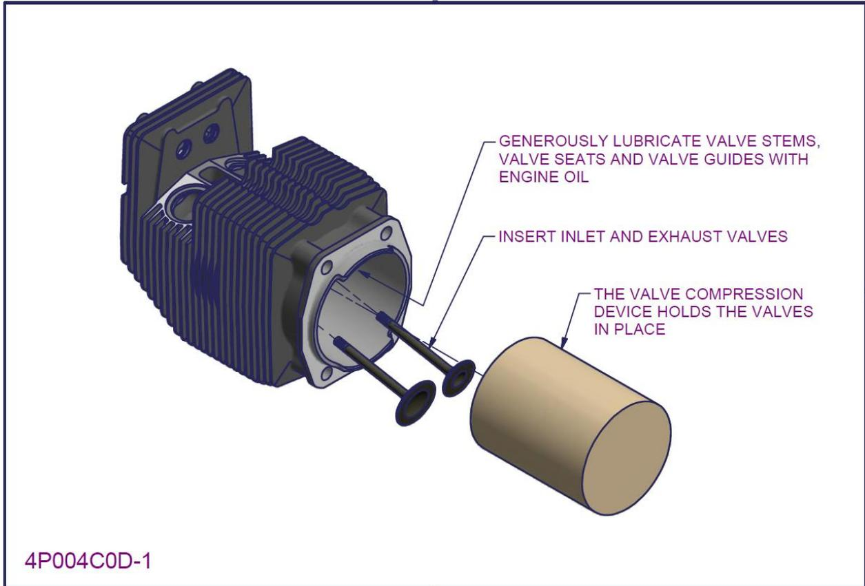
Figure 54 – 2200/3300 cylinder assembly 3
