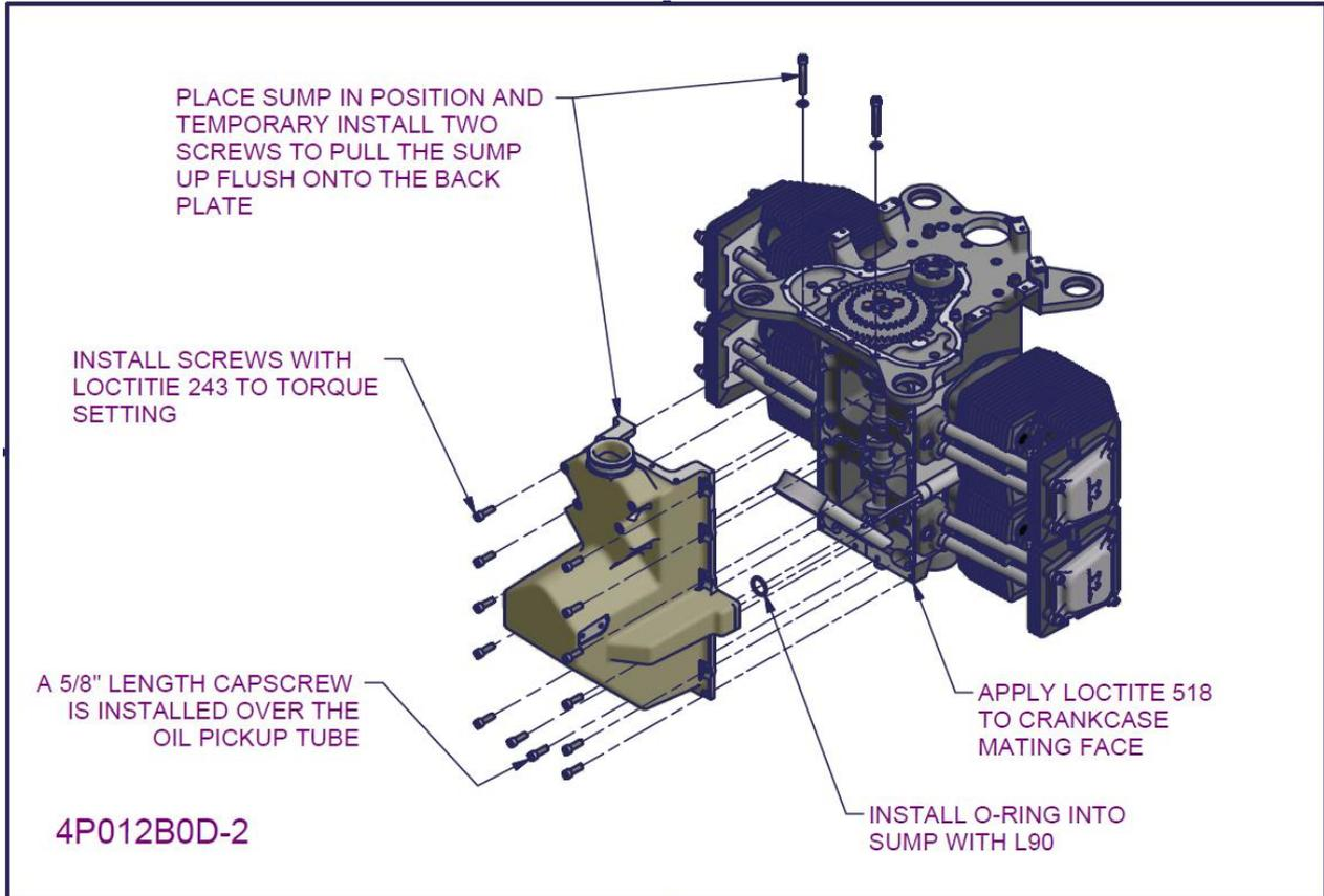
Figure 125 – 2200/3300 Sump installation 2
