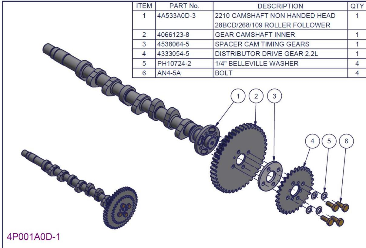
Figure 29 – 2200 Camshaft subassembly – Parts List
