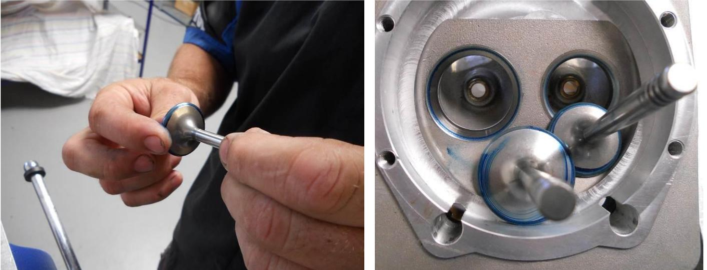
Figure 51 - checking valve sealing with bearing blue
