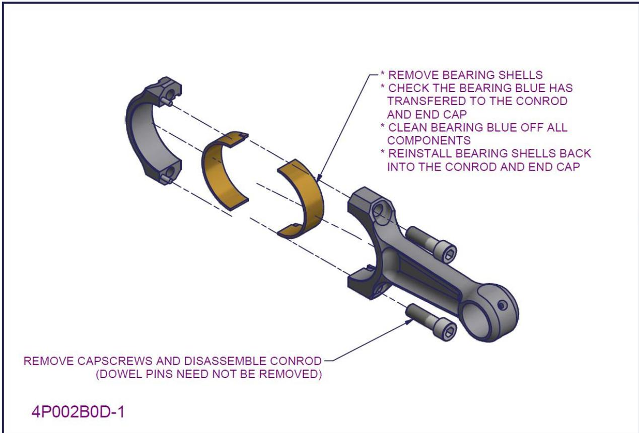
Figure 44 – 2200/3300 crankshaft subassembly 5
