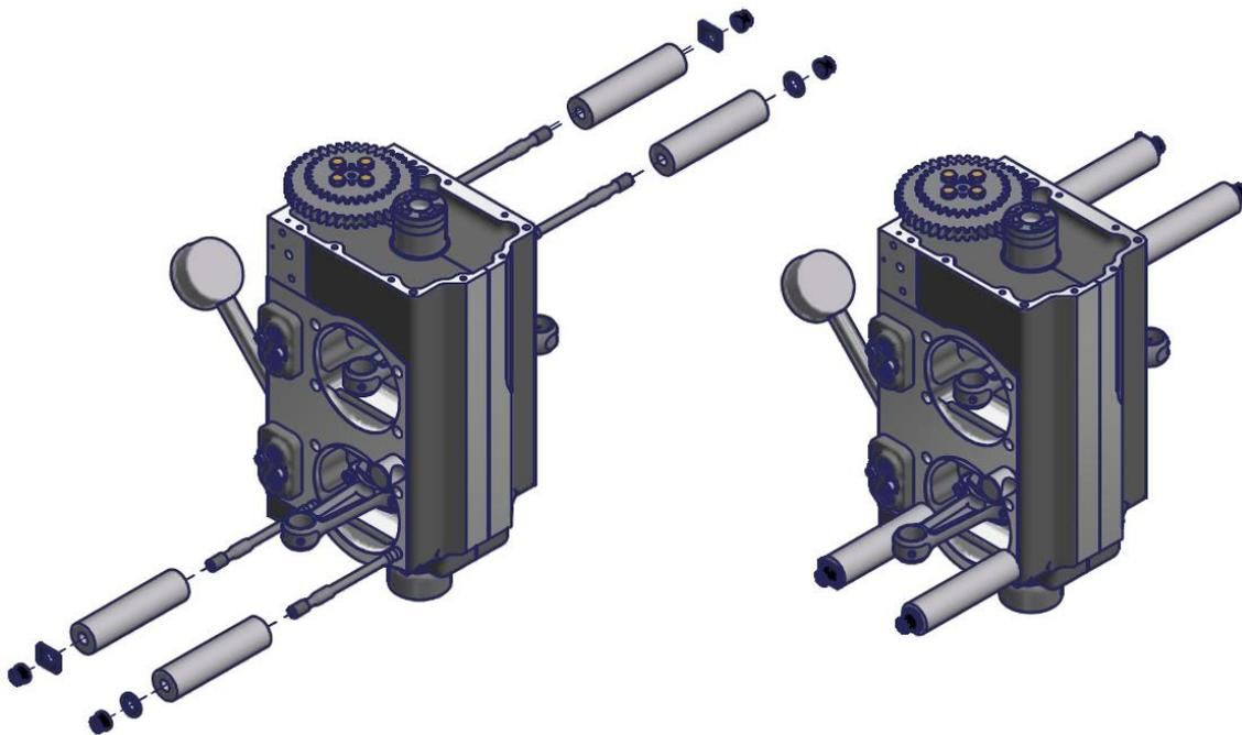
**Figure 4 - Securing crankcase halves for Top End Overhaul**
