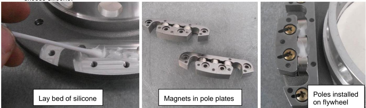
**Figure 86 - Flywheel ignition magnets and pole plate installation**
