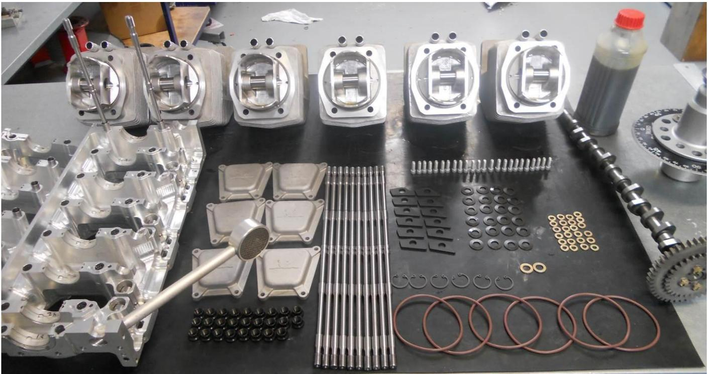
**Figure 102 - Engine assemblages, hardware and tools laid out ready to join the engine**
