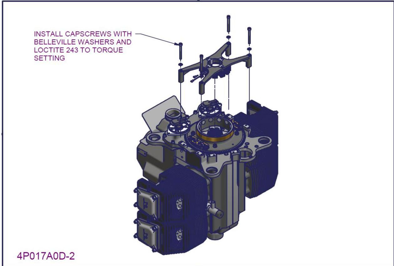
Figure 148 – 2200/3300 flywheel and alternator installation 2
