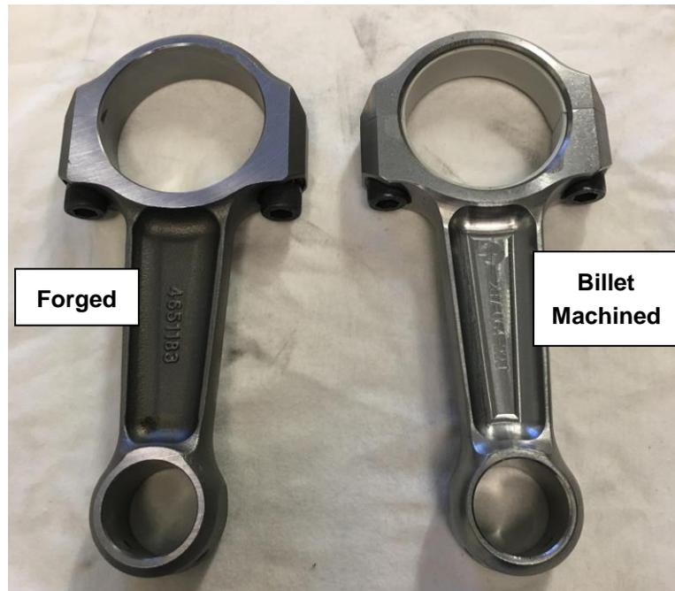
Figure 41 - Forged conrods vs Billet machined conrods
