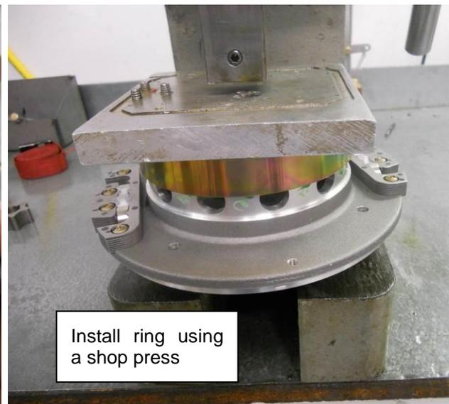
Figure 88 - Alternator magnet ring installation
