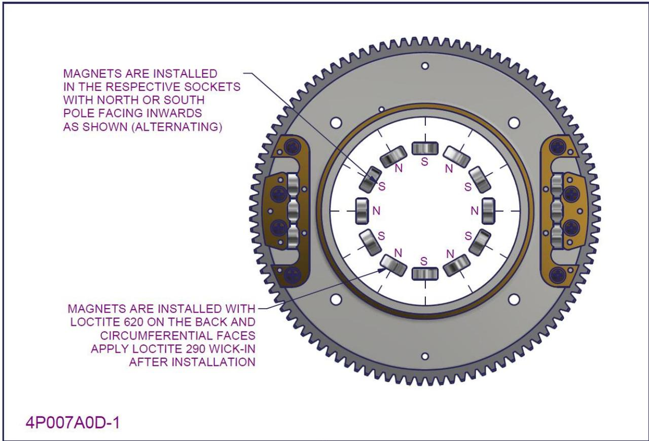
Figure 91 - 2200/3300 Flywheel subassembly (aluminium cross piece) 3
