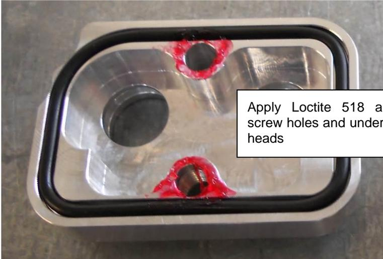
Apply Loctite 518 around the screw holes and under the screw heads
