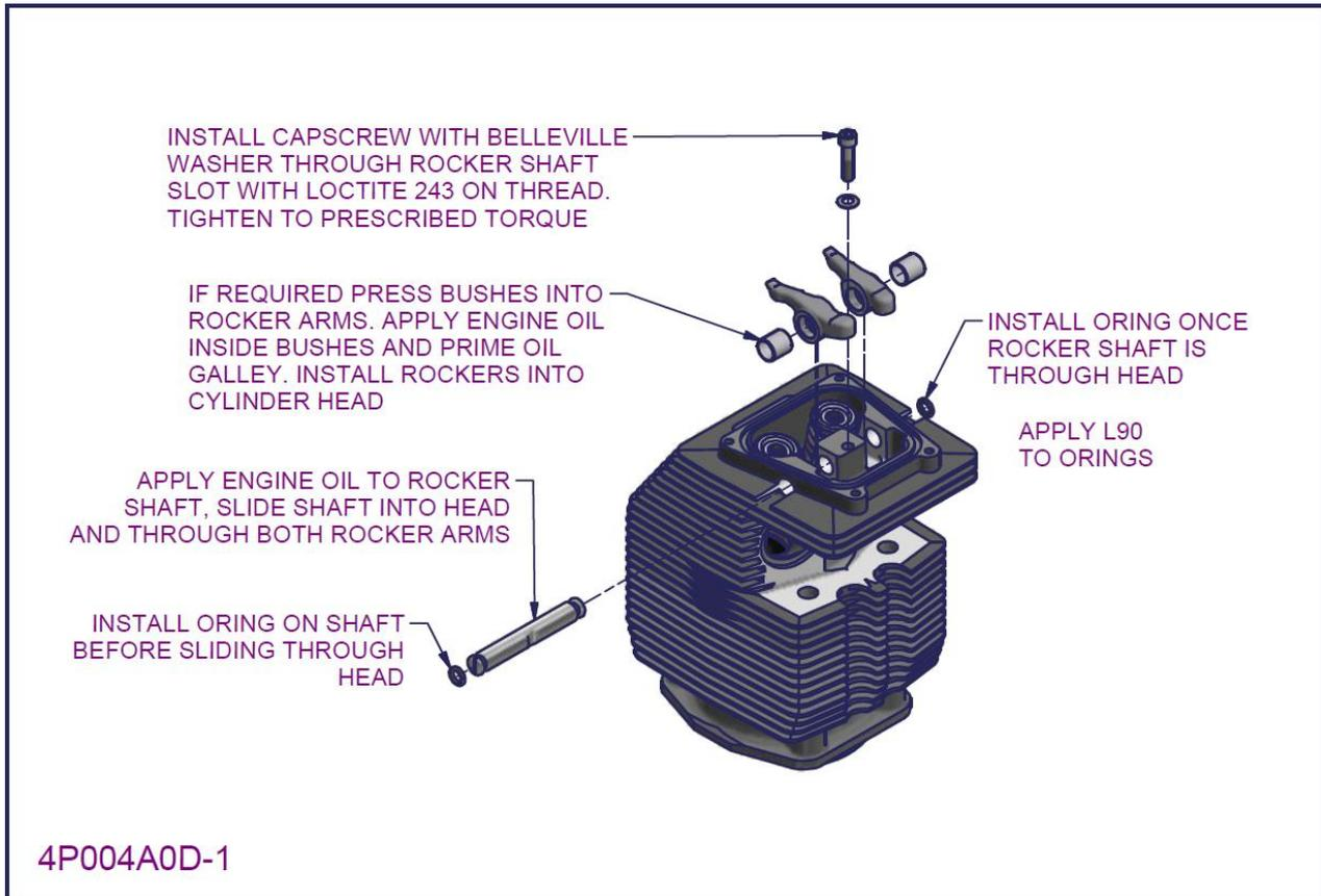
Figure 60 – 2200/3300 cylinder assembly 6
