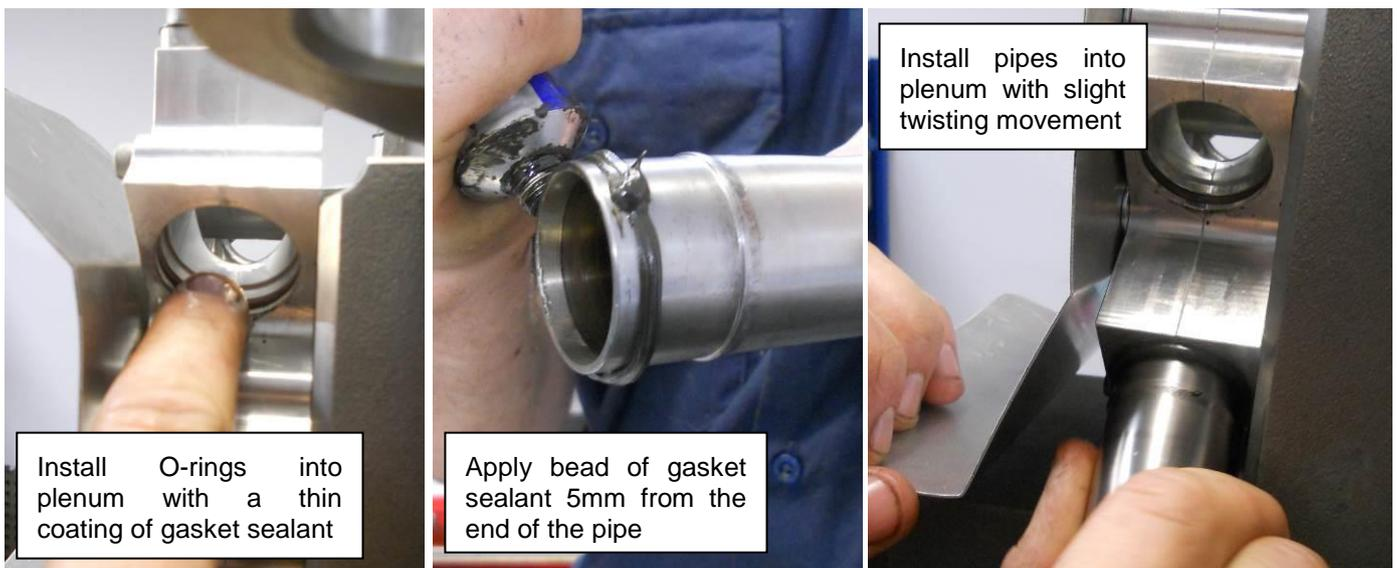
Figure 167 - Lower induction pipe installation
