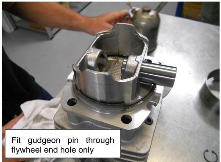
Figure 66 – Piston installation into the cylinder barrel
