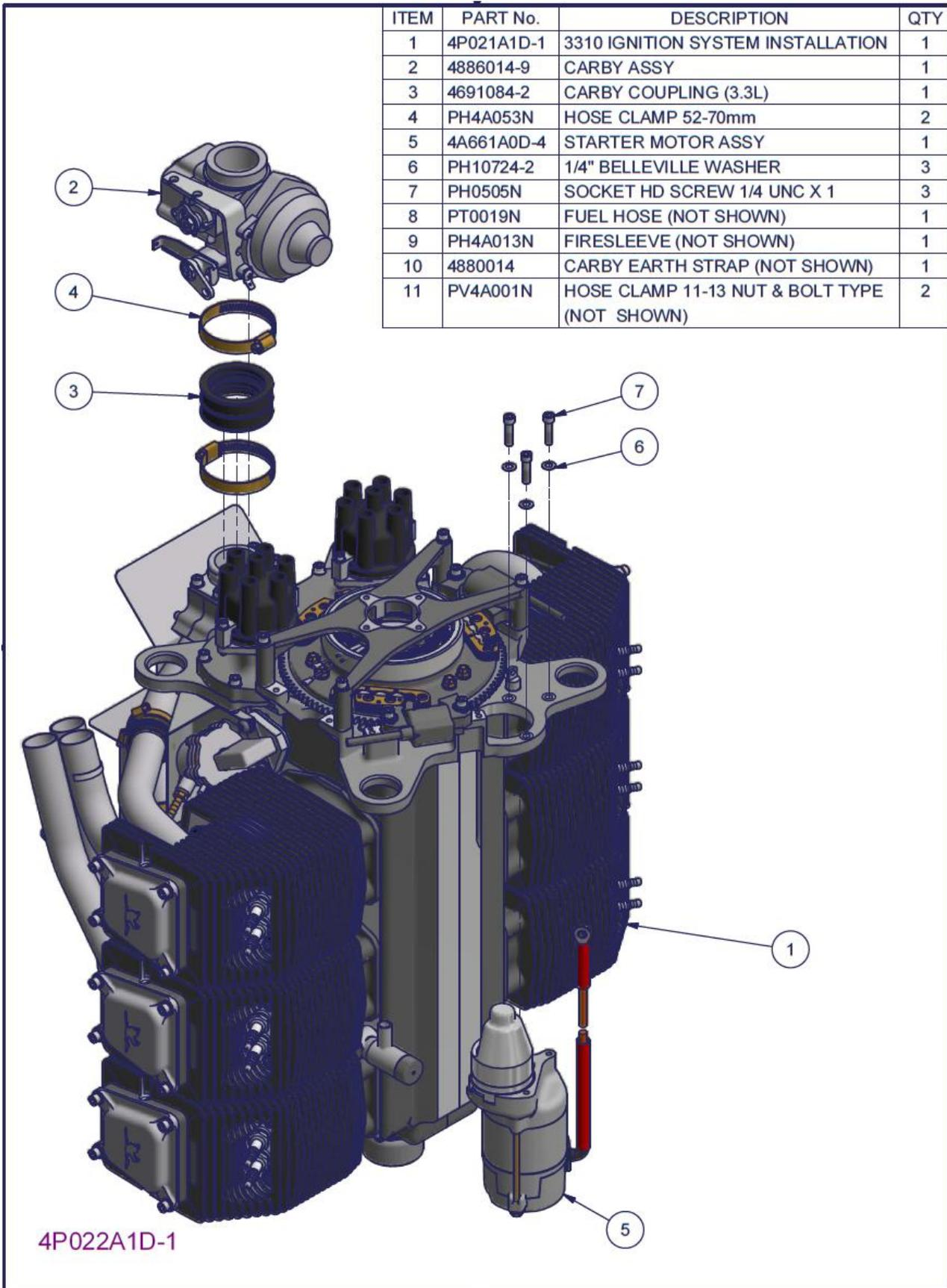
Figure 182 – 3300 Carburettor and Starter installation – Parts List
