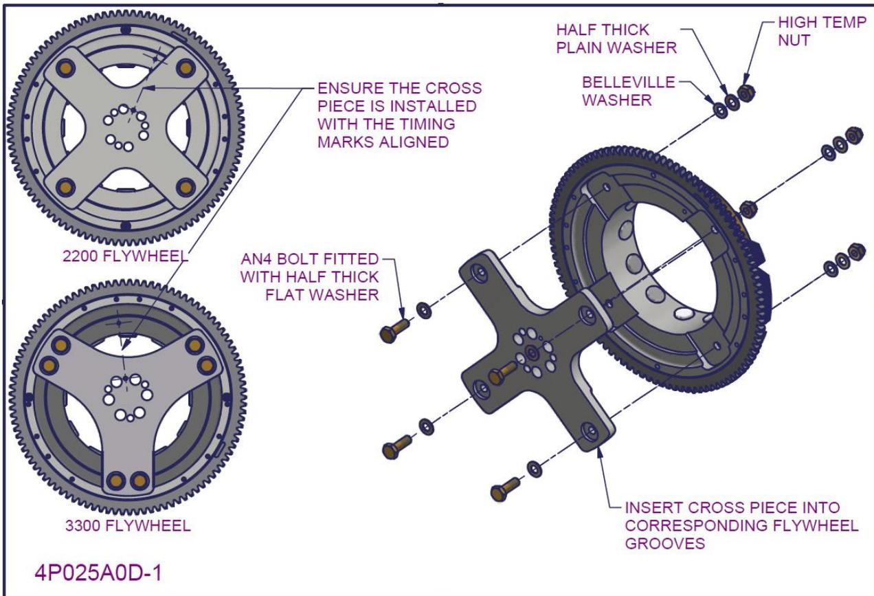
Figure 93 - 2200/3300 Flywheel subassembly (aluminium cross piece) 4
