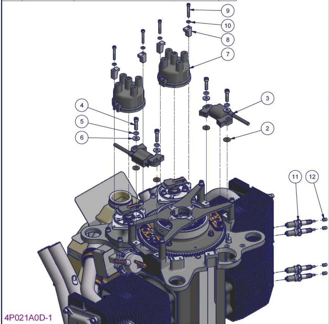
Figure 172 – 2200 Ignition system installation – Parts List
