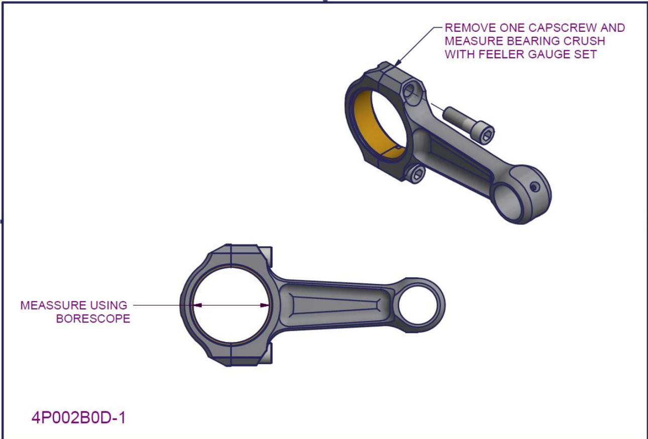
Figure 42 - 2200/3300 crankshaft subassembly 4
