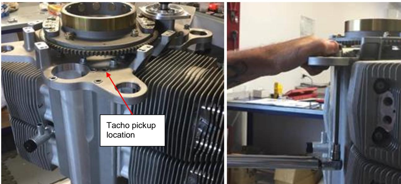
Figure 151 – Tacho pickup installation
