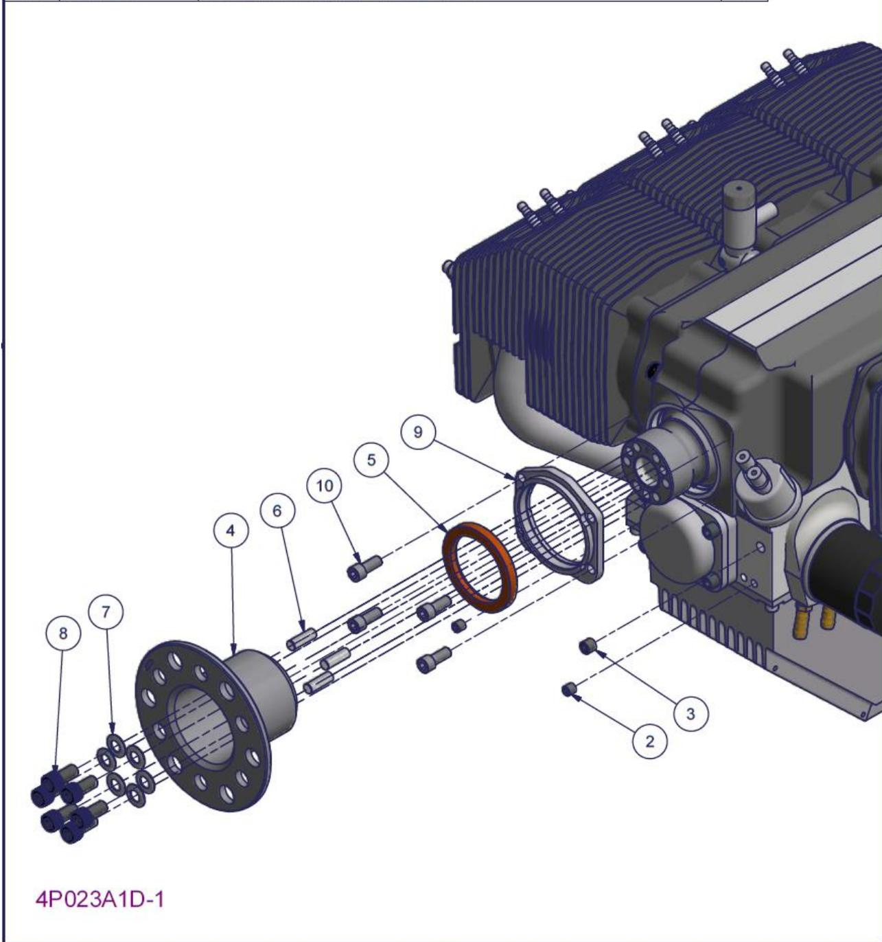
Figure 187 – 2200/3300 Front seal and propeller flange (separate seal housing) – Parts List
