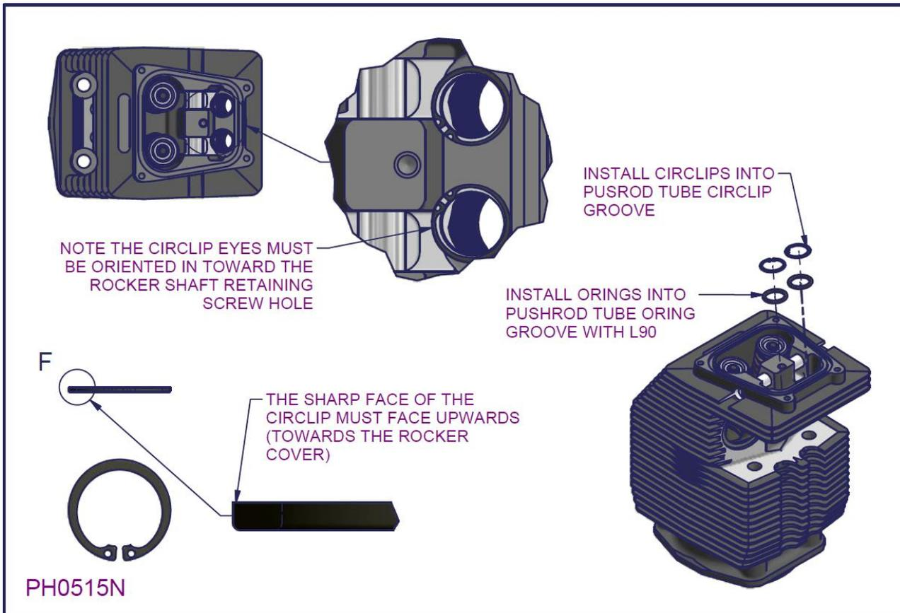
Figure 59 – 2200/3300 cylinder assembly 5b (Internal O-ring groove cylinder head)
