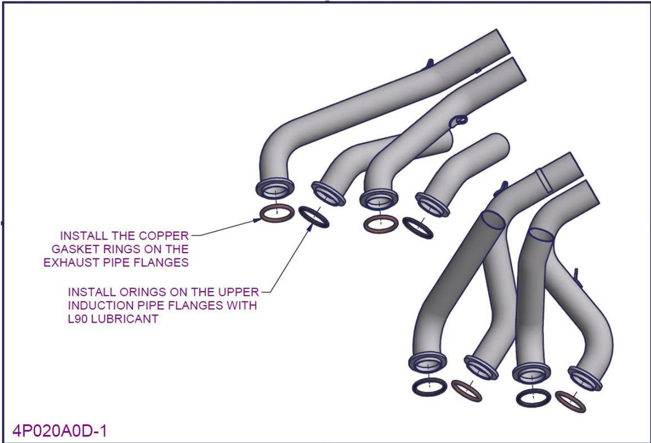
Figure 165 – 2200/3300 Exhaust and induction pipe installation 1
