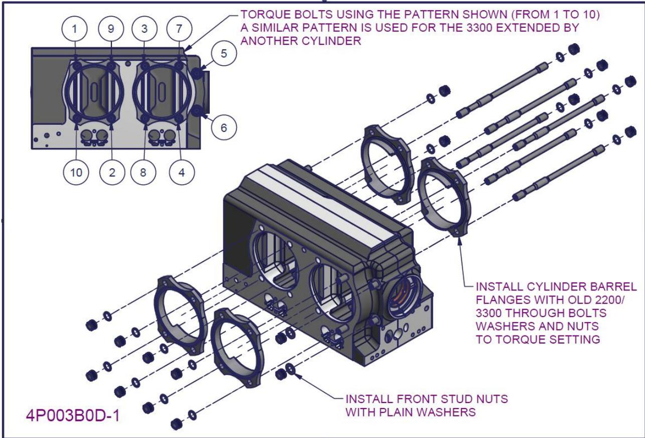
Figure 14 – 2200/330 crankcase subassembly 3
