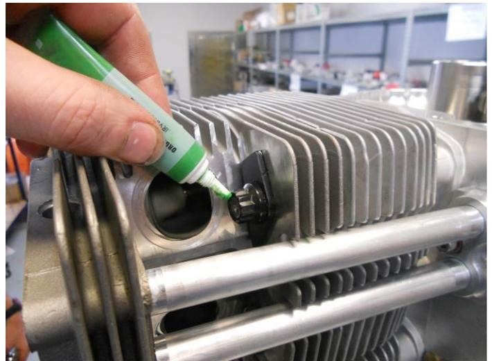
Figure 109 - Installing washers, nuts and tightening to torque
