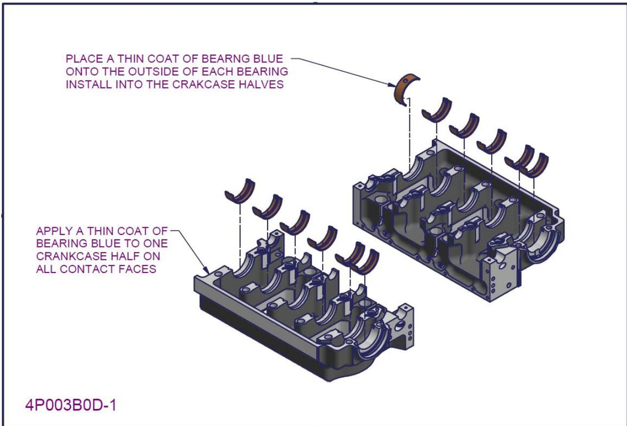
Figure 10 – 2200/3300 crankcase subassembly 1
