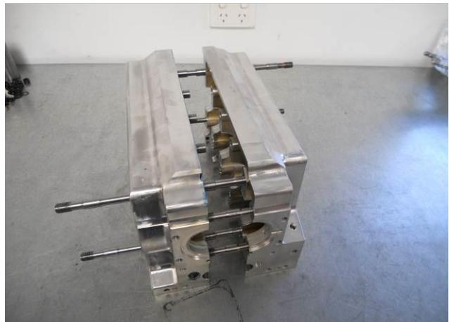
Figure 13 - Installing dowels and studs, pressing crankcase halves together
