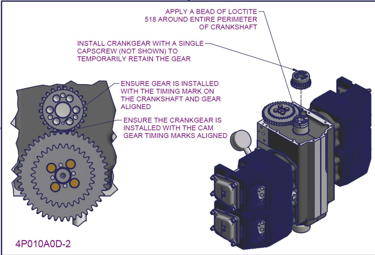
Figure 113 – 2200/3300 Joint engine assembly 7
