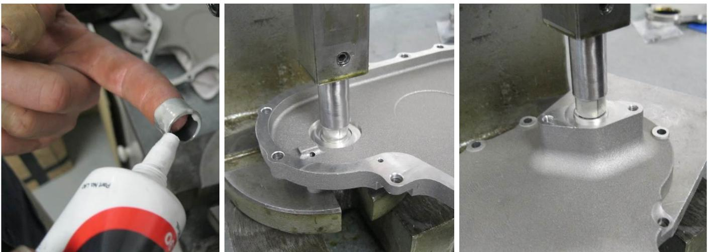
Figure 72 - Distributor shaft bush installation
