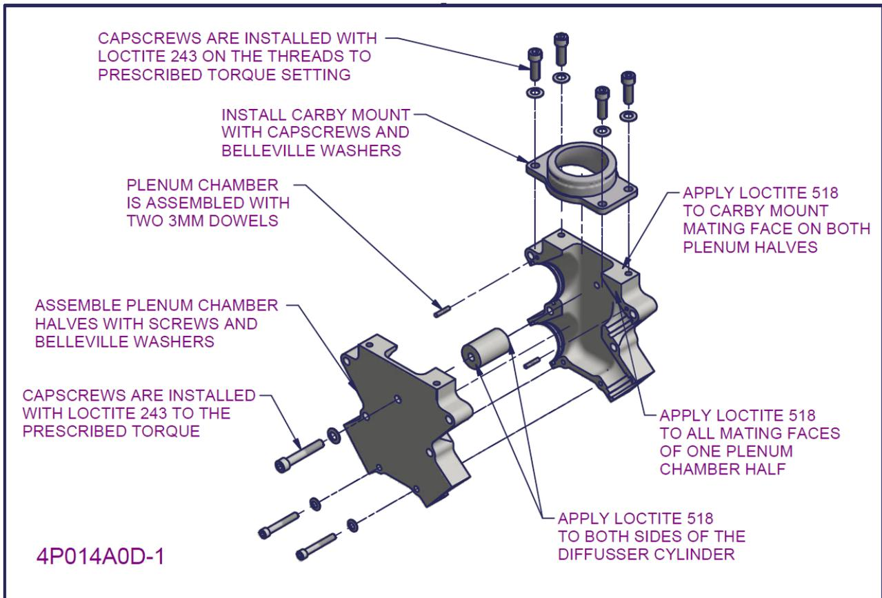
Figure 134 – 2200/3300 Plenum and Heat shield installation 1
