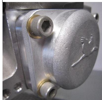
Installed oil pump assembly with washers under the cap screws.
