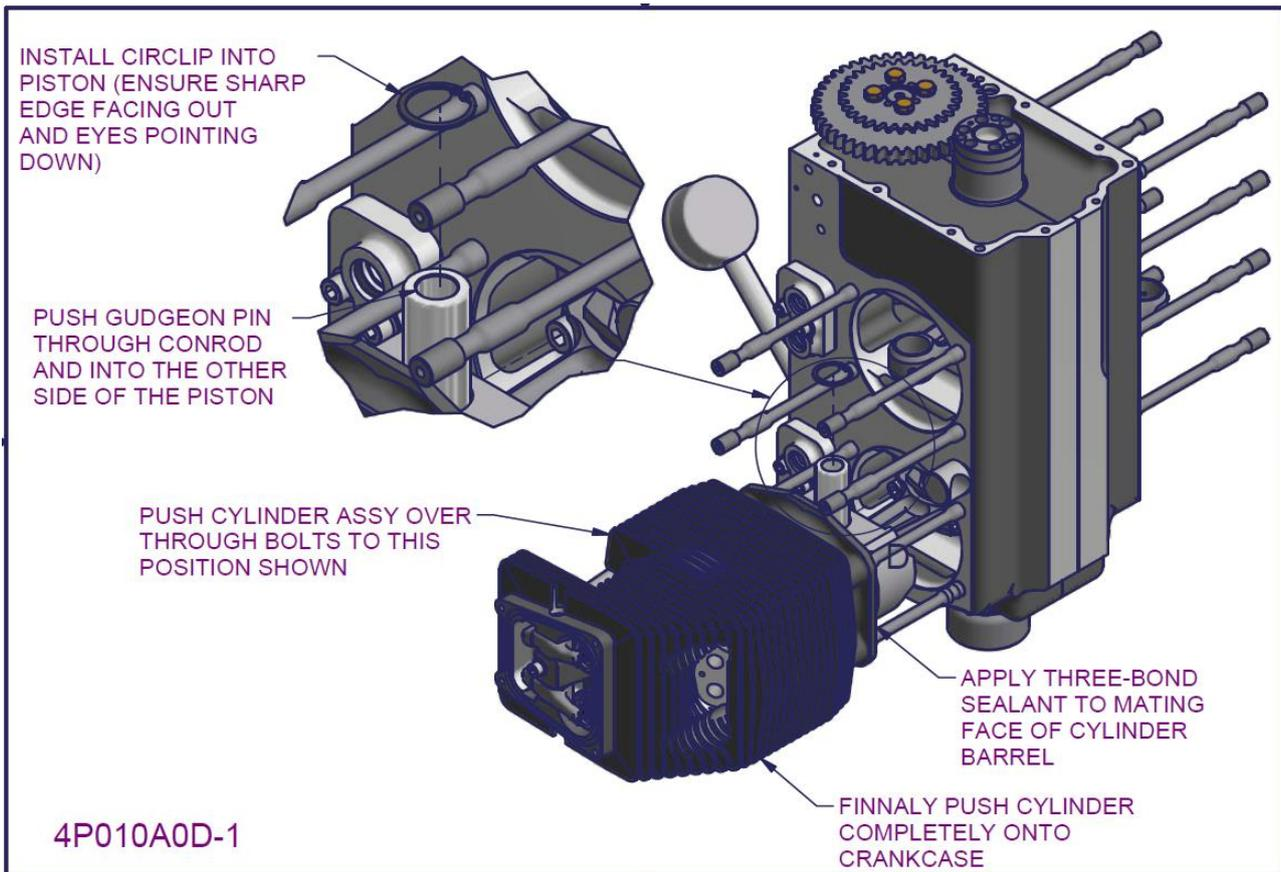
Figure 106 - 2200/3300 Joint engine assembly 3
