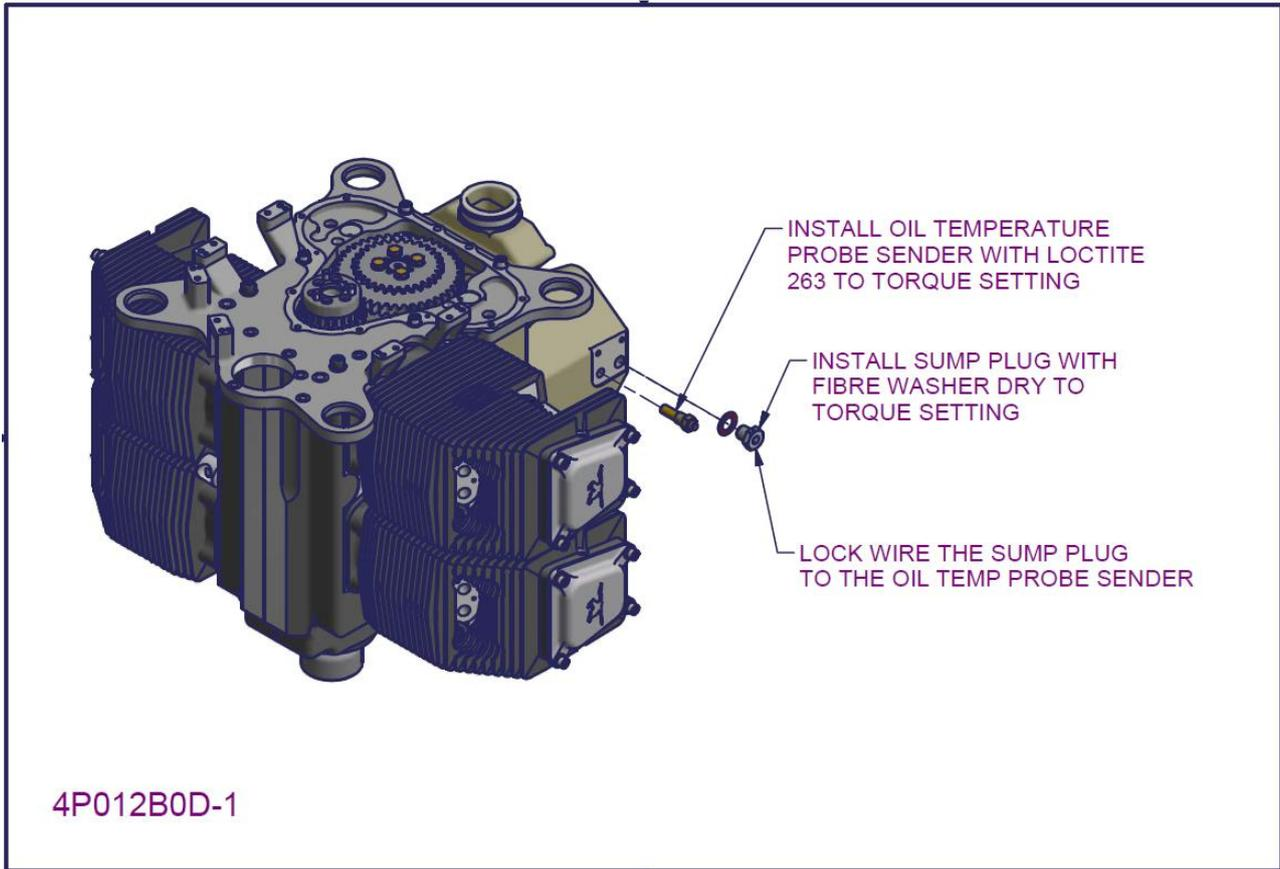
Figure 127 – 2200/3300 Sump installation 3
