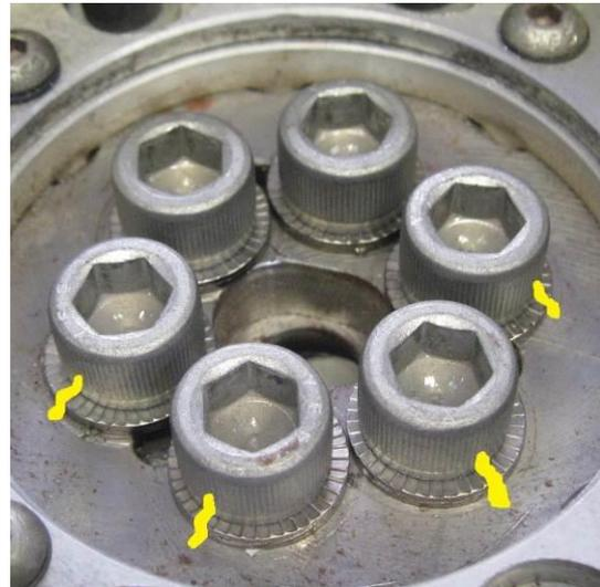
Repeat for the other five screws **ONE AT A TIME** using the diagonal pattern shown in section 0)
