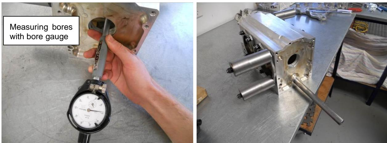
Figure 16 - Measuring Crankcase bearing and camshaft bores
