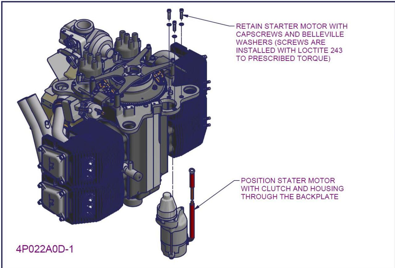
Figure 185 – 2200/3300 Carburettor and starter installation 2
