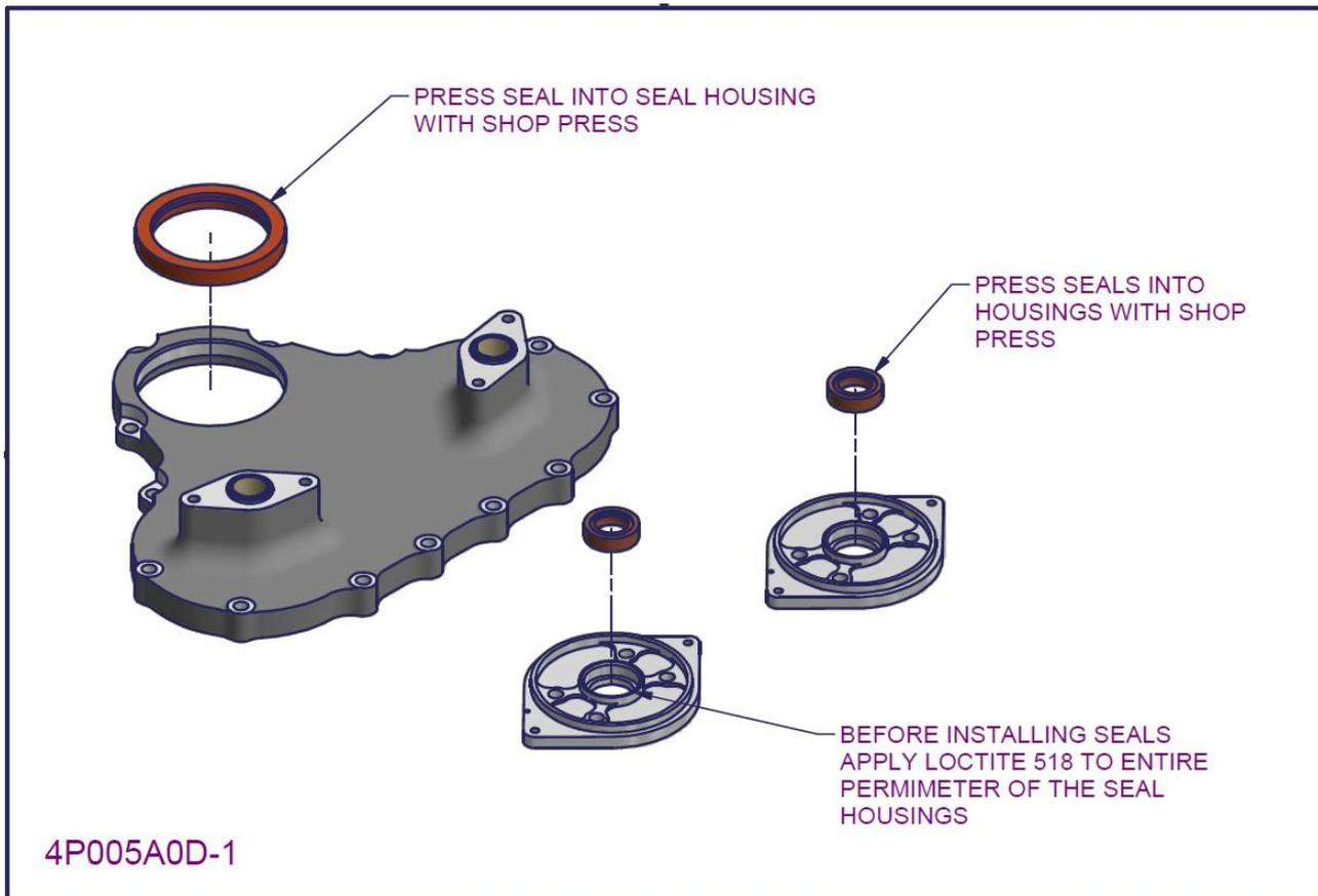
Figure 73 – 2200/3300 Distributor gearbox subassembly 2
