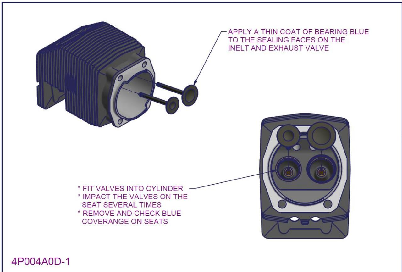
Figure 50 – 2200/3300 cylinder assembly 1
