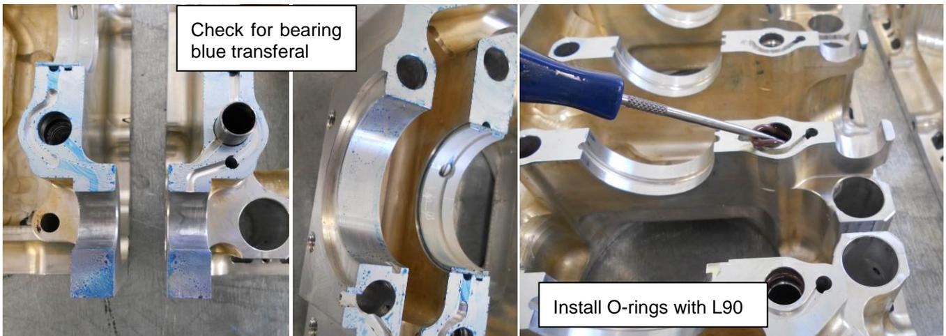
Figure 18 – Bearing blue inspection and O-ring installation
