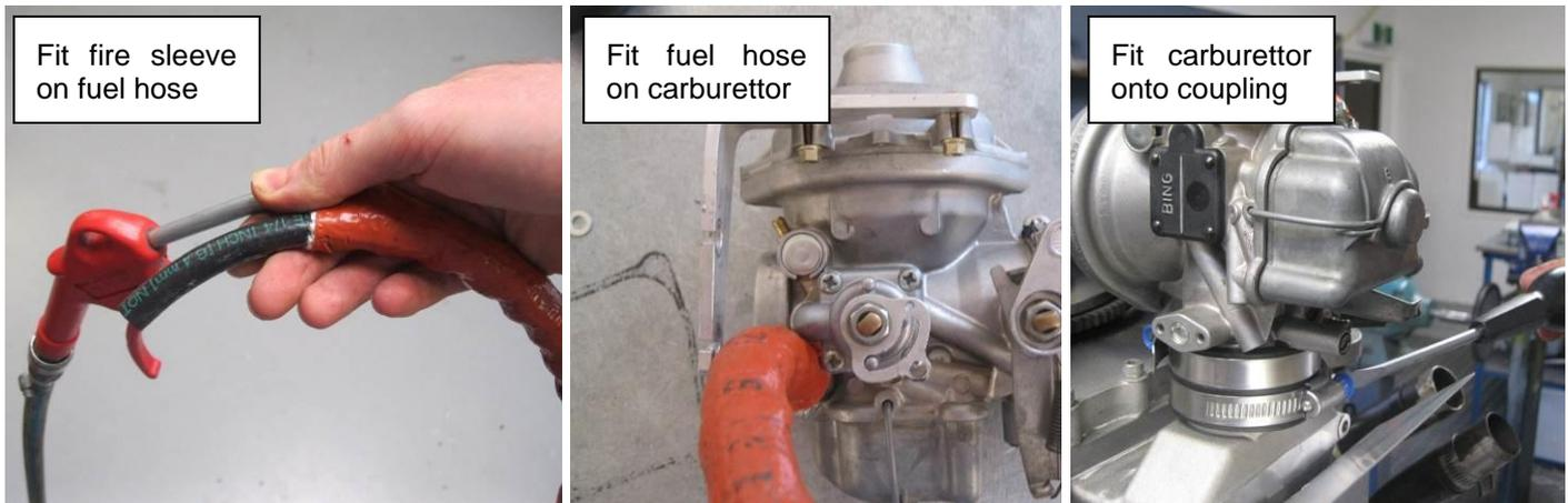
Figure 184 – Carburettor installation
