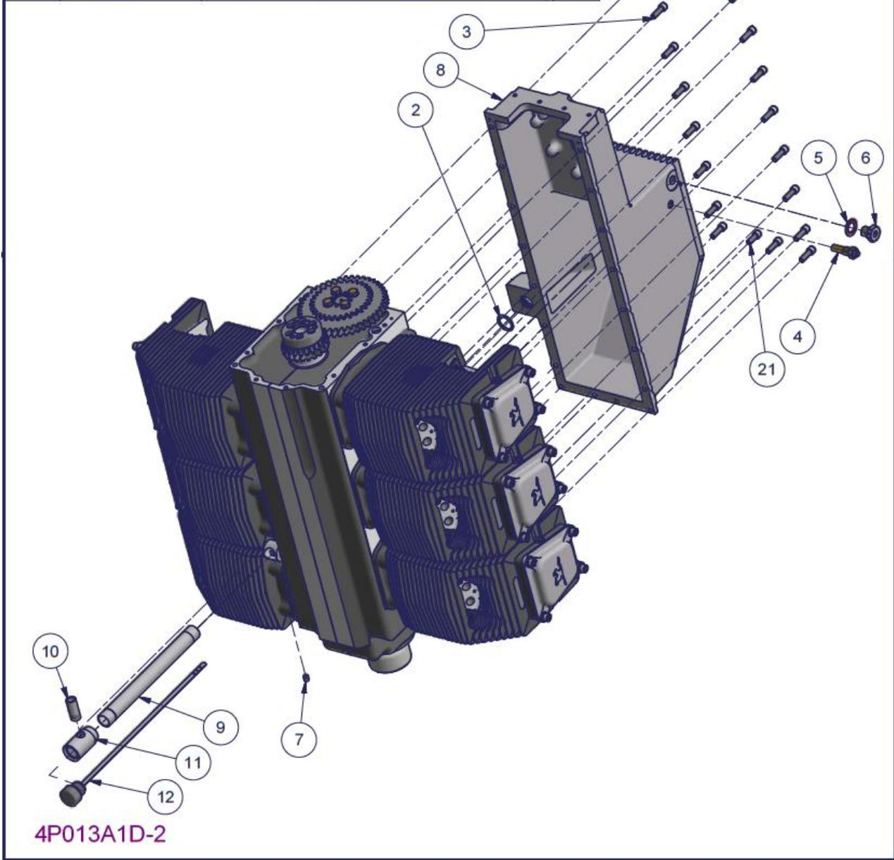
Figure 123 – 3300 Sump installation (No plenum) – Parts List
