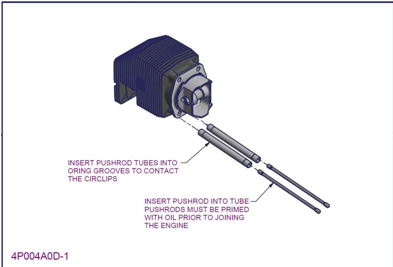
Figure 68 - 2200/3300 cylinder assembly 10b (Internal O-ring groove cylinder head)
