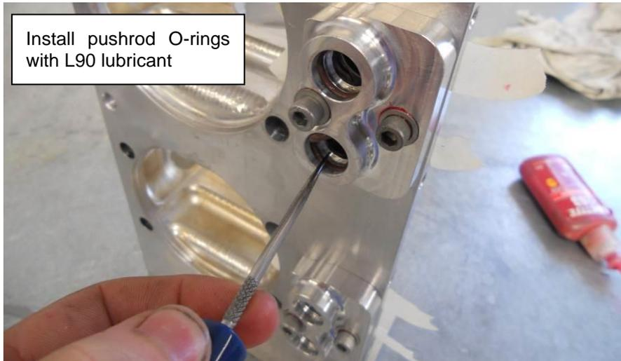
Install pushrod O-rings with L90 lubricant
