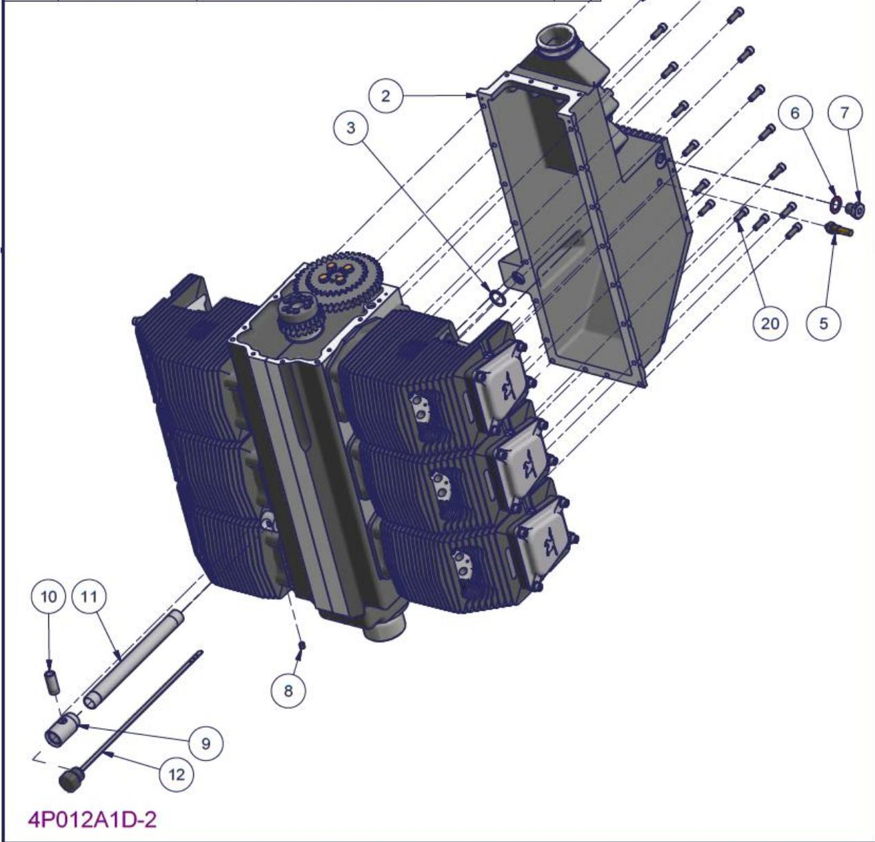
Figure 122 – 3300 Sump installation (integral plenum) – Parts List
