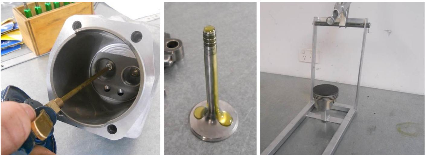
Figure 55 - Lubricating valves, seats and guides
