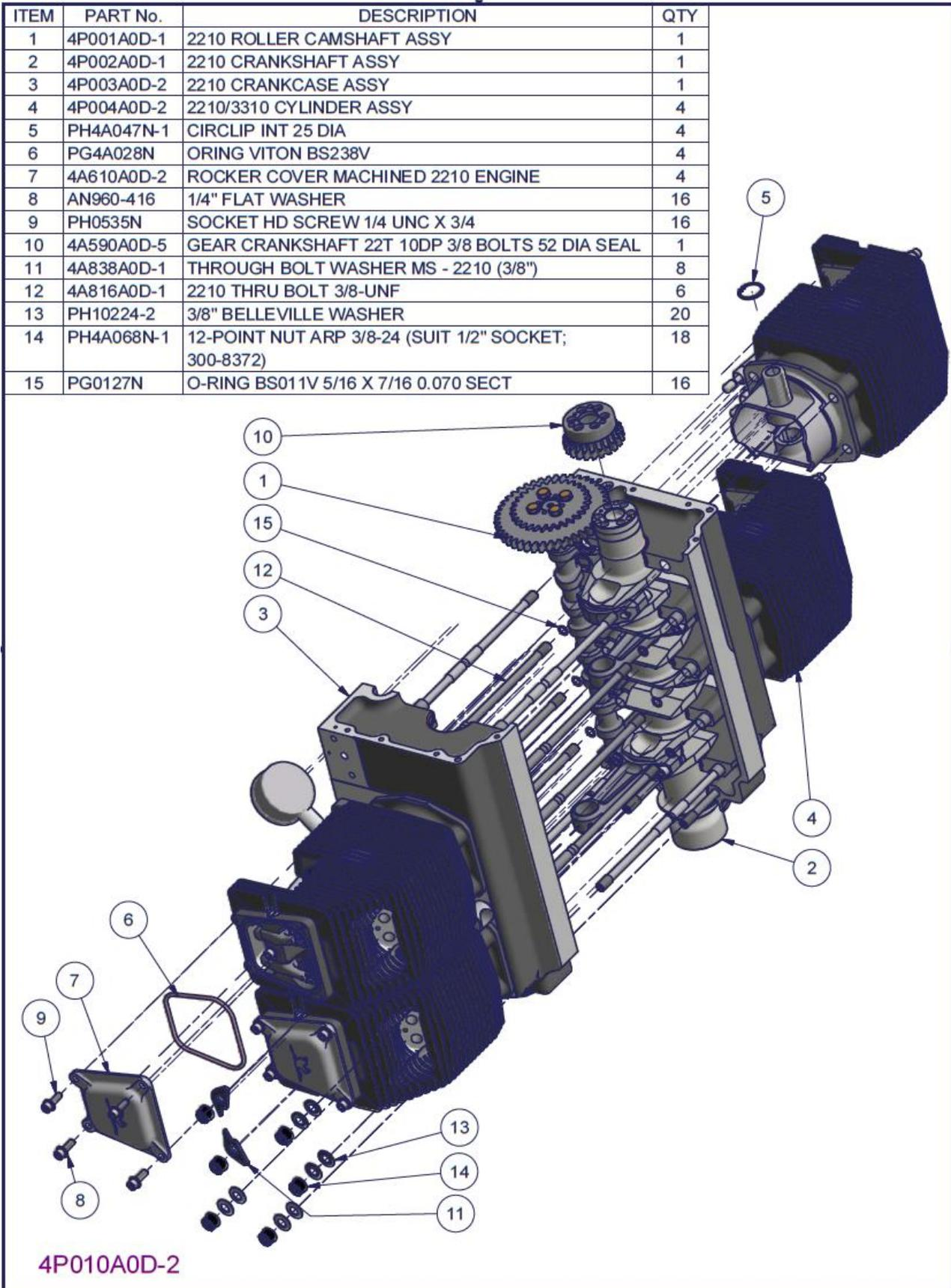
Figure 100 – 2200 Joint engine – Parts list
