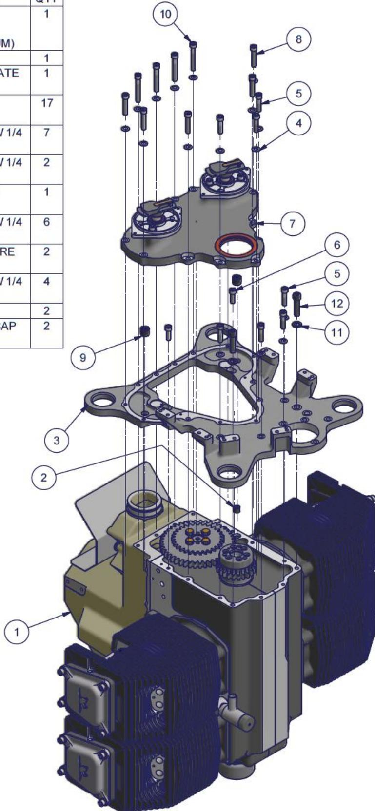
Figure 136 – 2200 back plate and distributor gearbox installation – Parts List
