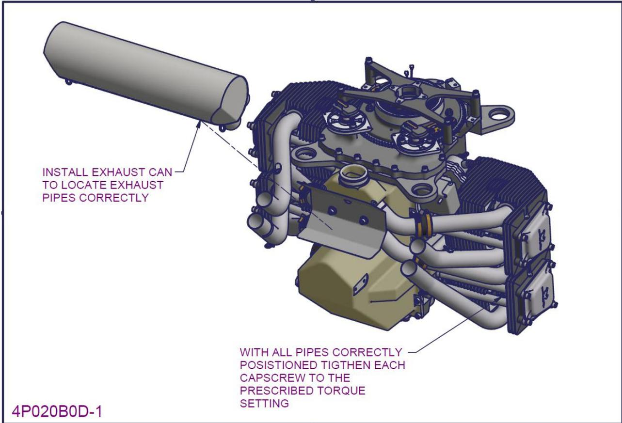
Figure 170 – 2200/3300 Exhaust and induction pipe installation 4
