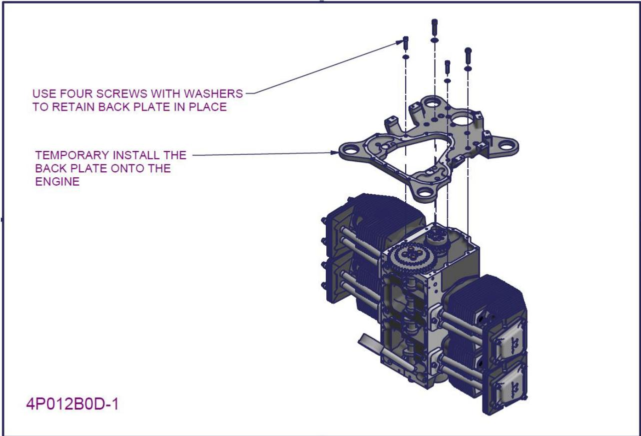
**Figure 124 – 2200/3300 Sump installation 1**
