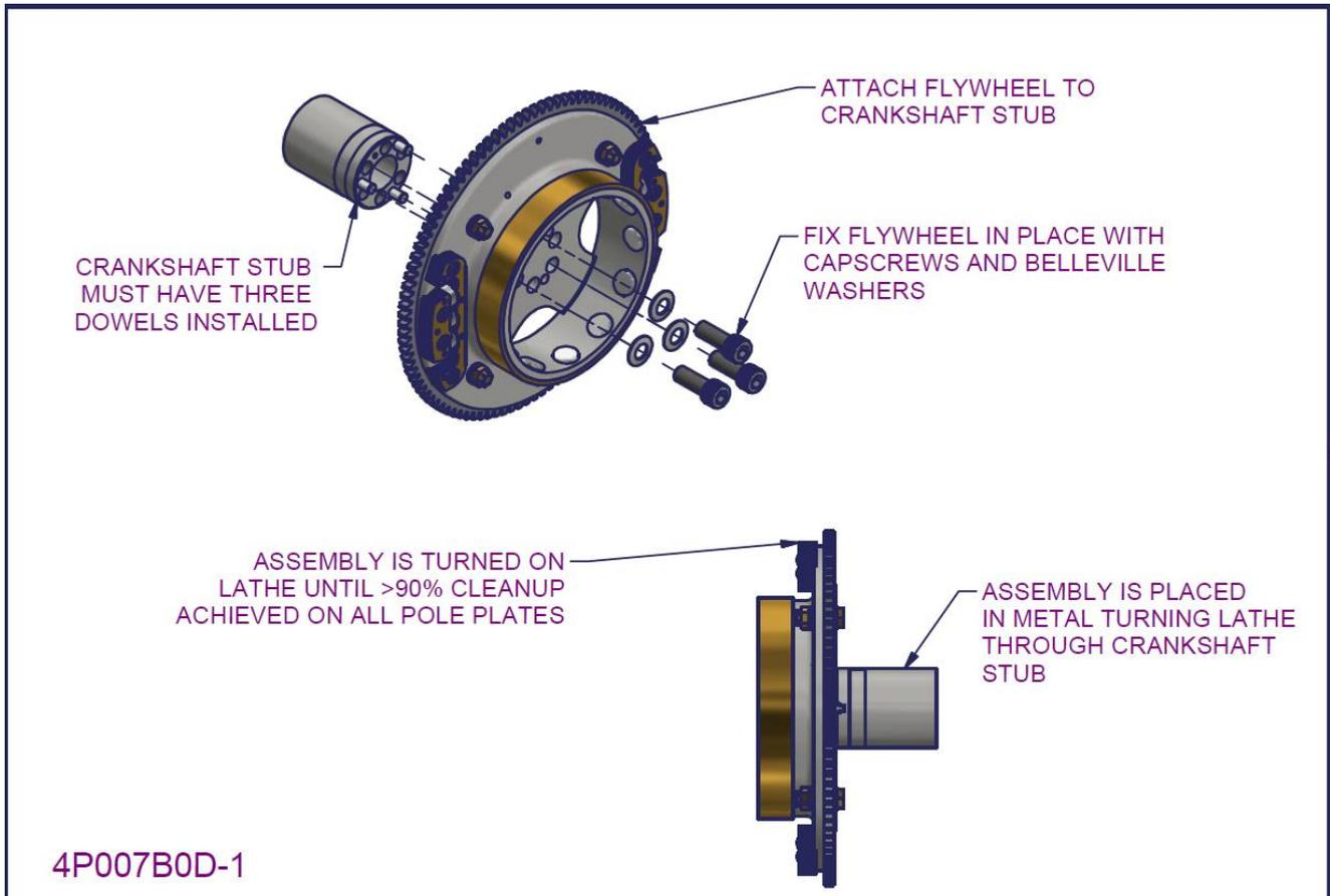
Figure 95 - 2200/3300 Flywheel subassembly (aluminium cross piece) 6
