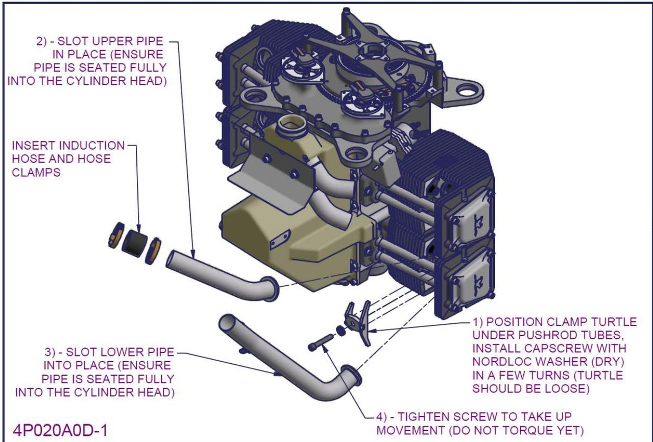
Figure 168 – 2200/3300 Exhaust and induction pipe installation 3
