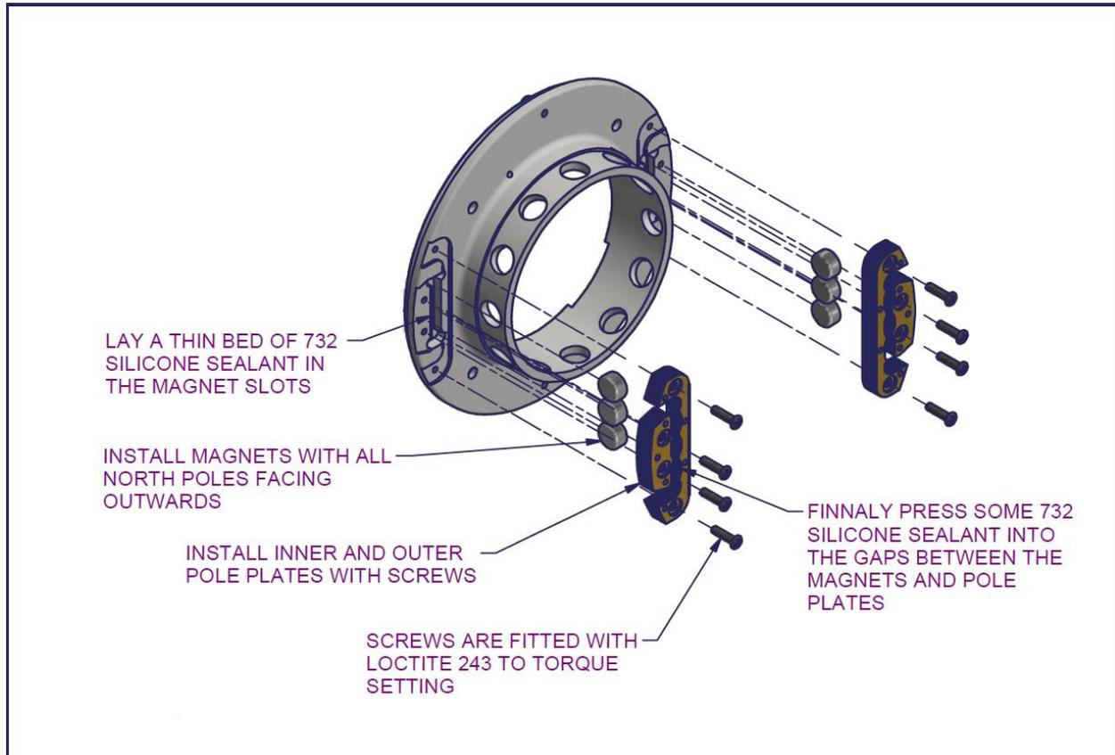
**Figure 85 – 2200/3300 Flywheel subassembly (aluminium cross piece) 1**
