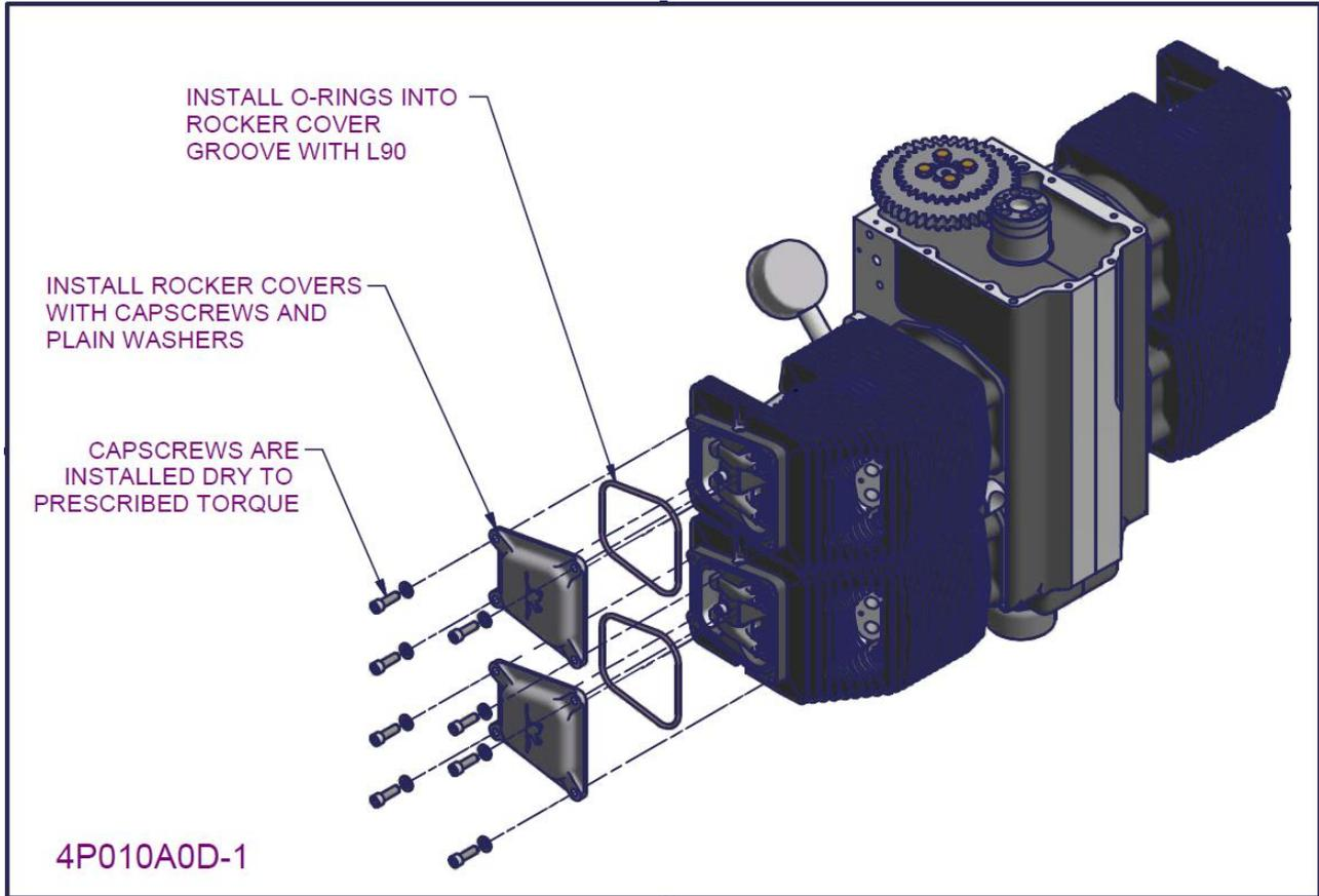
Figure 112 - 2200/3300 Joint engine assembly 6
