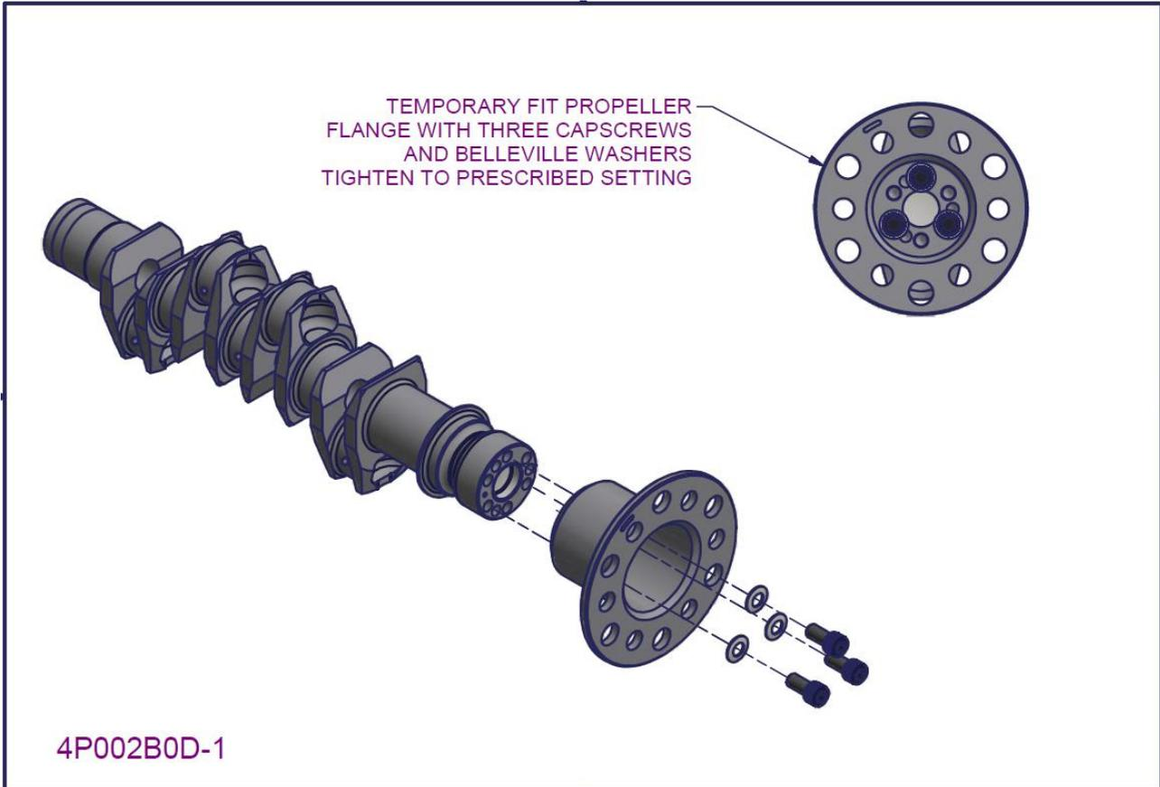
Figure 37 - 2200/3300 crankshaft subassembly 2
