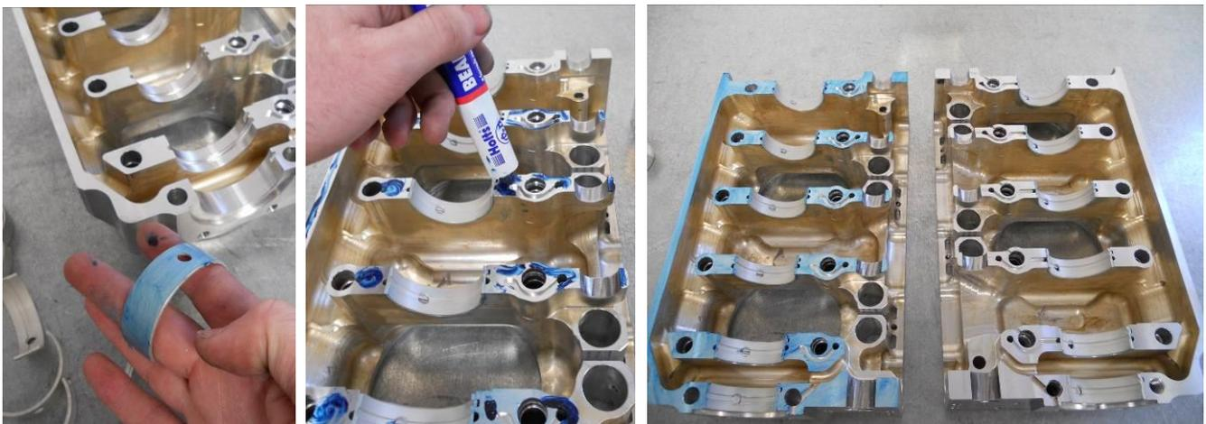
Figure 11 - Applying bearing blue to bearing shells and crankcase half
