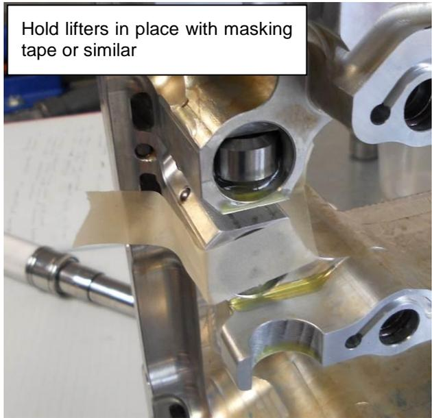
Hold lifters in place with masking tape or similar
