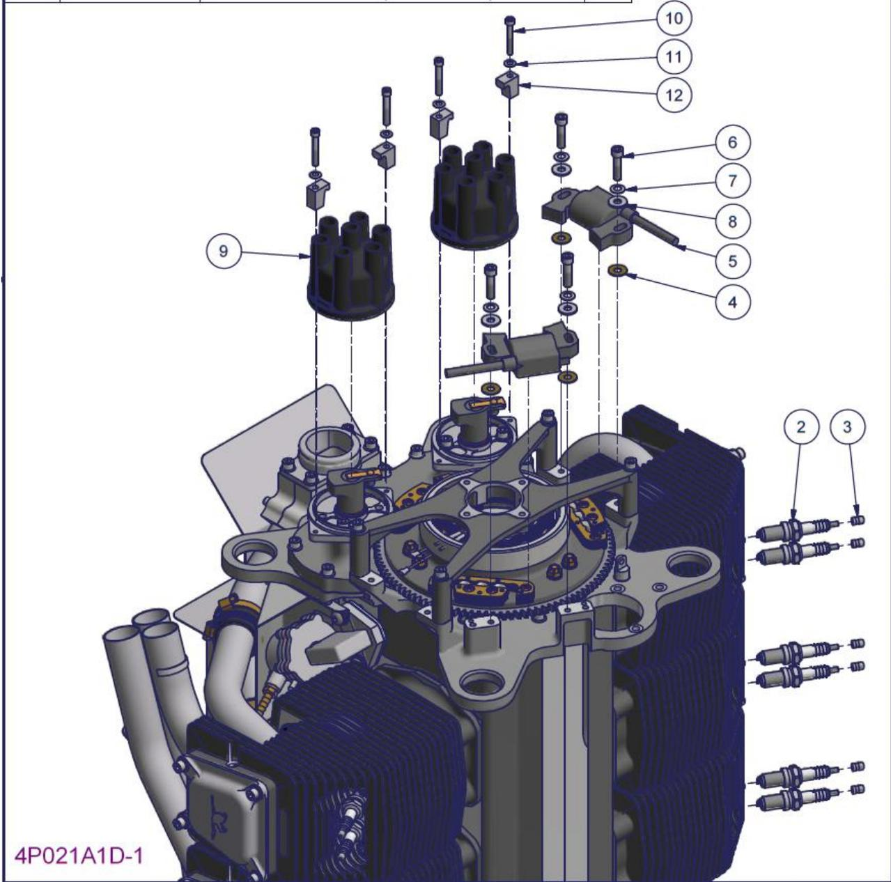
Figure 173 – 3300 Ignition system installation – Parts List
