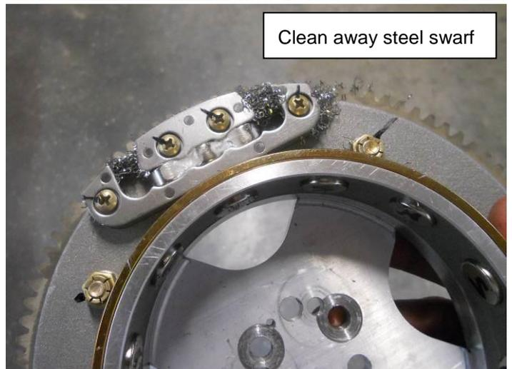
Figure 96 - Flywheel pole plate skimming
