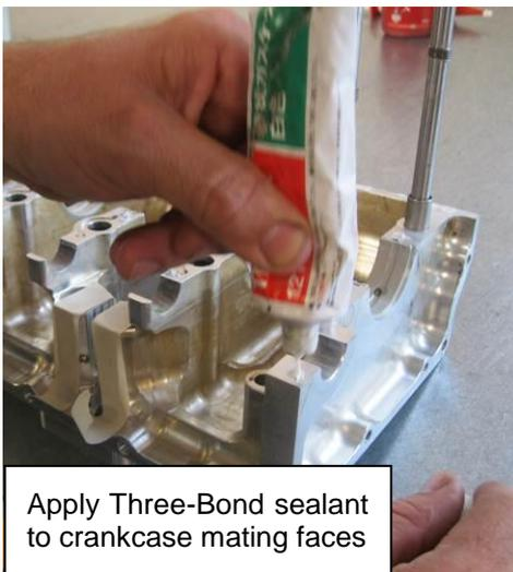
Apply Three-Bond sealant to crankcase mating faces
