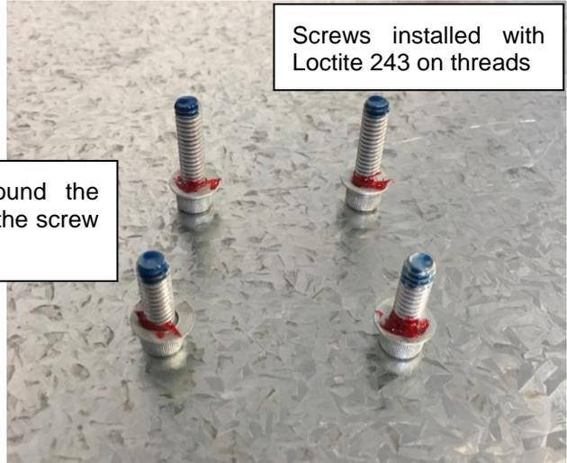
Screws installed with Loctite 243 on threads
