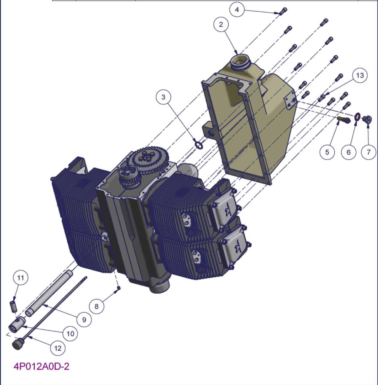
Figure 120 – 2200 Sump installation (integral plenum) – Parts List
