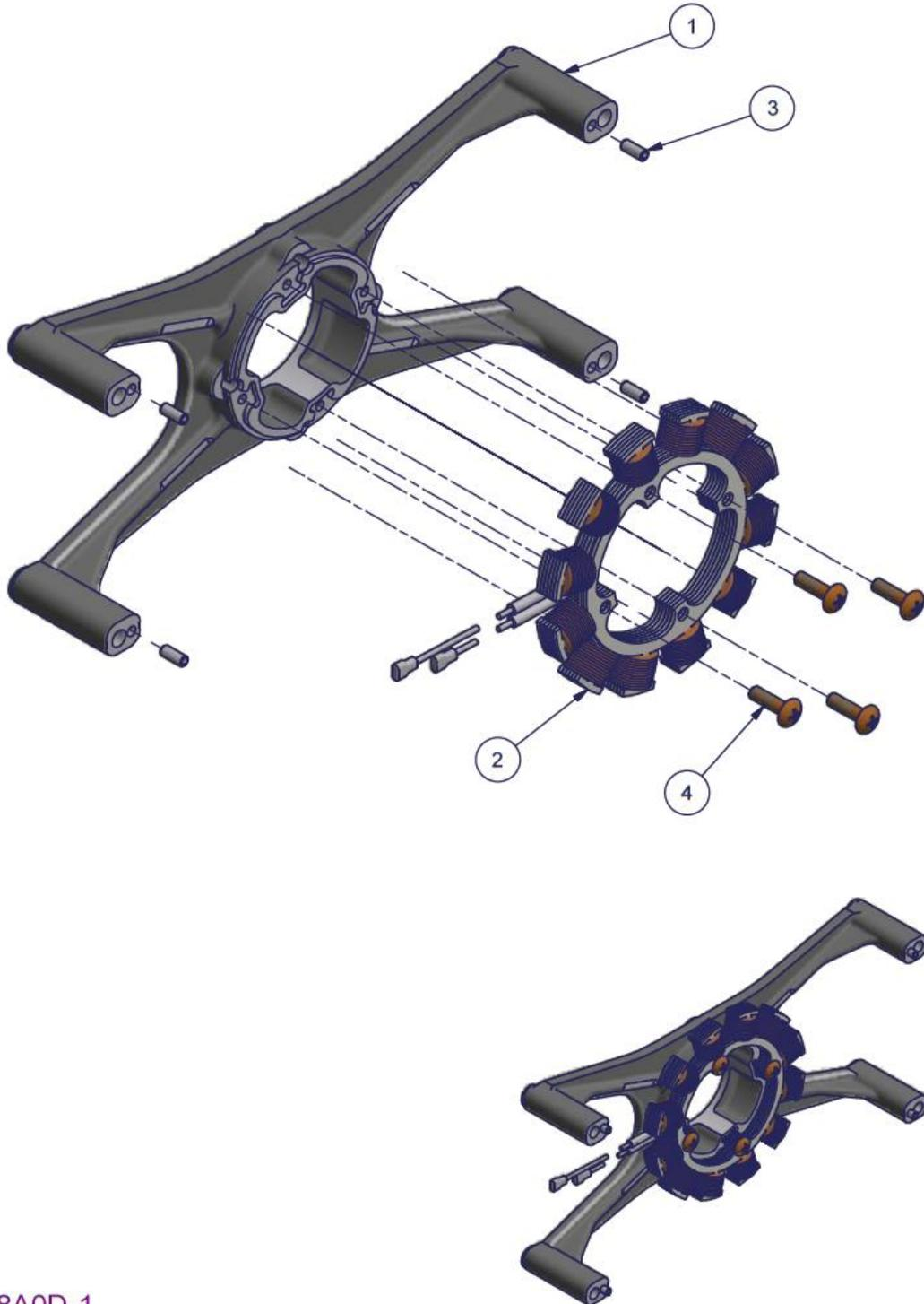
Figure 98 – 2200/3300 alternator stator subassembly – Parts list
