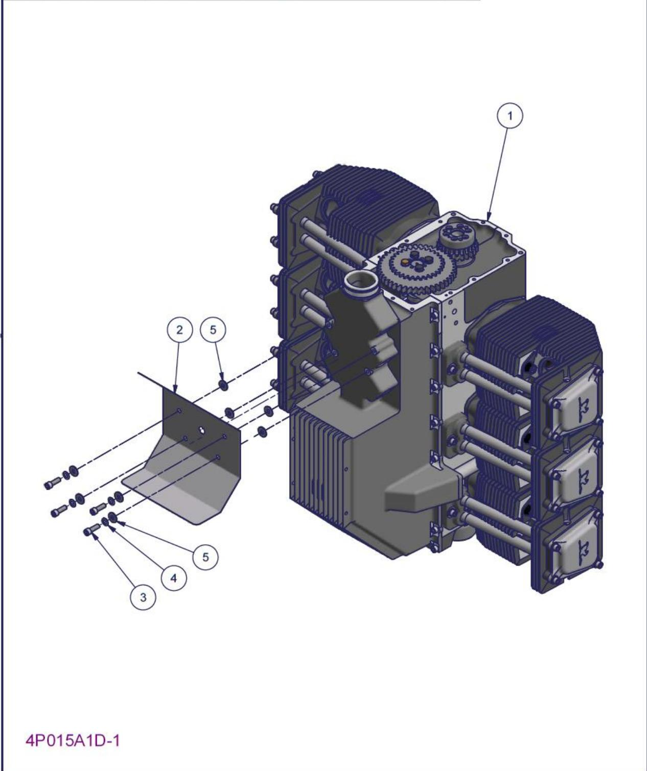
Figure 132 – 3300 Heat shield installation (integral plenum) – Parts List
