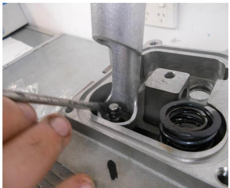
Figure 57 - Installing valve gear into the cylinder heads
