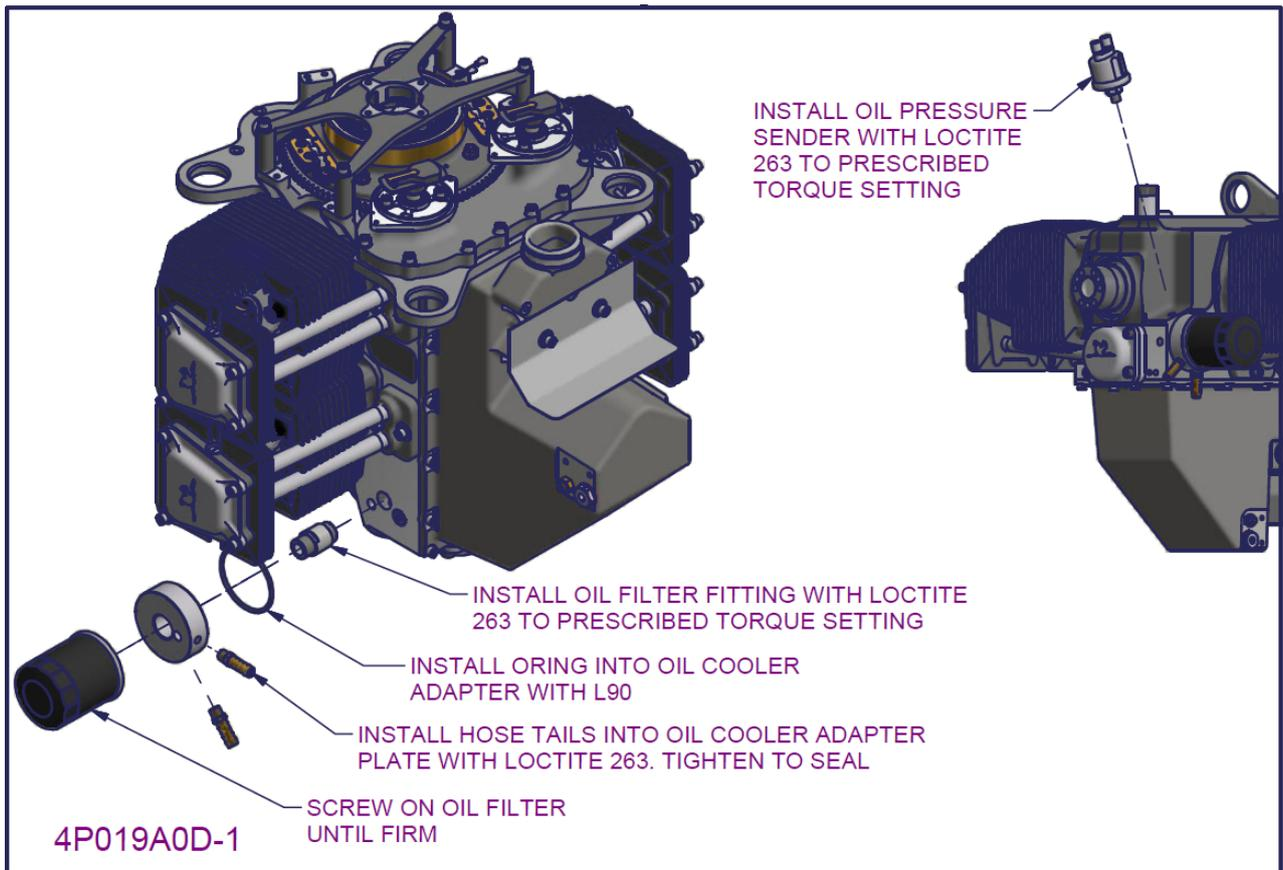
Figure 161 – 2200/3300 Oil pump and filter installation 3
