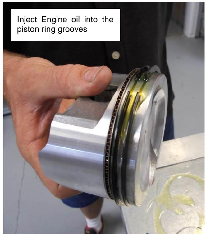
Figure 64 - Piston ring installation and oiling
