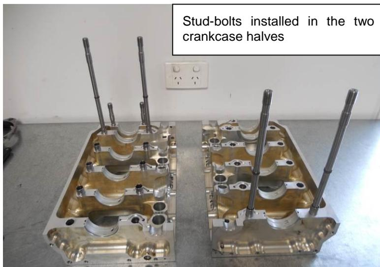
Figure 21 - Stud-bolts installed in the two crankcase halves
