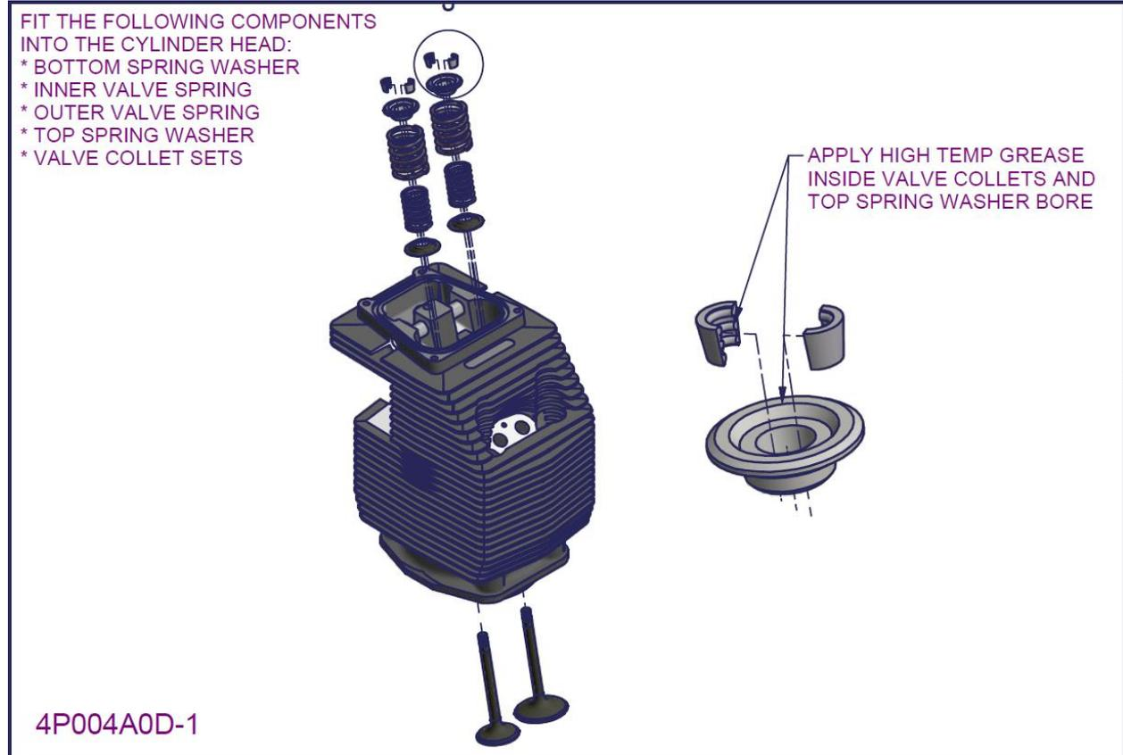
Figure 56 – 2200/3300 cylinder assembly 4
