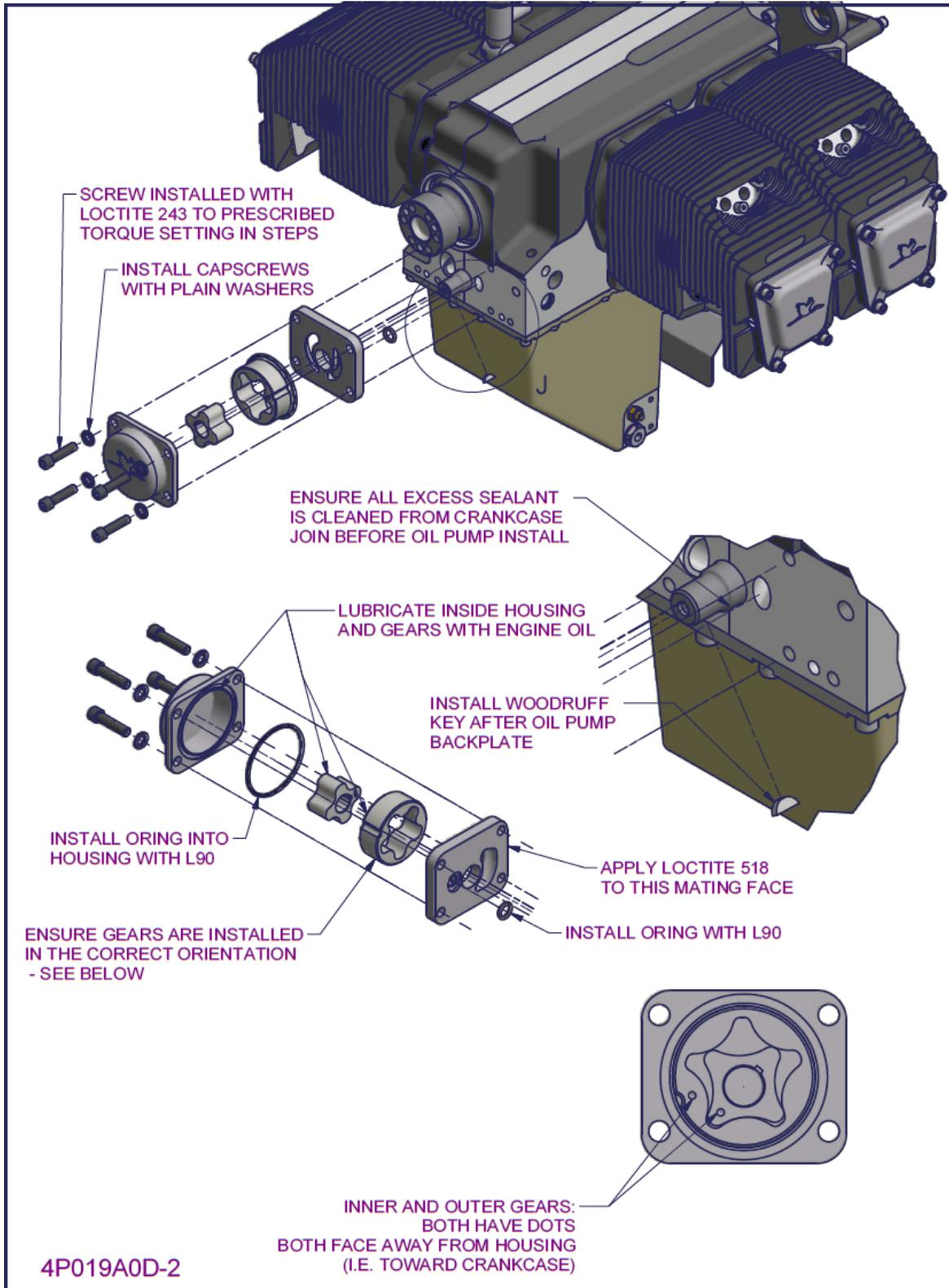
Figure 158 –2200/3300 Oil pump and filter installation 1
