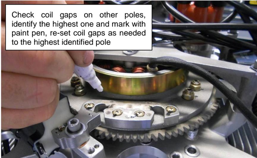
Figure 176 - Setting ignition coil gaps
