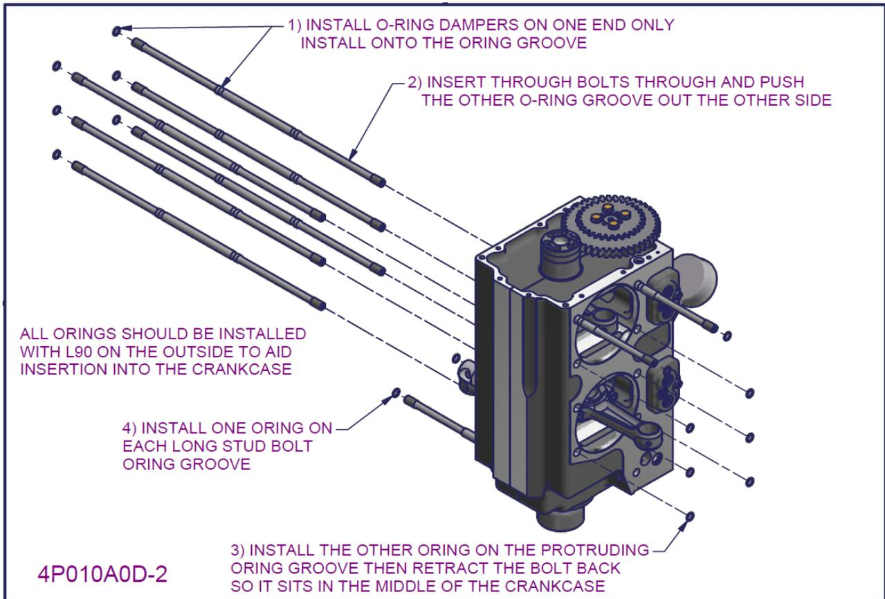
Figure 105 - 2200/3300 Joint engine assembly 2
