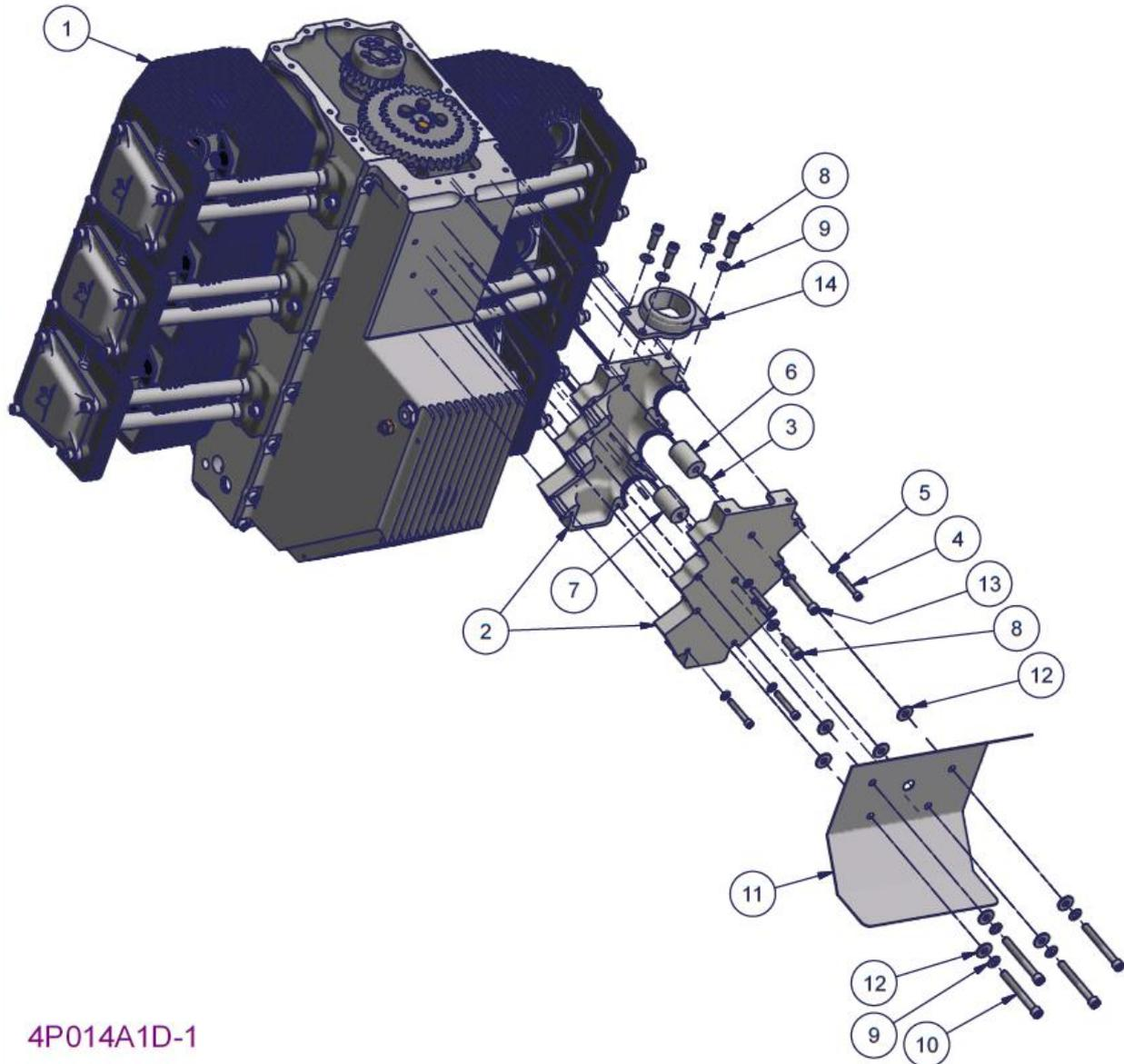
Figure 133 – 3300 Plenum and heat shield installation – Parts List
