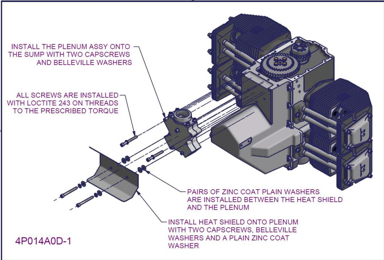
Figure 135- 2200/3300 Plenum and Heat shield installation 1
