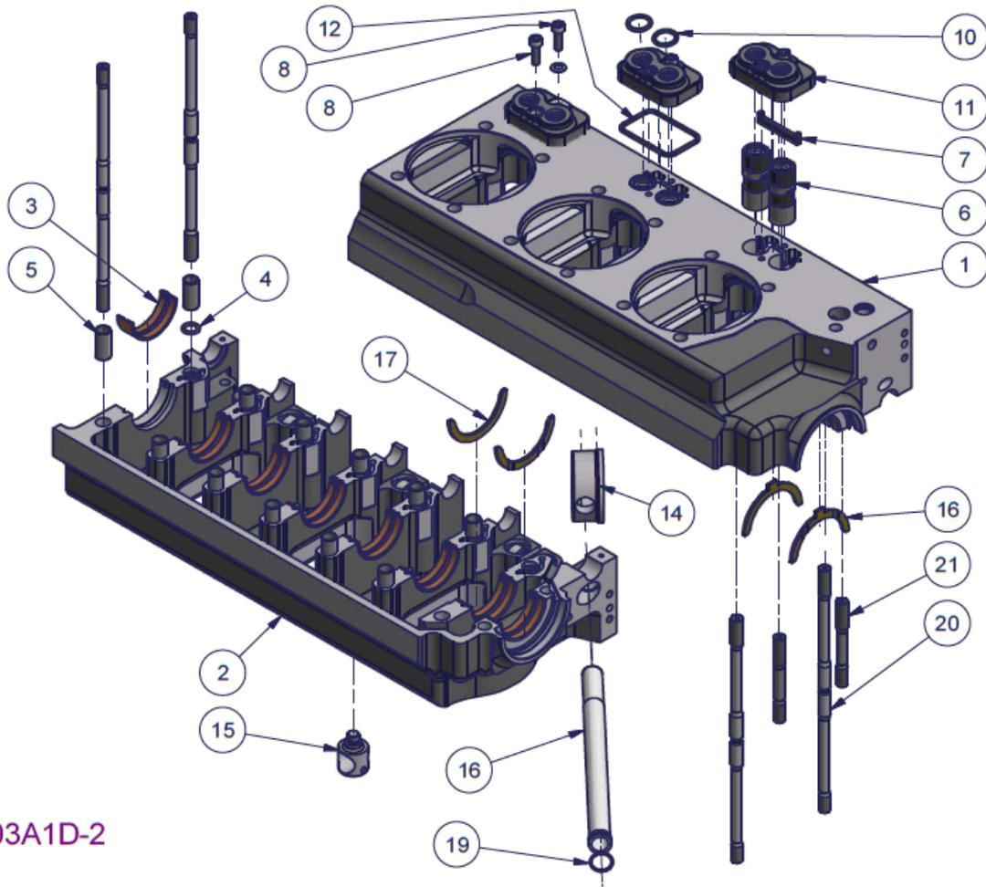
Figure 9 - 3300 Crankcase subassembly parts list
