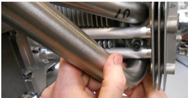
Figure 169 - position exhaust and upper induction pipes with clamp turtles
