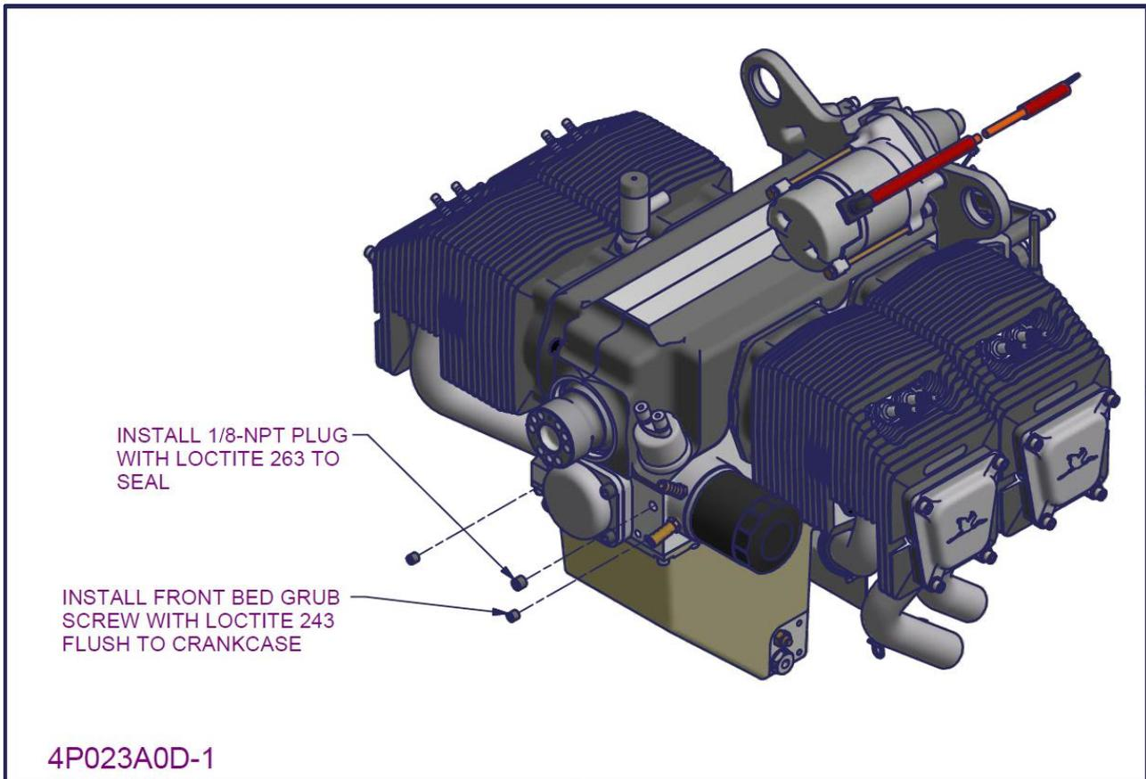
Figure 188 – 2200/3300 Front seal and propeller flange installation 1
