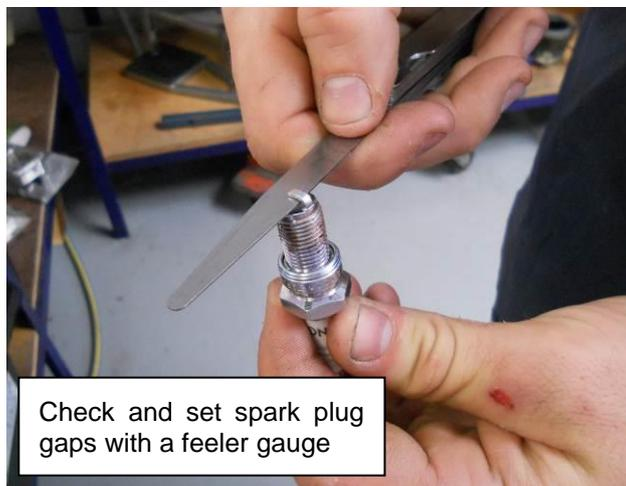
Figure 178 - Checking and setting spark plug gaps
