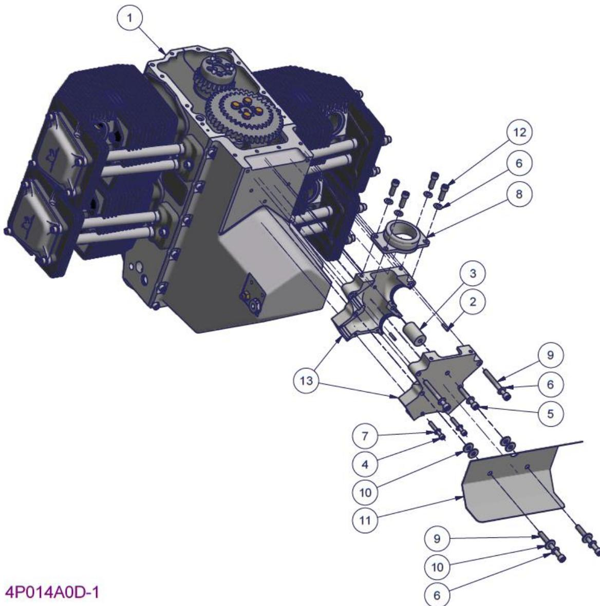
Figure 131 – Plenum and Heat shield installation – Parts List
