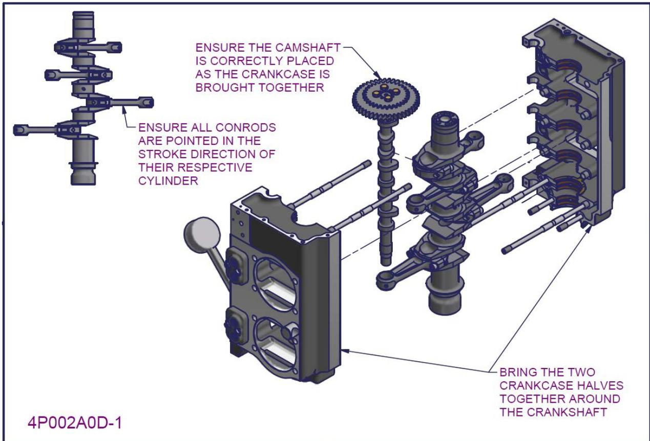
Figure 103 - 2200/3300 Joint engine assembly 1
