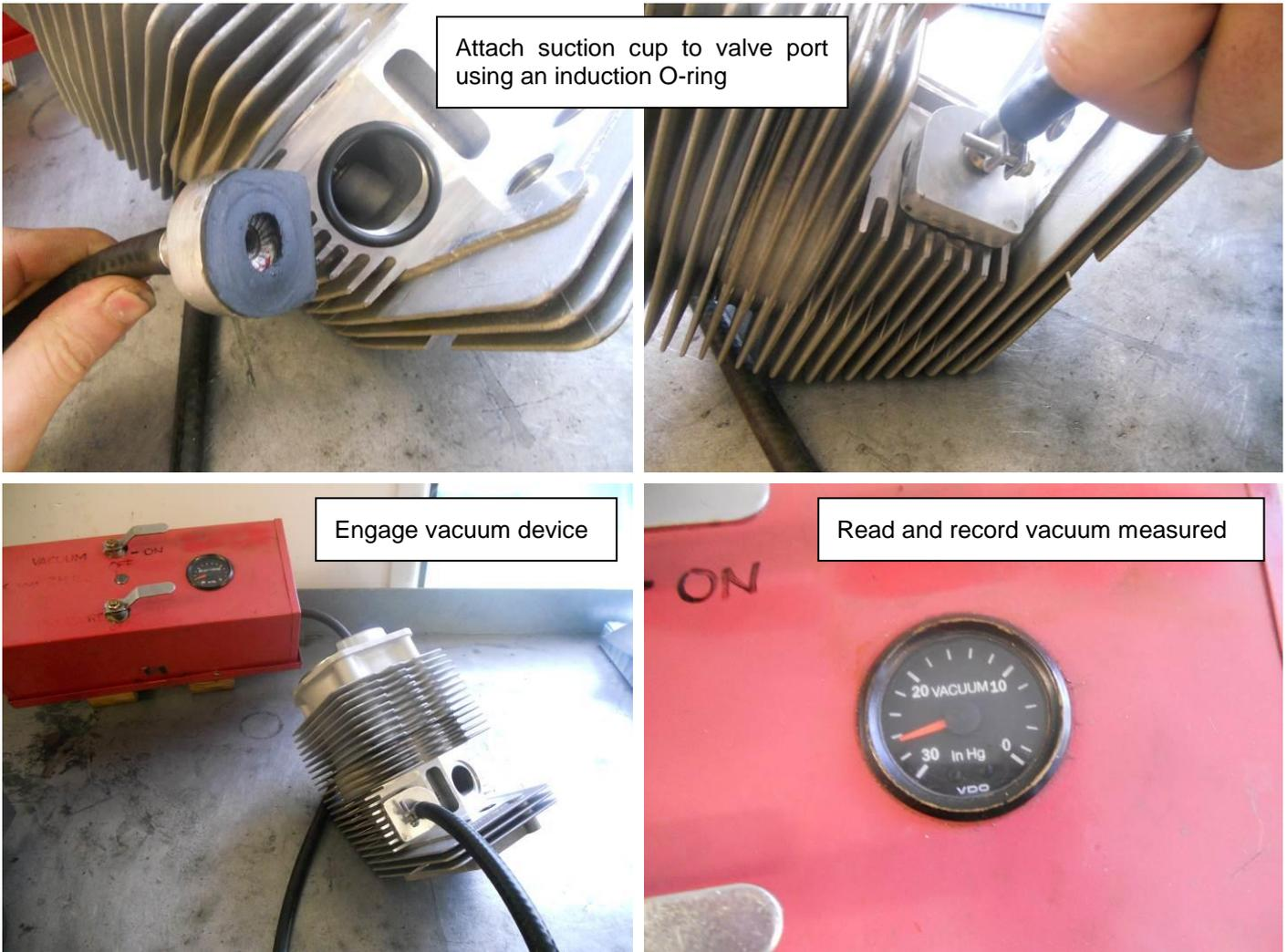
Figure 52 - Using a vacuum check to assess the valve sealing quality
