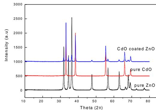
**Fig. 1** XRD spectrum of the pure ZnO, CdO and CdO-ZnO composite
