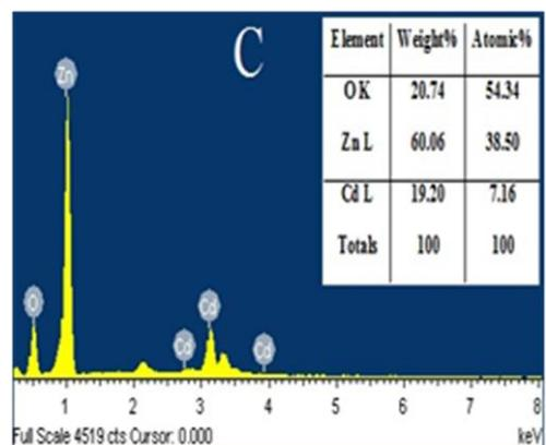
**Fig. 3** EDX analysis of pure ZnO pure CdO and CdO-ZnO composite nanoparticles
