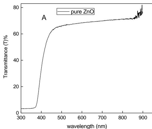
**Fig. 5** A, B, C Transmittance spectra of pure ZnO, CdO and CdO-ZnO composite film
