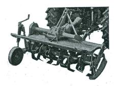
The Series I 'E' Type Rotavator ran to Serial No. 11628 and in 1958 the Series II machine commenced (Serial No. 11629). In this series the famous Selectatilth gearbox was introduced as an alternative to the single speed gearbox.
