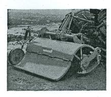
In 1954 the 'E' Mounted Rotavator appeared. This was the first Universal Mounted Machine capable of attachment to most farm tractors with 3-point linkage, and thereby superseded many special and 'F' type Rotavators which were built for individual tractor 5 mgle dreed stransmin KA. DJ models.
