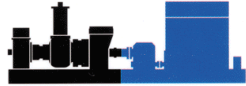
3. Turbine - generator module
