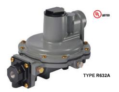
Type R632A has 1/8-inch NPT built-in gauge taps, orificed to a No. 54 drill size, on the upstream and downstream sides. These taps provide easy access for testing the proper operation of the First and Second-Stage while the system is pressurized. This regulator also features a large 3/4-inch drip-lip vent to reduce the chance of blockage by freezing rain or sleet when properly installed with the vent pointing down.
