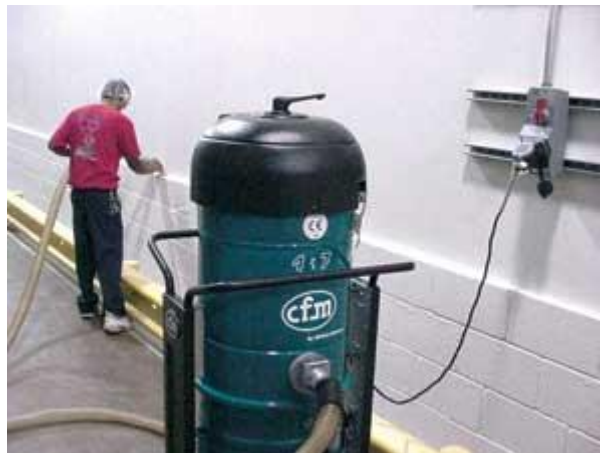
Figure 2. Riviana Foods uses a HEPA-filtered portable vacuum for cleaning the rice-drying side of its processing facility. Photo courtesy of Riviana Foods.
