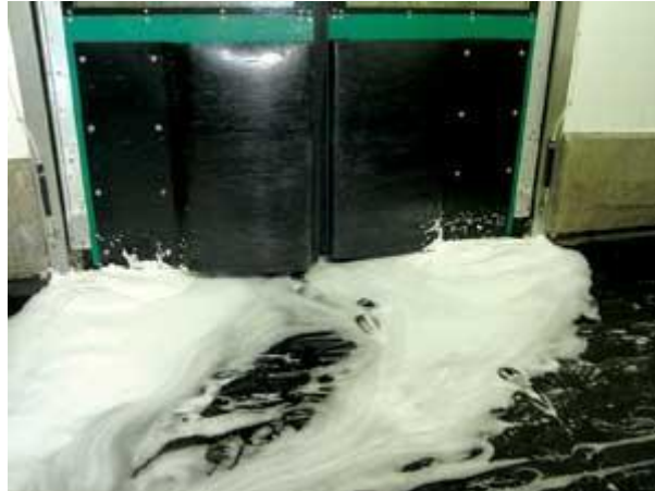
Figure 3. To prevent listeria from being transported from one room to the next, a quaternary ammonia door foamer, at 800 parts per million (ppm), is sprayed in every doorway linked to the assembly area. Photo courtesy of Overhill Farms.
