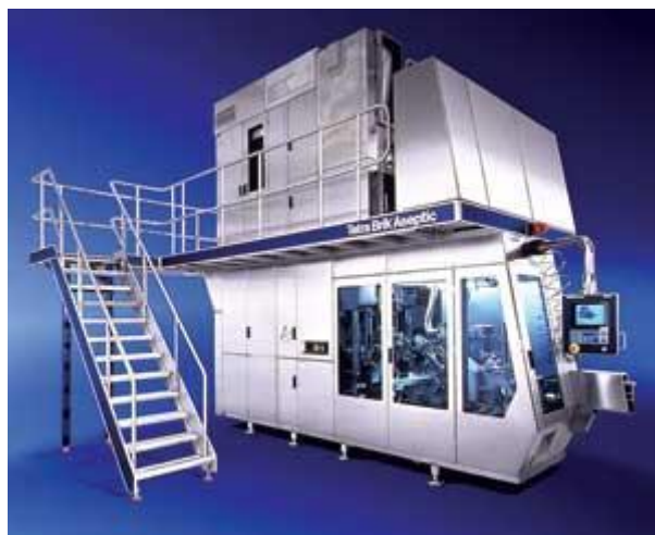
Figure 1. The Tetra Brik Aseptic TBA/21 filling machine is one example of a closed-loop aseptic processing system, which keeps product batches isolated to prevent contamination. Photo courtesy of Tetra Pak.
