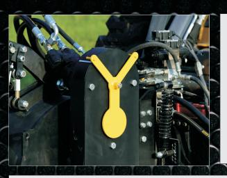
A level gauge built into the belt guard cover keeps the grinder housing parallel to the road surface ensuring proper function of the glide wheel system.
