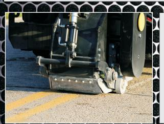
The **TRANSFORMER GRINDER** uses five urethane rubber seals to help control dust and debris.
