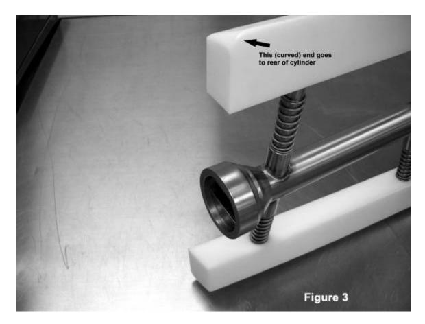
The drive shaft in the back of the machine must be lubricated daily with Vaseline, Lubri-Film or Petro Jel. Put a generous amount around the round part of the drive shaft. When you install the drive shaft in the back of the machine the excess Vaseline will be pushed forward into the cylinder which you can then wipe off.
