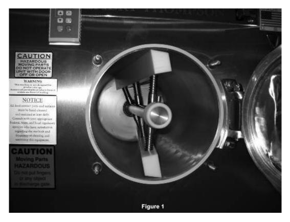
It is important that the scraper blades be installed properly – see figures 2 and 3. When installing the blades on the dasher, the curved end of the blade goes to the back of the machine. Note: if your machine is three phase power, check that the rotation is *counter-clockwise*.
