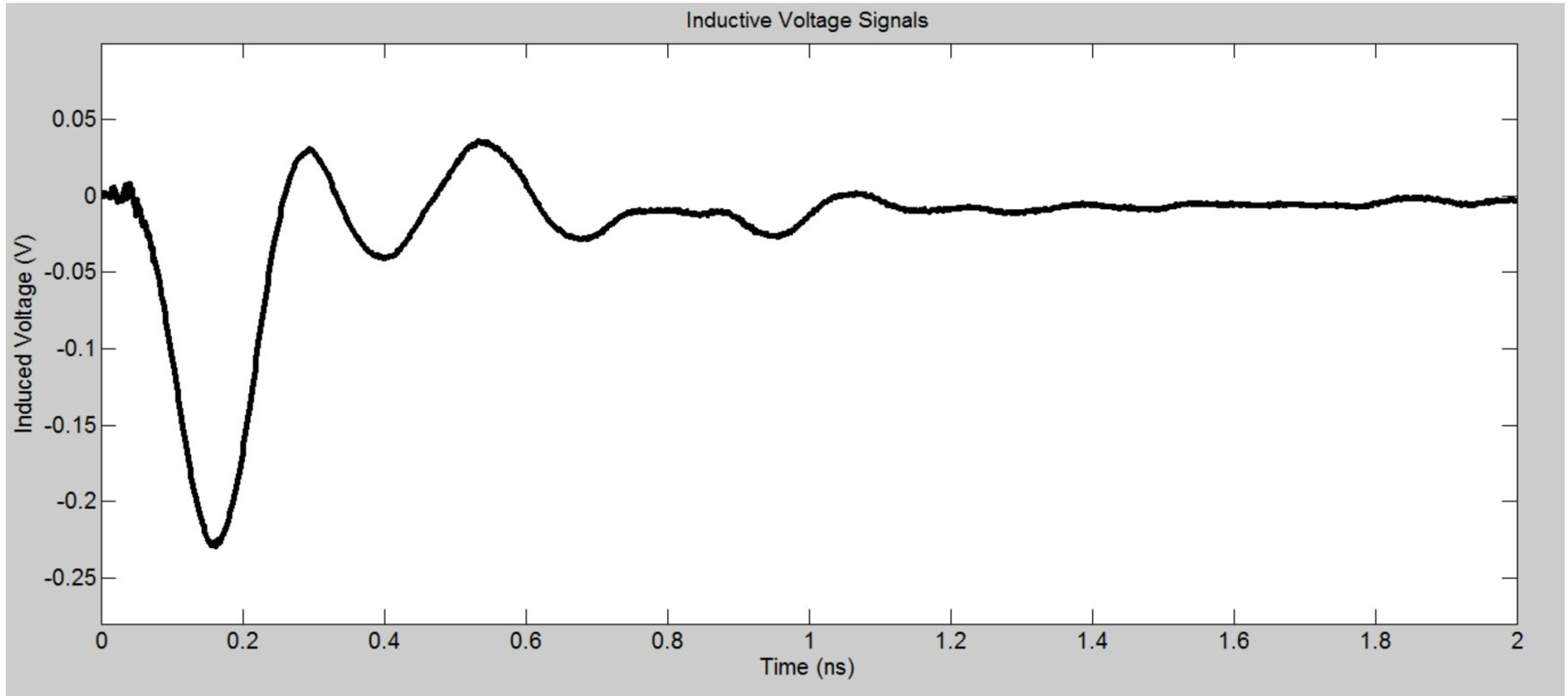
Example of a typical corrected measurement. Note the measured voltage signal is still not exactly a damped sine wave as predicted. Why?
