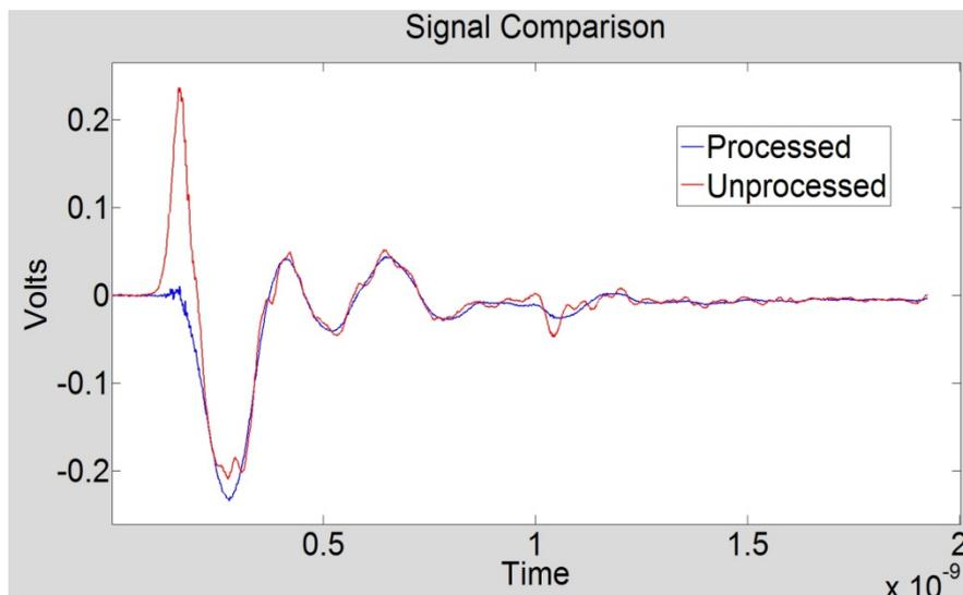
This introduces relatively large voltage spikes and an apparently noisy signal (red). Signals must be time shifted to correlate them between 0V and -2.5V. This yields the actual signal (blue).
