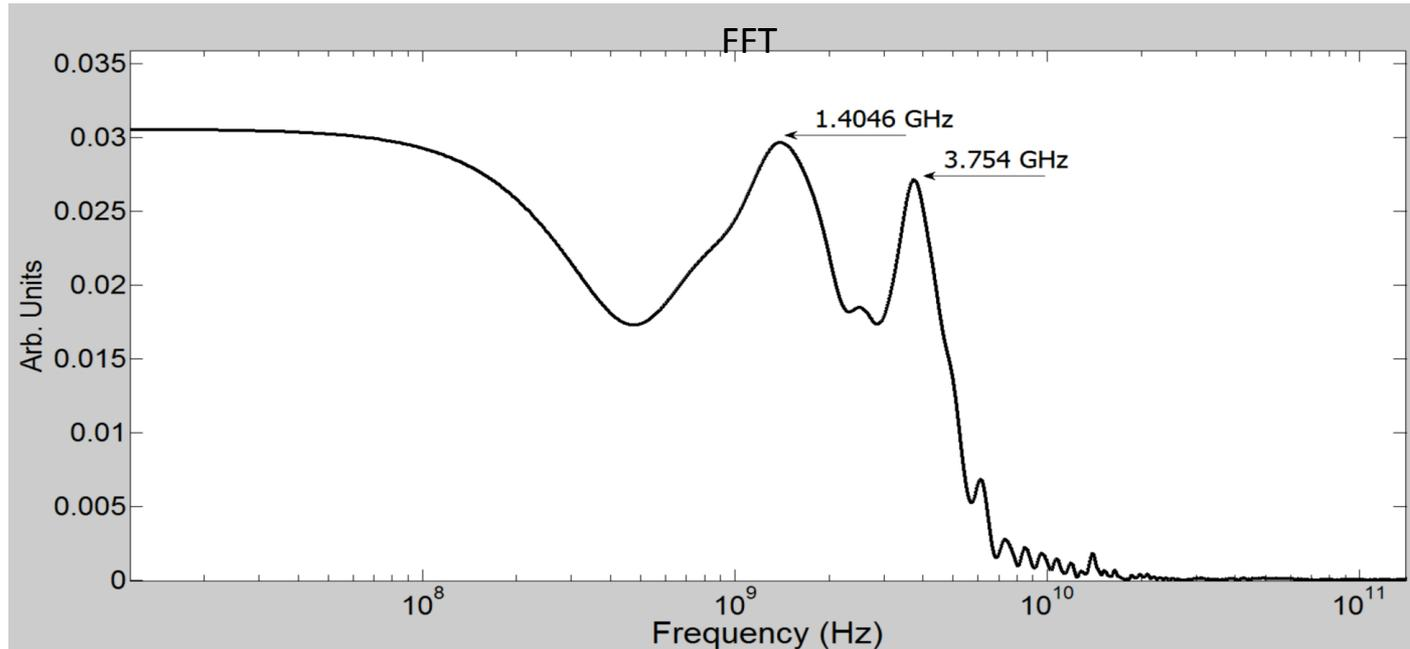
Two main resonance peaks are seen when an FFT is done on time-domain results. They must both be accounted for in a time domain data fit. The low frequency mode is the known resonant frequency of magnetite from FMR experiments. The definite origin of the higher mode is presently unknown.
