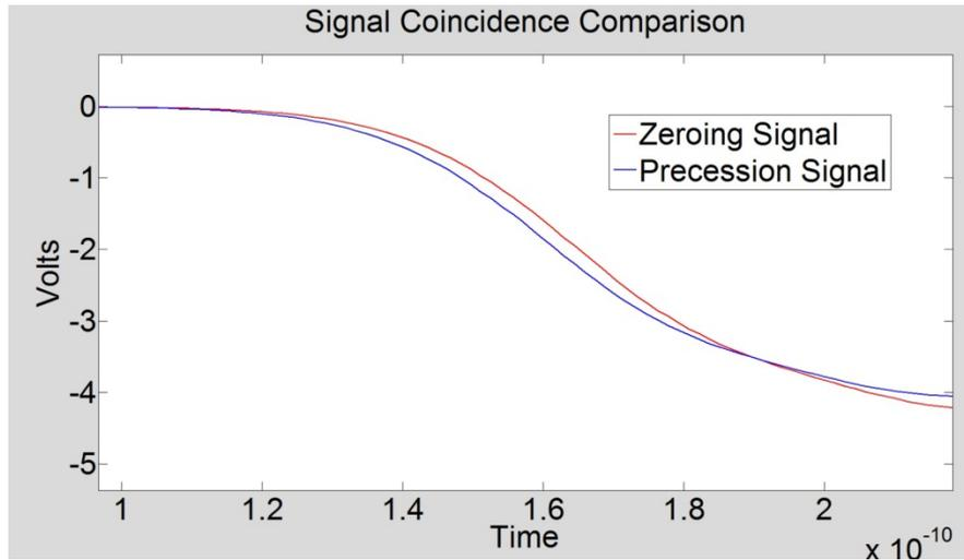
“Zeroing” step signal is not aligned in time with “Precession” step signal due to a *slight* drift in trigger signal.
