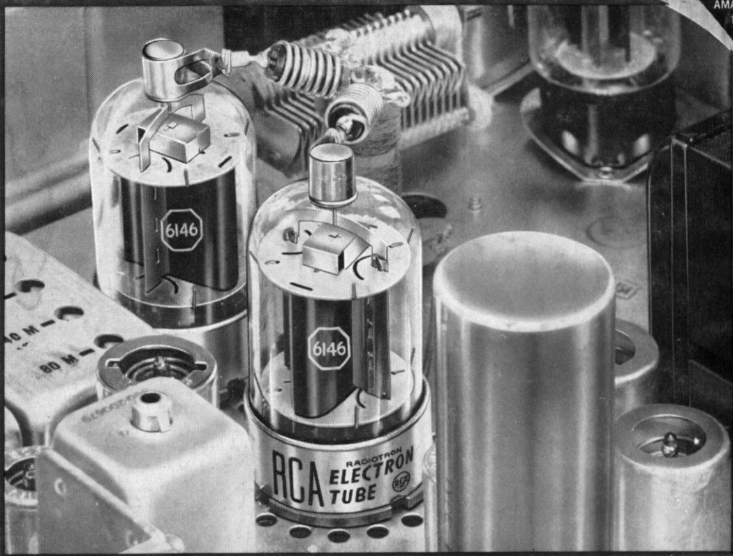
Inside view of the HT-37, showing the two RCA-6146's in parallel in the linear final.
