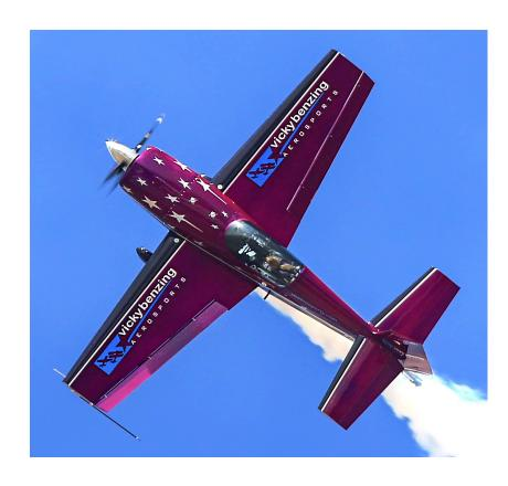
Vicky's beautiful monoplane was designed and built by Extra Aircraft for use in world level aerobatic competition. It is capable of +/- 10 G maneuvers with roll rates in excess of 400 degrees per second and has a top speed of 250 mph.
